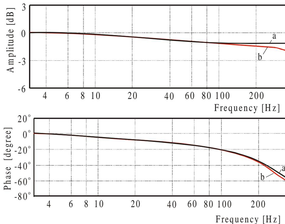
Figure 8- Amplitude and phase response of the magnetic actuators force for two different input currents:  $i(t) = i_s \sin(\omega t)$ ; a)  $i_s = 1,5$  A, b)  $i_s = 3$  A.
