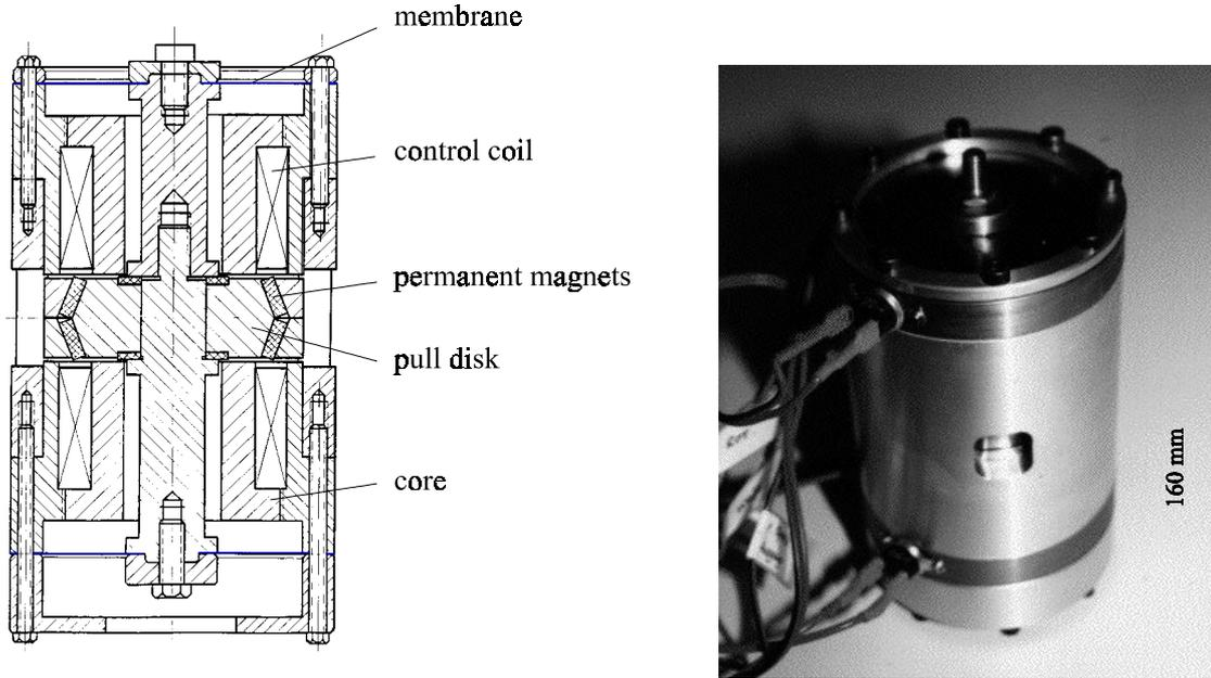
Figure 4- Sketch and prototype of the magnetic actuator.
