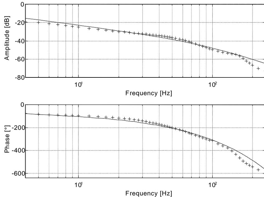
Figure 2- Transfer characteristics of the regulating distance: simulation (—); measurement (+++).
