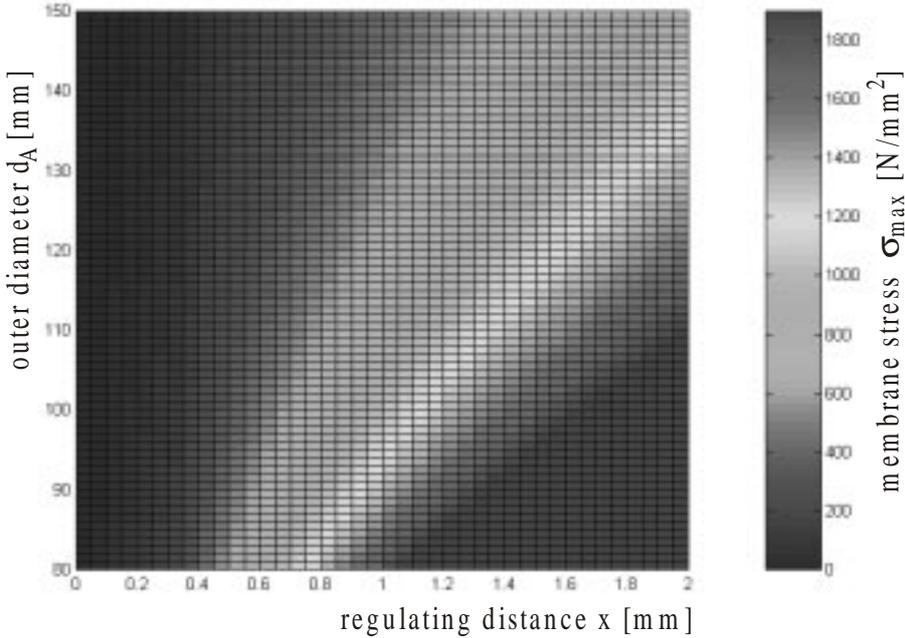
Figure 6- Maximum membrane stress as a function of the outer diameter  $d_A$  and the control distance  $x$ .
