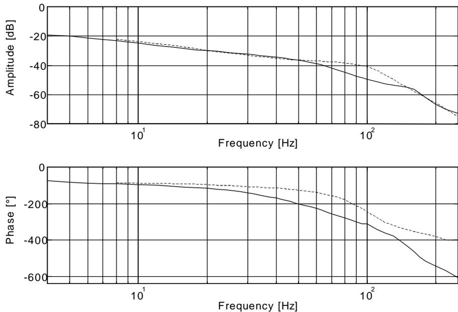
Figure 3- Measured transfer characteristic of the regulating distance for various length of the oil pipes: 2 m (—), 0.5 (---).
