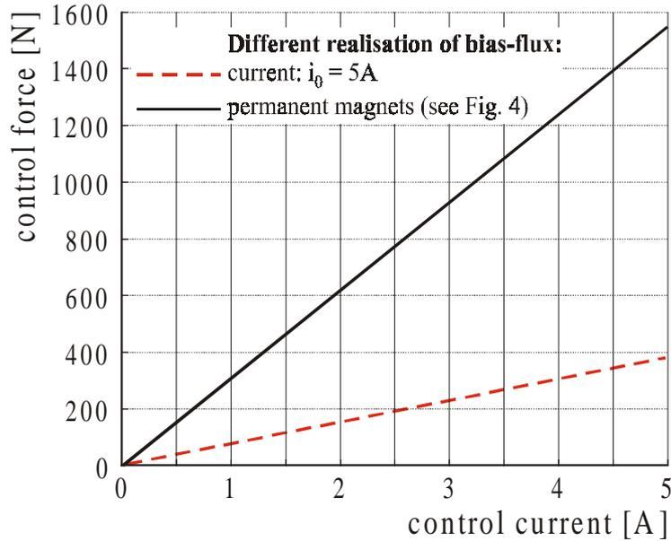
Figure 5- Measured force-current diagram for various magnetic actuators in the reference position  $x = 0$ .
