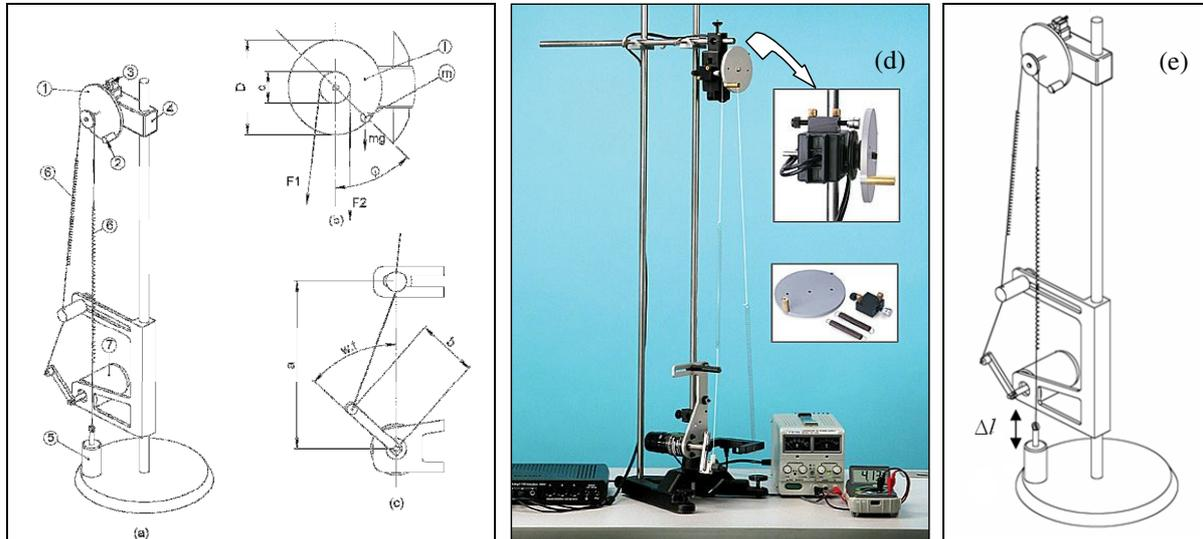
Figure 1. Nonlinear pendulum. (a) Physical Model. (1) Metallic disc; (2) Lumped mass; (3) Magnetic damping device; (4) Rotary Motion Sensor; (5) Actuator; (6) String-spring device; (7) Electric motor. (b) Parameters and forces on the metallic disc. (c) Parameters from driving device. (d) Experimental apparatus. (e) Actuator.
