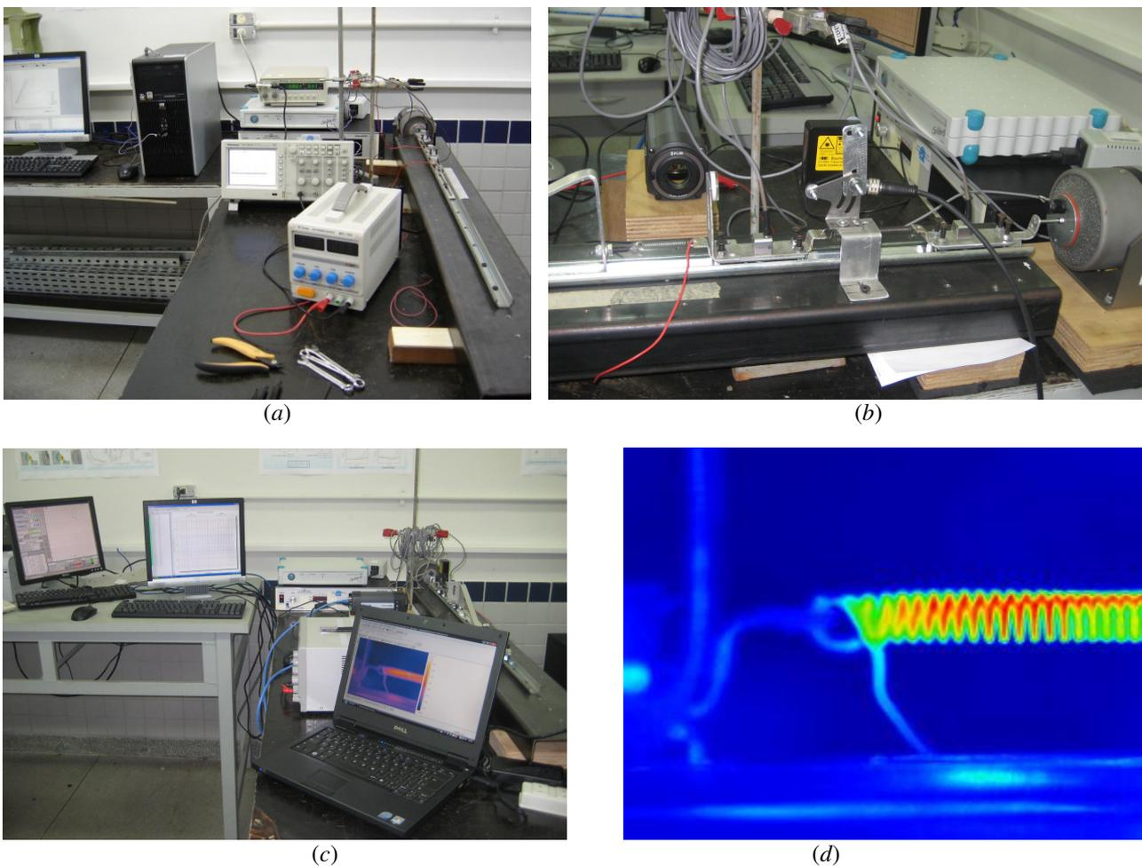
Figure 1. Experimental apparatus to study the dynamical behavior of linear oscillators at LACTM-CEFET/RJ (a-c). Infrared (IR) thermal image of the SMA spring subjected to a 1.2A electric current (d).
