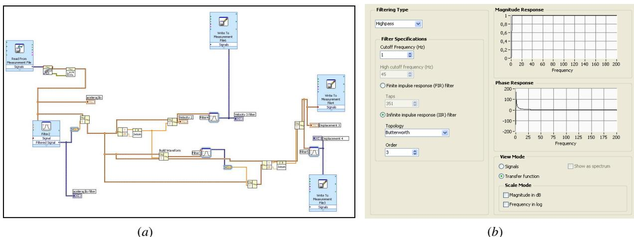
Figure 3. Double integration Labview procedure for accelerometer signal: (a) block diagram and (b) filter parameters and transfer function.
