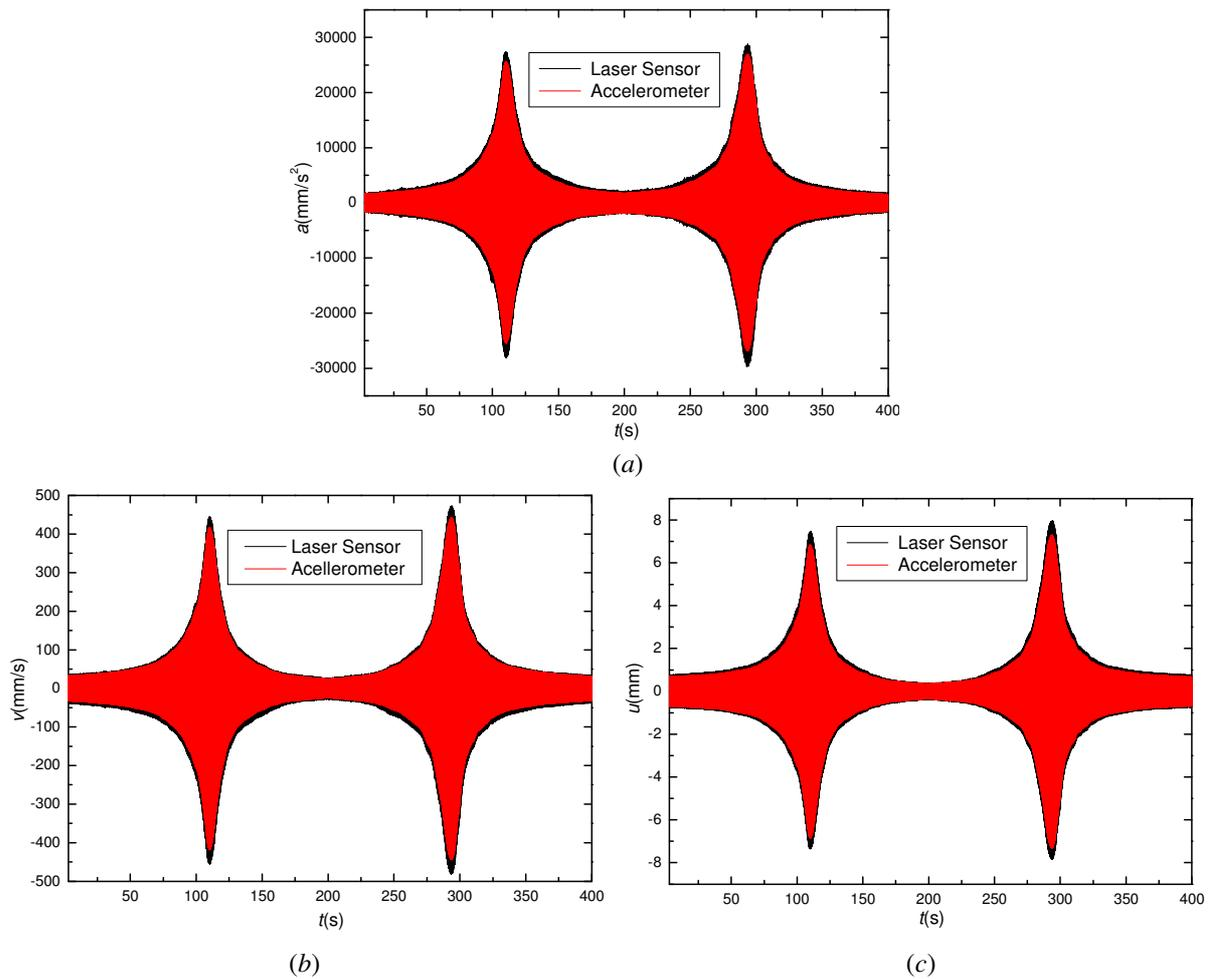
Figure 4. *Linear elastic oscillator*: acceleration (a), velocity (b) and displacement (c) time evolution considering two complete forward and backward sweep cycles (7.5Hz to 11.5Hz and 11.5Hz to 7.5 Hz).
