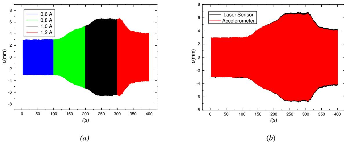
Figure 11. *SMA oscillator*: displacement evolution of car 2. Accelerometer (a) and comparison between accelerometer and laser signals (b) during heating (0.6 → 0.8 → 1.0 → 1.2 A) for 8.9 Hz.
