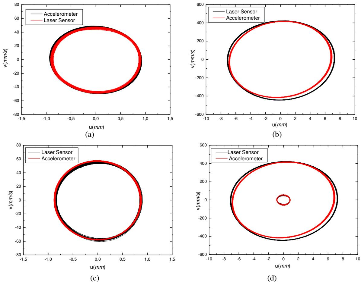
Figure 5. Linear elastic oscillator phase space: (a) 8.5Hz, (b) 9.6Hz, (c) 10.5Hz and (d) 8.5, 9.6 and 10.5Hz.
