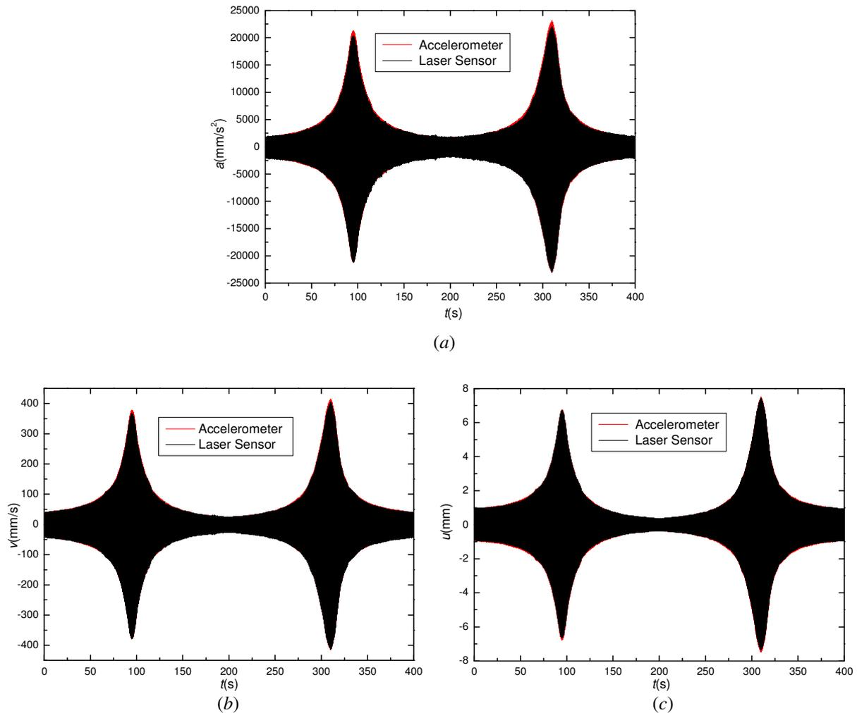
Figure 6. SMA oscillator: acceleration (a), velocity (b) and displacement (c) time evolution considering two complete forward and backward sweep cycles (7Hz to 11Hz and 11Hz to 7Hz).
