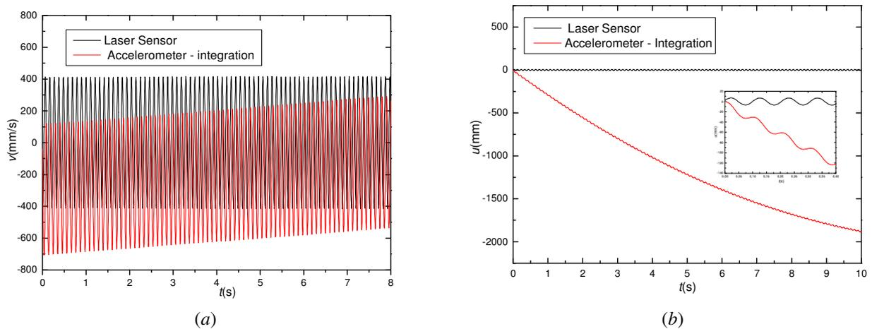
Figure 2. Direct numerical integration of a 9.6 Hz sinusoidal accelerometer. (a) velocity and (b) displacement.
