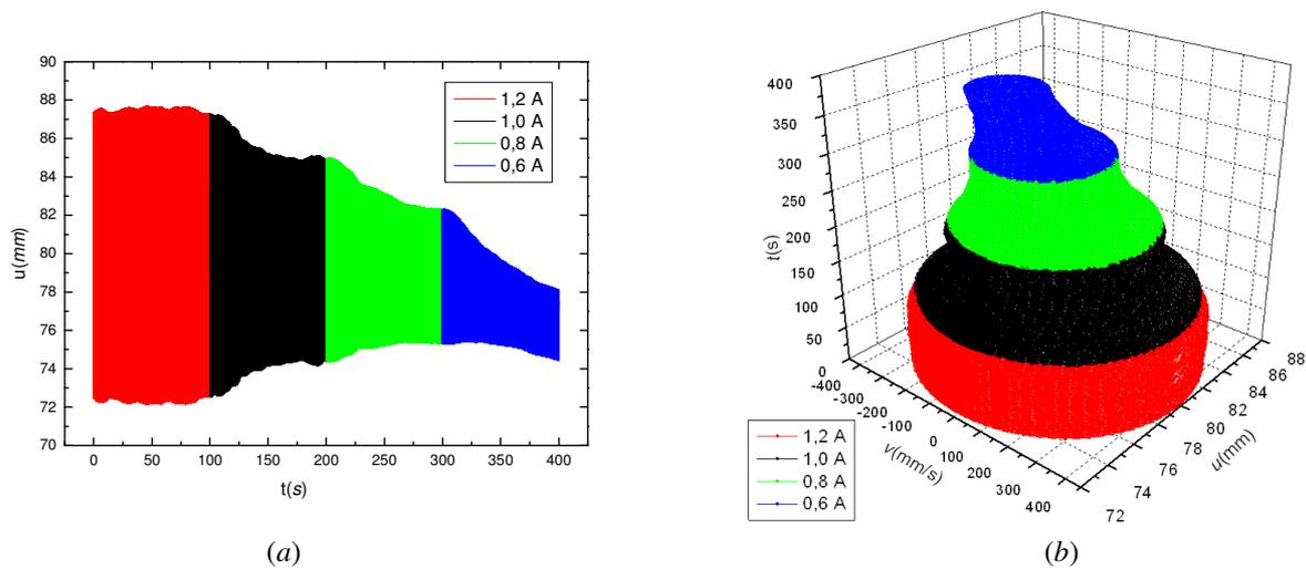
Figure 10. *SMA oscillator* dynamics from laser transducer signal: displacement evolution of car 2 (a) and phase space (b) during cooling (1.2 → 1.0 → 0.8 → 0.6A) for 9.2Hz..
