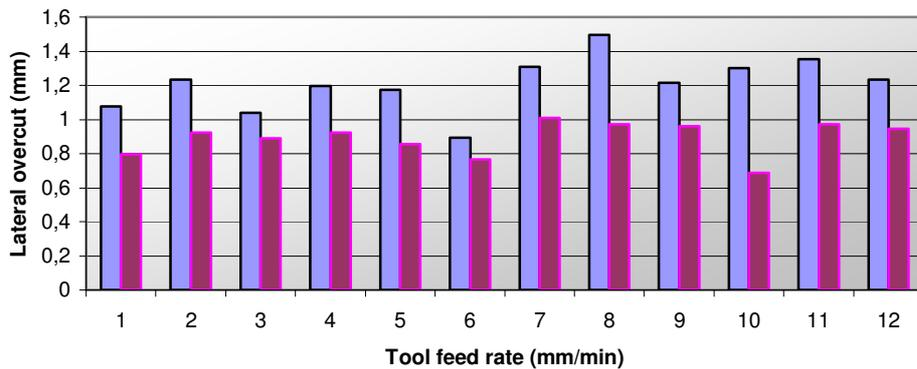
Figure 11. Comparative results of lateral overcut with  $\text{NaCl}$  and  $\text{NaNO}_3$ .
