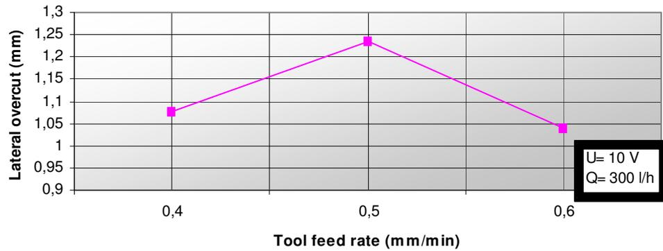
Figure 7. Lateral overcut with 300 L h<sup>-1</sup>, 10V and NaCl.
