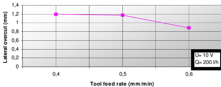
Figure 8. Lateral overcut with 200 L h<sup>-1</sup>, 10V and NaCl.
