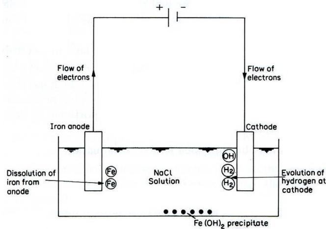
Figure 1. Electrolytic dissolution of iron, McGeough (1988).
