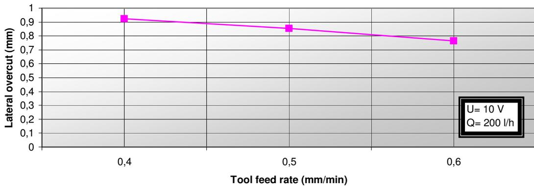
Figure 10. Lateral overcut with electrolyte flow of  $200 \text{ L h}^{-1}$ ,  $10\text{V}$  and  $\text{NaNO}_3$ .
