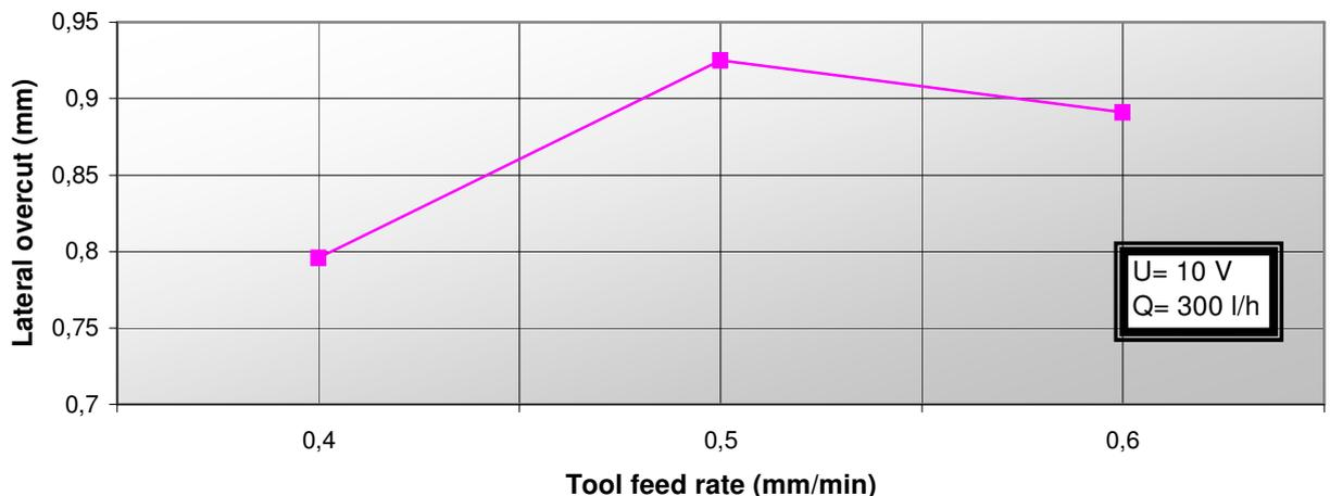
Figure 9. Lateral overcut with electrolyte flow of 300L h<sup>-1</sup>, 10V and NaNO<sub>3</sub>.
