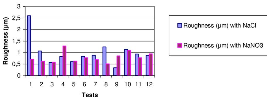
Figure 13. Comparative study of roughness between NaCl and NaNO<sub>3</sub>
