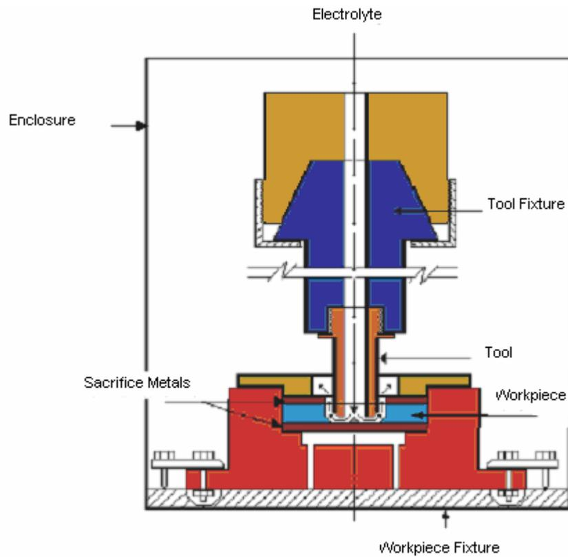
Figure 4. Schematic diagram of experimental set-up
