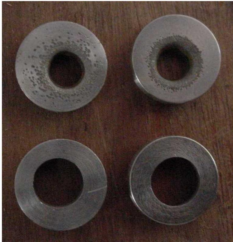
Figure 6. Workpieces machined without insulation plates (above) and with insulation plates (below).
