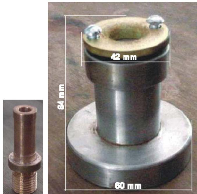
Figure (5). Electrochemical tool (without isolation, left) and support for securing workpiece (right), Silva Neto (2004).
