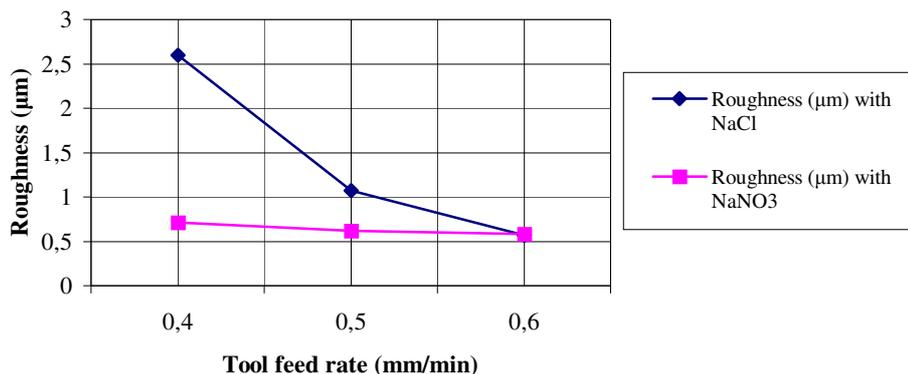
Figure 12. Roughness in function of tool feed rate.
