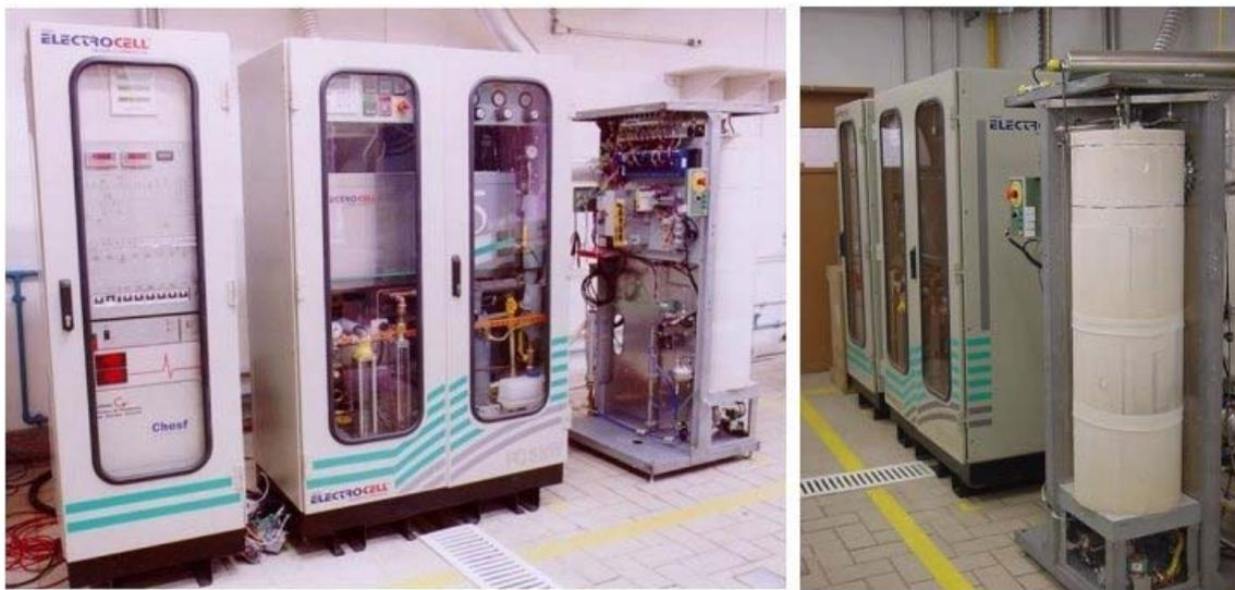
Figure 1. Different views of the Distributed generation 5kWe PEMFC-NG Reformer power cogeneration system.
