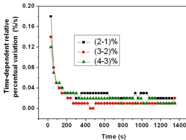
Figure 7. Results of electrochemical activation process tests of the 5kWe-PEMFC: relative percentual variations (in relation to the curves shown in Figure 6) in function of the tested operation time.
