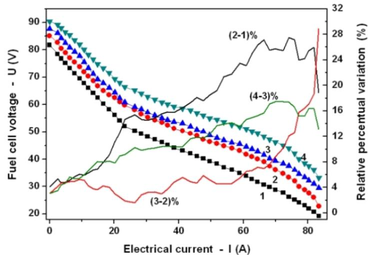
Figure 6. Results of electrochemical activation process tests of the 5kWe-PEMFC: four curves  $I \times U$  numbered (1 to 4) in increasing order of activation, and respective relative percentual variations between each pair of curves.
