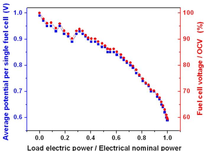
Figure 5. Curves of average potential per single fuel cell and the ratio between fuel cell voltage and OCV in function of the electric power used..
