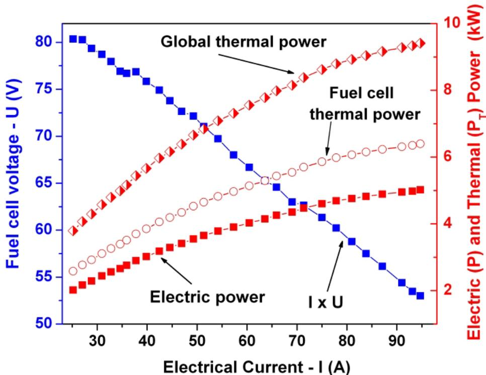
Figure 4. Characteristic curve  $I \times U$ , electric and thermal power versus electrical current in the typical region of operation (intermediate region of the Figure 3) of the analyzed 5kWe PEMFC-Natural gas reformer power cogeneration system.
