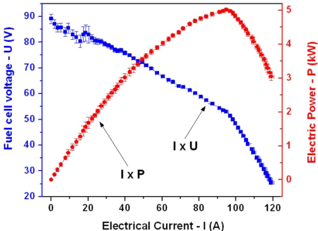
Figure 3. Performance curves ( $I \times U$  e  $I \times P$ ) of the 5kWe PEMFC-Natural gas reformer power cogeneration system.
