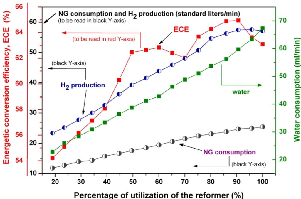
Figure 2. Characteristic curves of the NG reformer: flow rates of consumption of NG and deionized water, hydrogen production flow rate, and average energetic conversion efficiency (read in red y-axis) in function of the percentage of utilization of the reformer.
