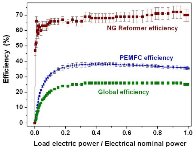
Figure 8. Relationships between efficiencies and electric power used.
