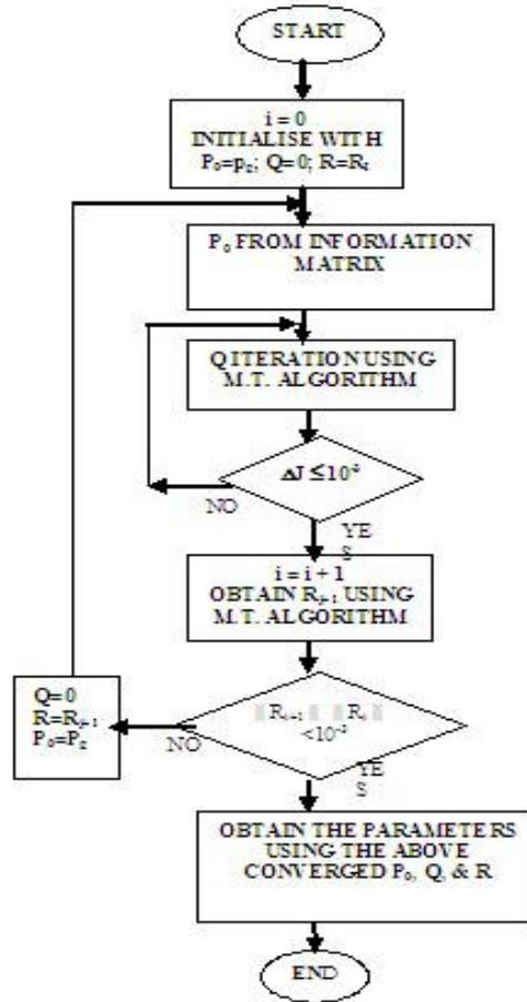
Fig-6 Schematic flow of Adaptive Estimation tuning process
