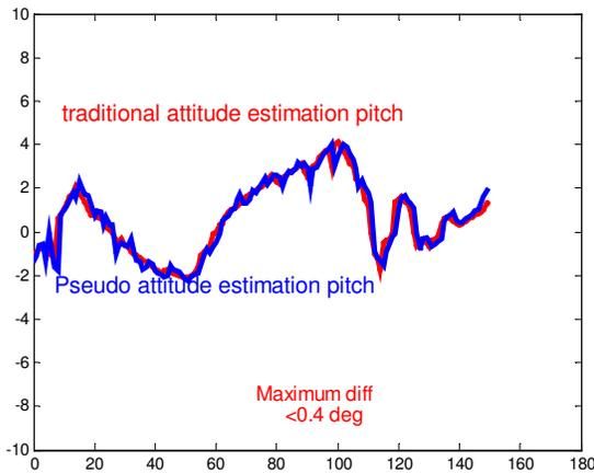
Fig-11B Comparison of "Pitch" angle Attitude estimation
