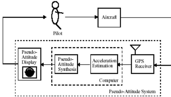
Fig – 5 Pseudo Attitude Display System and its components
