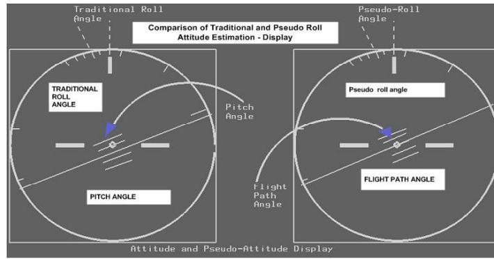
Fig-9 Snap shot of the Display: Comparison of Conventional and Pseudo Roll Attitude Estimation
