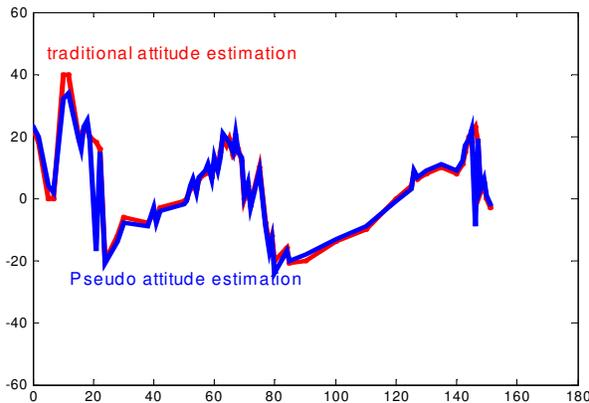
Fig-10 C Comparison of Traditional and Pseudo "Roll" Estimation
