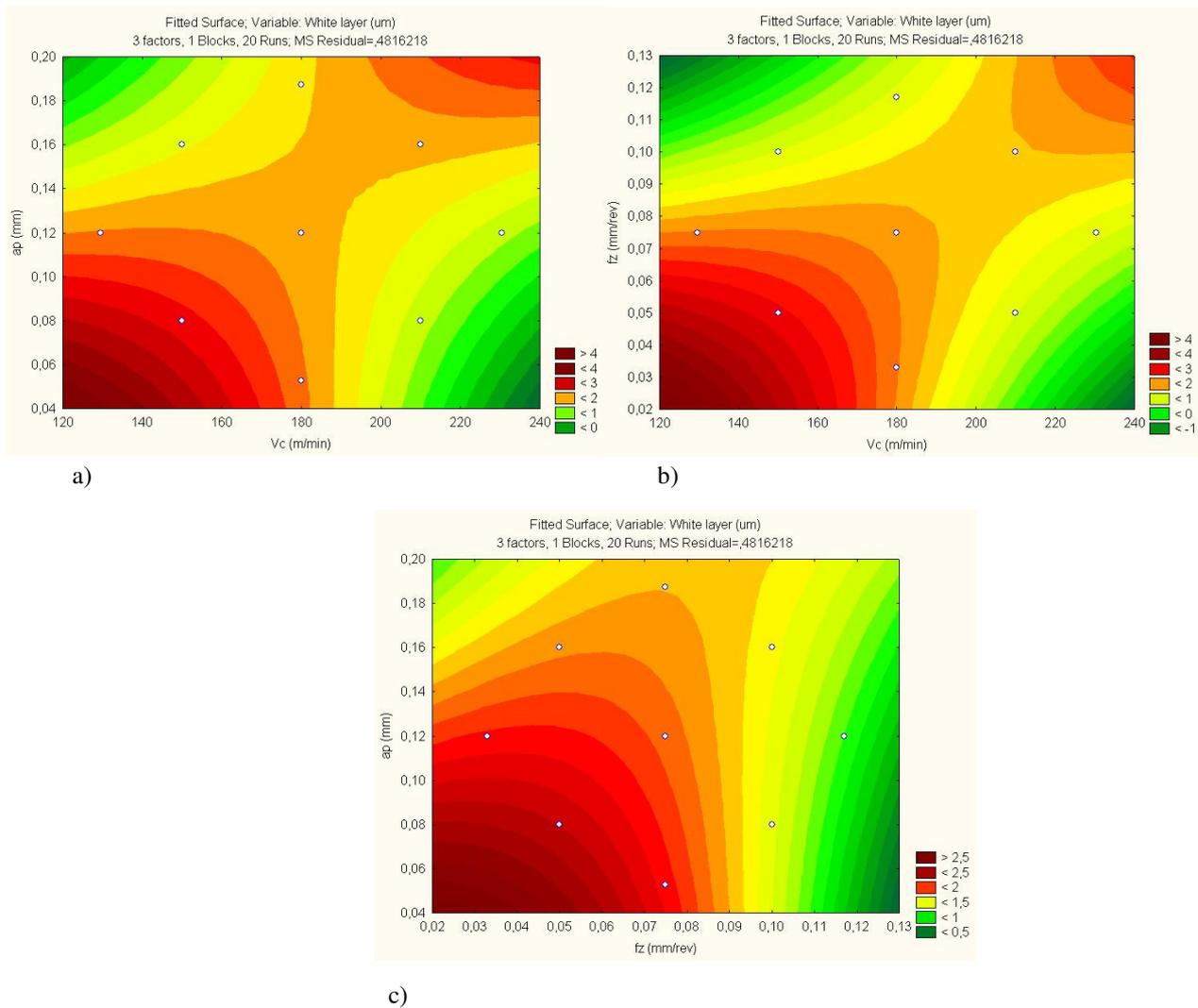
Figure 7. Graphs: a) “ $V_c \times a_p$ ”; b) “ $V_c \times f_z$ ”; c) “ $f_z \times a_p$ ” for the white layer thickness
