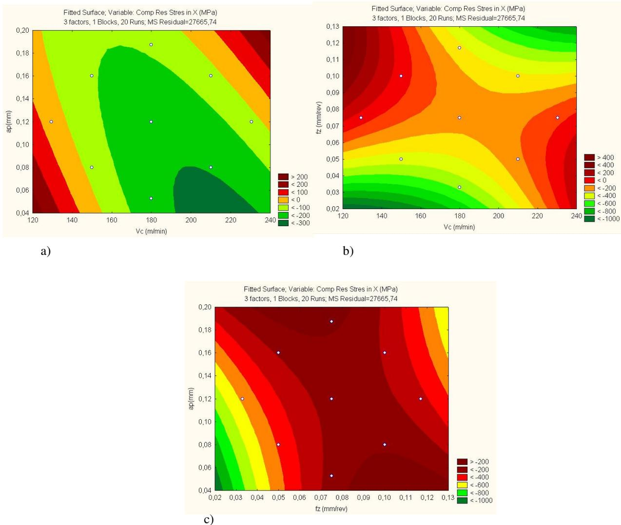
Figure 12. Graphs: a) “ $V_c$  x  $a_p$ ”; b) “ $V_c$  x  $f_z$ ”; c) “ $f_z$  x  $a_p$ ” for maximum residual stresses of compression
