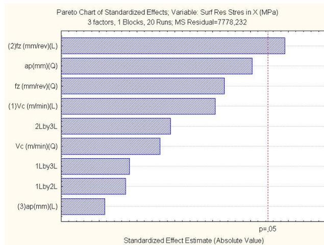
Figure 9. Pareto chart for the residual stresses on the surface
