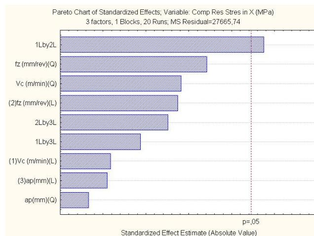
Figure 11. Pareto chart for the maximum residual stress of compression
