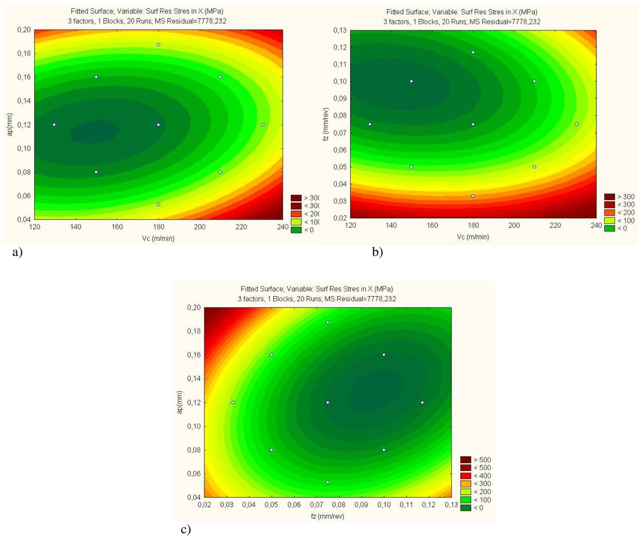
Figure 10. Graphs: a) "Vc x ap"; b) "Vc x fz"; c) "fz x ap" to surface residual stresses
