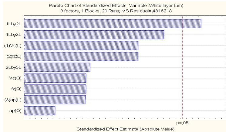
Figure 6. Pareto chart for the white layer thickness
