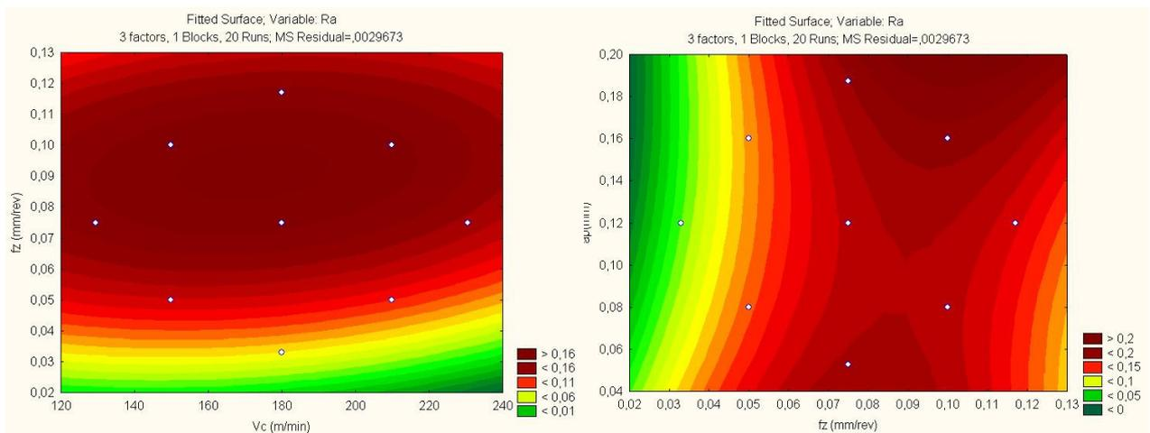
Figure 4. Graphs: “ $v_c \times f_z$ ” e “ $f_z \times a_p$ ” for roughness “Ra”
