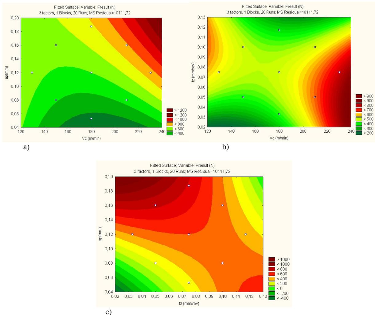
Figure 2. Graphs: a) “ $v_c \times a_p$ ”; b) “ $v_c \times f_z$ ”; c) “ $f_z \times a_p$ ” for the resultant force
