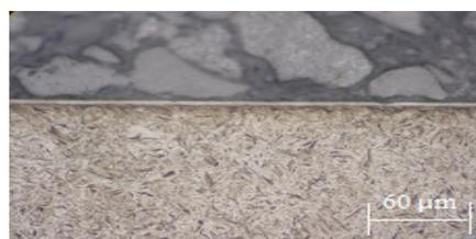
Figure 5 – White layer in a specimen
