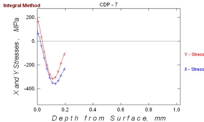
Figure 8. The typical behavior of the profile of the residual stresses measures in the body of test 7
