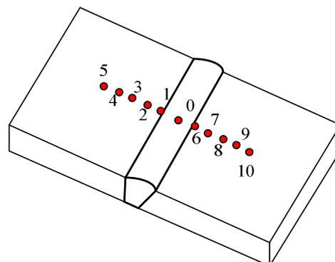
Figure 2.7 Point of measure in the aluminum alloy test specimens
