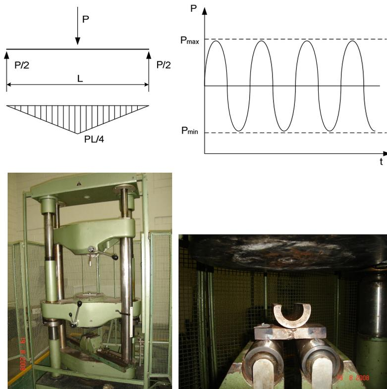
Figure 2.7 Three point bending test (Engineering School Laboratory, Mackenzie Presbyterian University)
