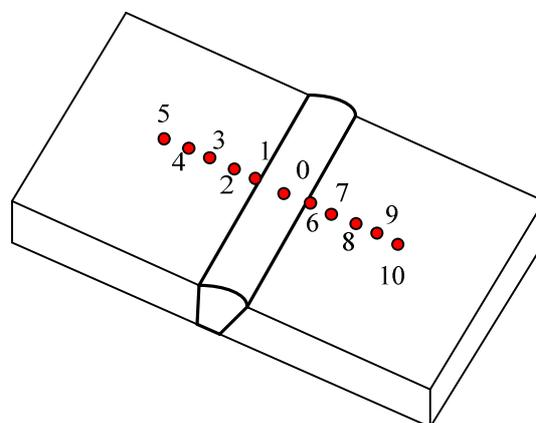
Figure 2.4 Points where the hardness (HB) was measured
