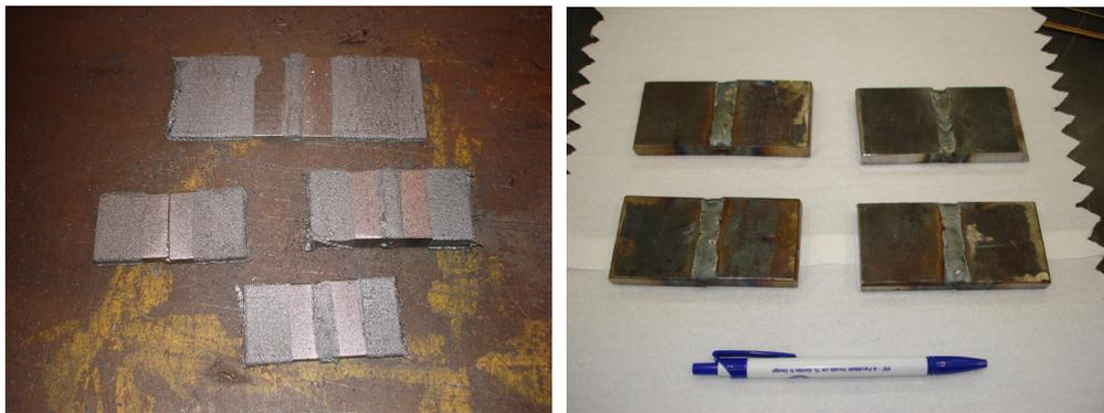
Figure 2.1 Test specimens with and without shot-peening
