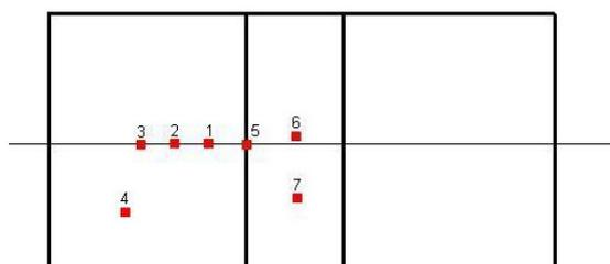
Figure 2.5 Points of measure in as-welded condition steel test specimen
