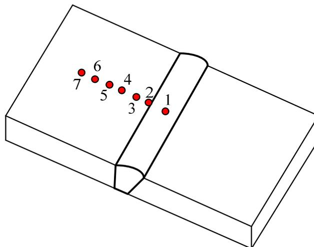
Figure 2.2 Points where the hardness (HRB) was measured
