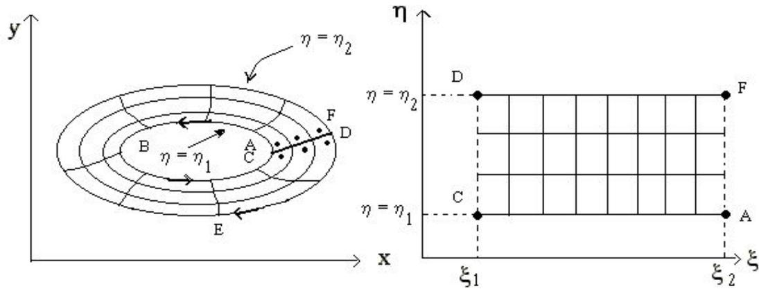
Figure 1. Double connected physical grid and the transformed computational domain.
