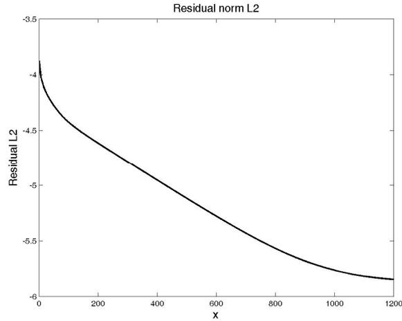
Figure 3. Residual history cylinder geometry
