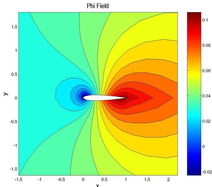
Figure 8. The potential for the airfoil NACA0012
