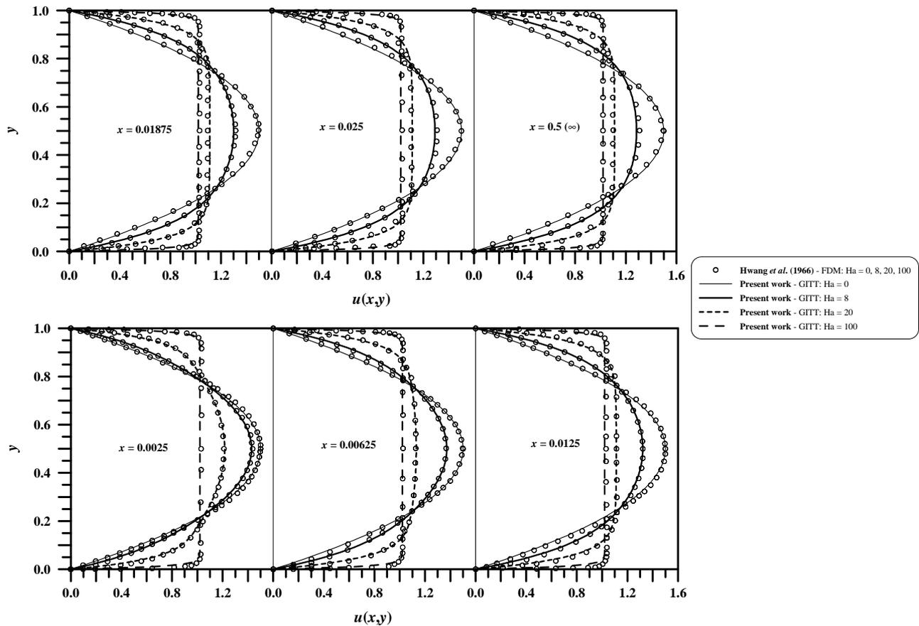
Figure 3. Effect of magnetic field on longitudinal velocity profile development: comparisons with numerical results for  $Ha = 0, 8, 20$  and  $100$
