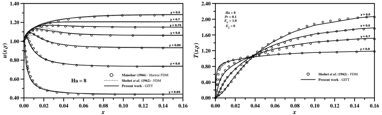
Figure 4. Development behavior of the (a) Longitudinal velocity and (b) Temperature, for different transversal coordinates. Comparisons with other numerical results for  $Ha = 8$ ,  $Pr = 0.1$ ,  $E_c = 1.0$  and  $E_z = 0$ .
