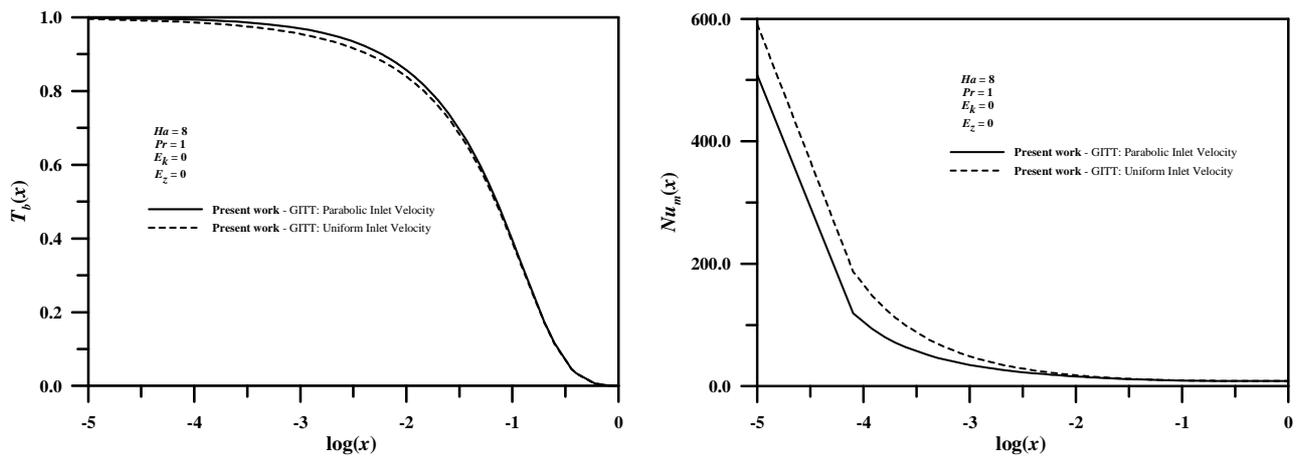
Figure 1. Effect of inlet velocity profile on: (a) Bulk mean temperature and (b) Average Nusselt number, for  $Ha = 8$
