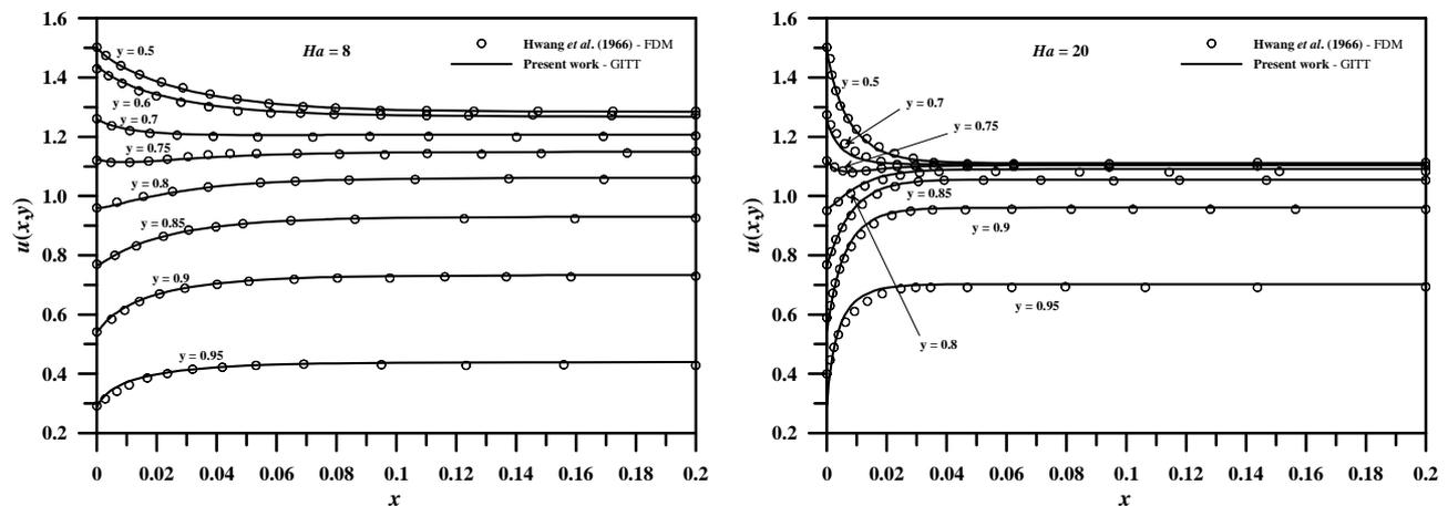
Figure 2. Effect of magnetic field on flow development: comparison with numerical results for different transversal positions: (a)  $Ha = 8$ , (b)  $Ha = 20$
