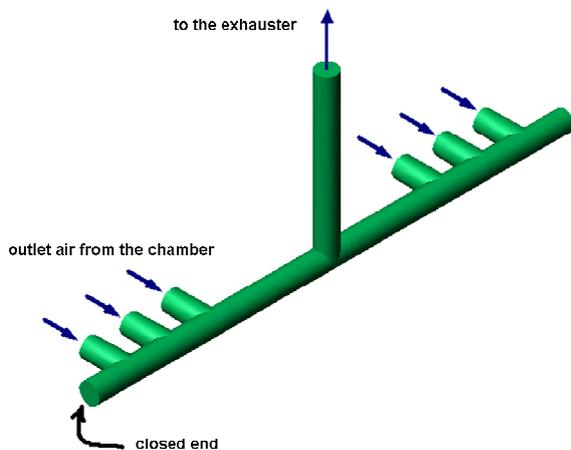
Figure 7. System of exhaustion pipes.
