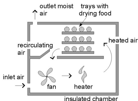
Figure 1. Main thermal processes that are observed in a small size dehydrator.
