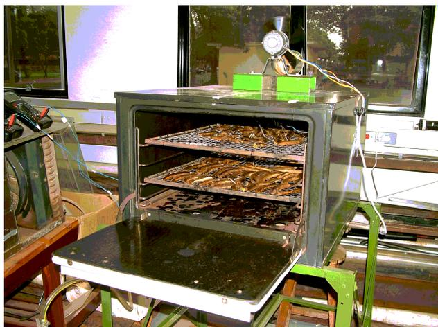
Figure 9. Dryer with the load of bananas.
