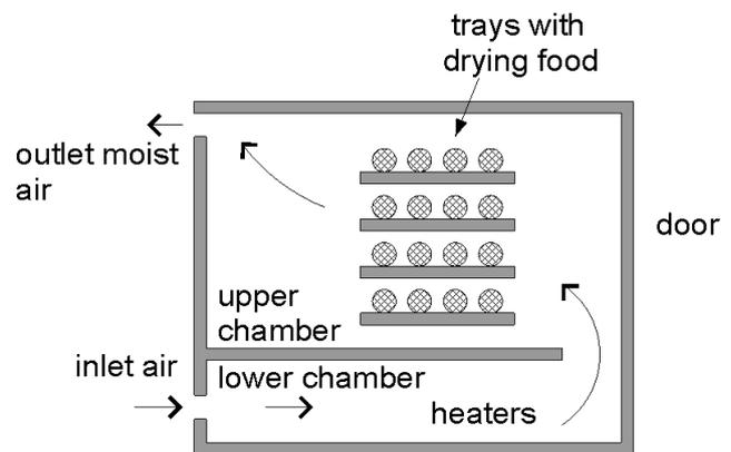
Figure 6. Side view of the dryer, showing the new path the air will follow inside the chamber.
