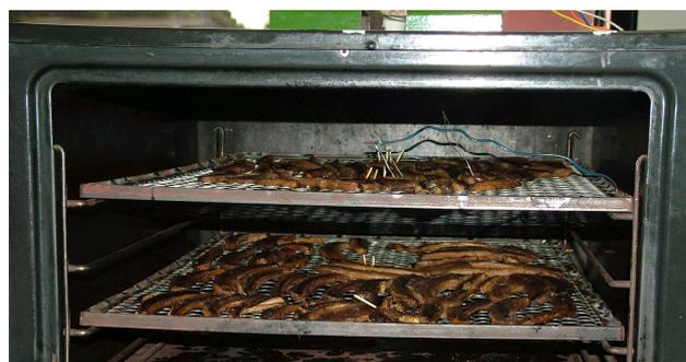
Figure 10. Detail of the load of bananas, with one of the thermocouples.
