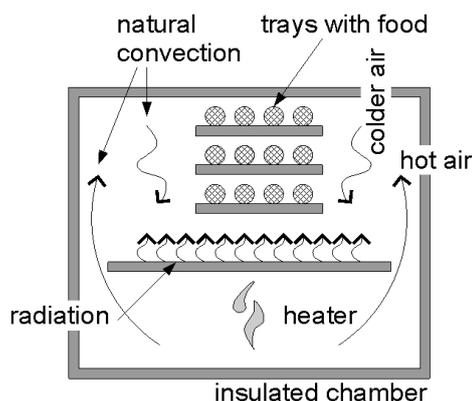
Figure 2. Main thermal processes that are observed in an ordinary oven.
