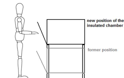
Figure 4. Elevation of the insulated chamber, in order to improve ergonomics.
