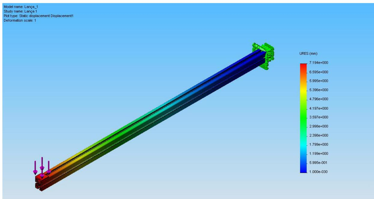
Figure 5. Displacement analysis for 170N
