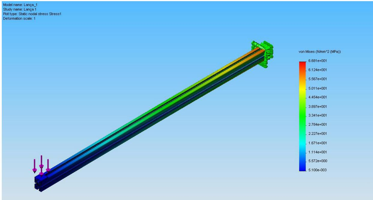
Figure 6. Tension analysis for 500N – Safety factor 2.9
