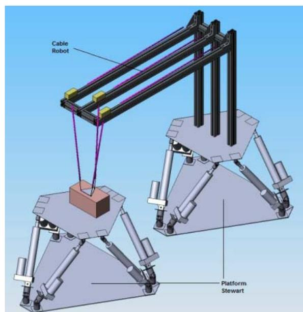
Figure 3. General design of cable robot plataform
