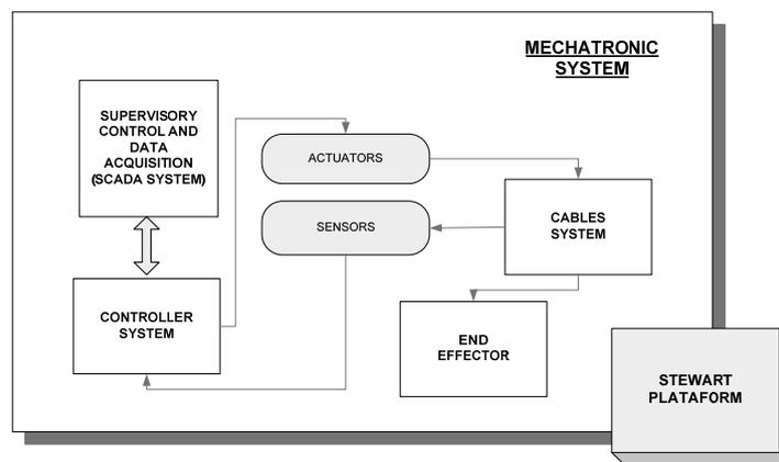
Figure 2. Mechatronic system for cable suspension manipulator
