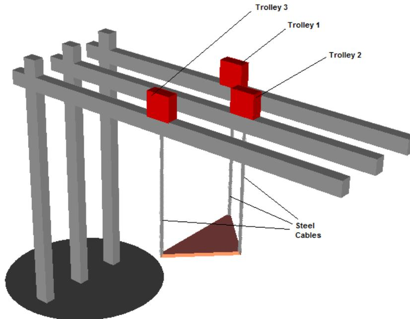
Figure 4. General design of cable robot platform using UM software®.
