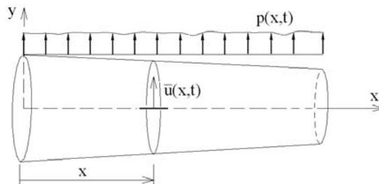
Figure 1. Straight beam with lateral displacement
