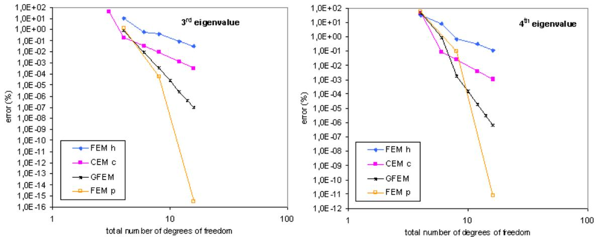
Figure 4. Relative error (%) for the 3<sup>rd</sup> and 4<sup>th</sup> beam eigenvalues
