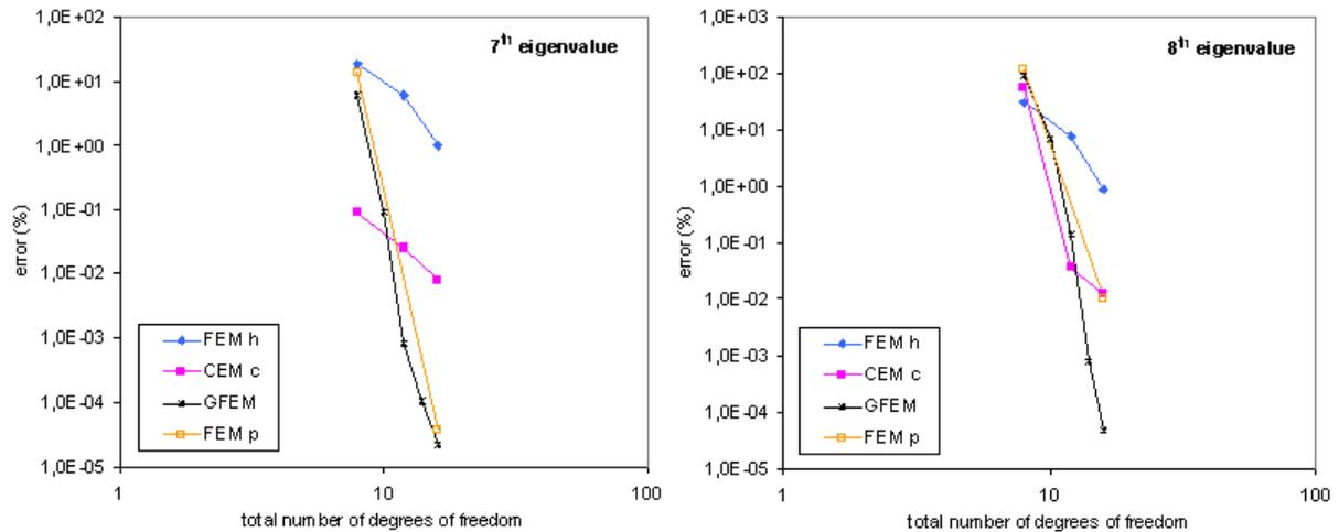
Figure 6. Relative error (%) for the 7<sup>th</sup> and 8<sup>th</sup> beam eigenvalues
