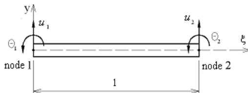
Figure 2. Beam element
