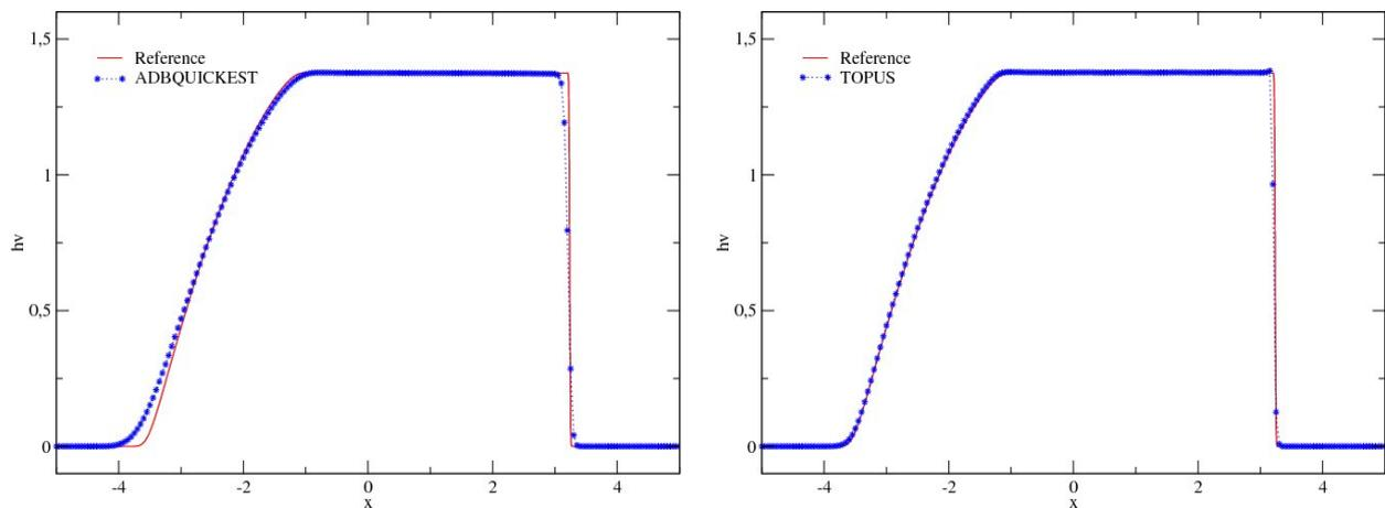
Figure 7. Numerical and reference solutions for the dam break problem.
