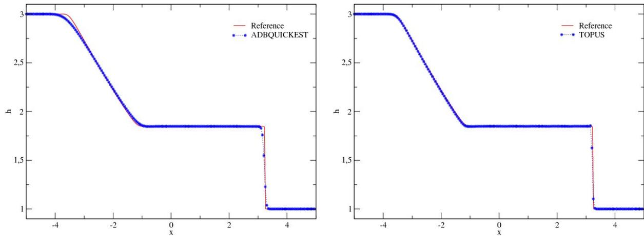
Figure 6. Numerical and reference solutions for the dam break problem.
