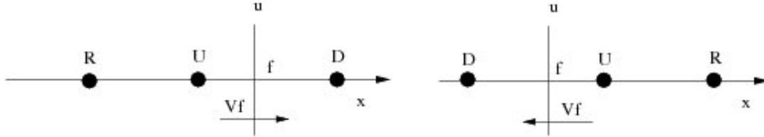
Figure 1. Interfaces and their related grid points for defining normalized variables.
