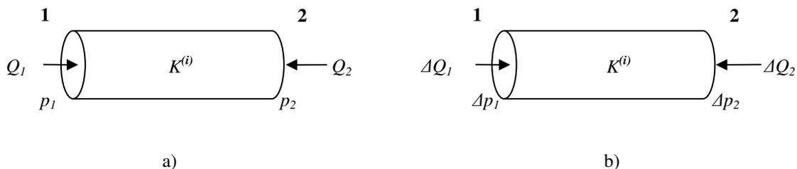
Figure 1. Pipe between nodes 1 and 2, with a) permeability coefficient  $K^{(i)}$ , nodal discharges  $Q_1$  and  $Q_2$ , and nodal pressures  $p_1$  and  $p_2$ . b) Increment in nodal discharges  $\Delta Q_1$  and  $\Delta Q_2$ , and increment in pressures  $\Delta p_1$  and  $\Delta p_2$ .
