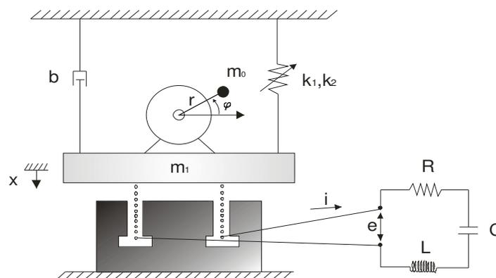
Figure 1 - Schematic of a non-ideal structure coupled to nonlinear electromechanical vibration absorber device [11].
