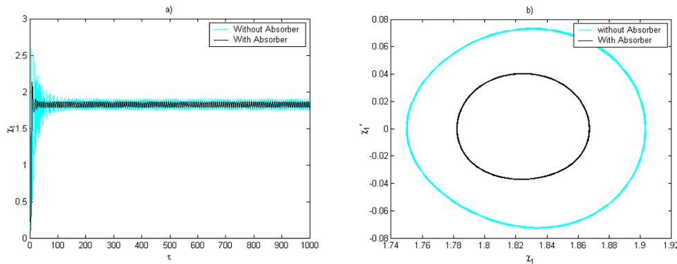
**Figure 3 – a) Time history of the displacement of the mechanical Duffing oscillator, b) Phase portrait. For  $\mu_1 = 14$ .**
