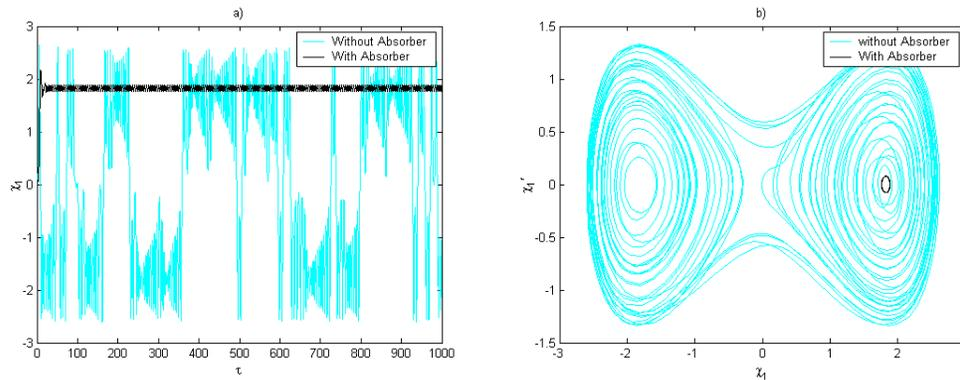
**Figure 5 – a) Time history of the displacement of the mechanical Duffing oscillator, b) Phase portrait. For  $\mu_1 = 19$ .**
