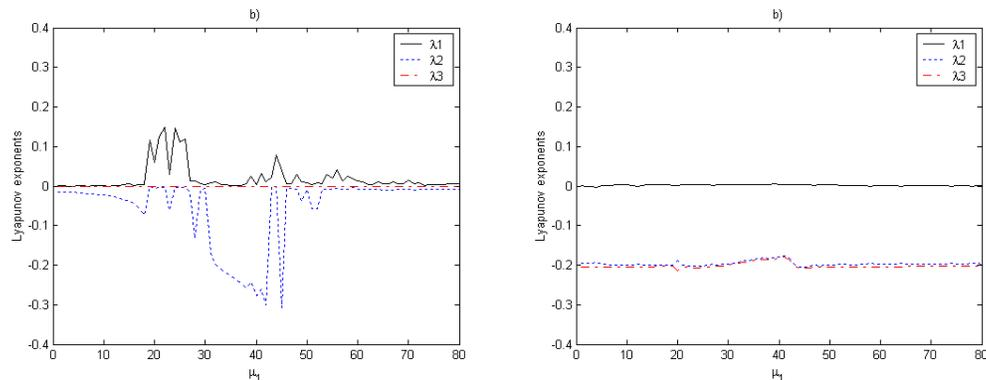
**Figure 9 – Three largest Lyapunov exponents of the system: a) without absorber and b) with absorber.**
