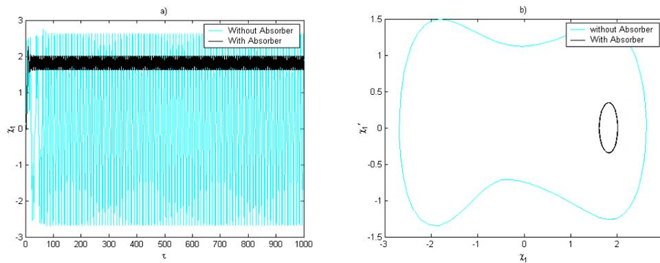
**Figure 6 – a) Time history of the displacement of the mechanical Duffing oscillator, b) Phase portrait. For  $\mu_1 = 28$ .**
