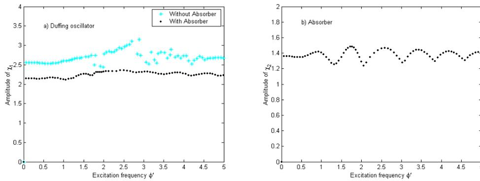
**Figure 2 – a) Frequency response curve for the double-well Duffing oscillator without and with absorber and b) Frequency response curve for the electromechanical absorber.**
