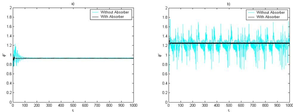
**Figure 8 – Time evolution of the motor velocity: a) for  $\mu_1 = 14$  and b) for  $\mu_1 = 19$ .**
