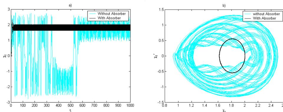
**Figure 7 – a) Time history of the displacement of the mechanical Duffing oscillator, b) Phase portrait. For  $\mu_1 = 43$ .**
