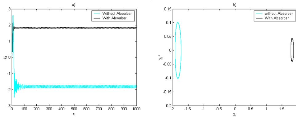
**Figure 4 – a) Time history of the displacement of the mechanical Duffing oscillator, b) Phase portrait. For  $\mu_1 = 15$ .**
