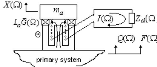
Figure 1. Electro-viscoelastic vibration neutralizer configuration
