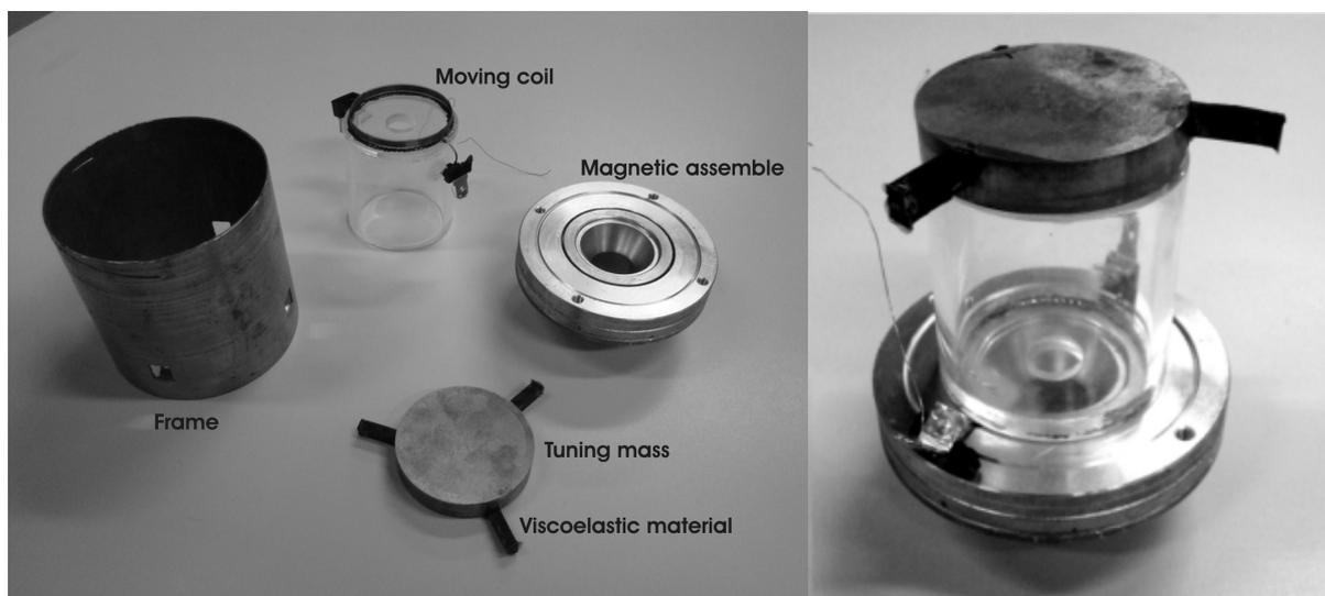
Figure 5. Neutralizer pieces and mounting process
