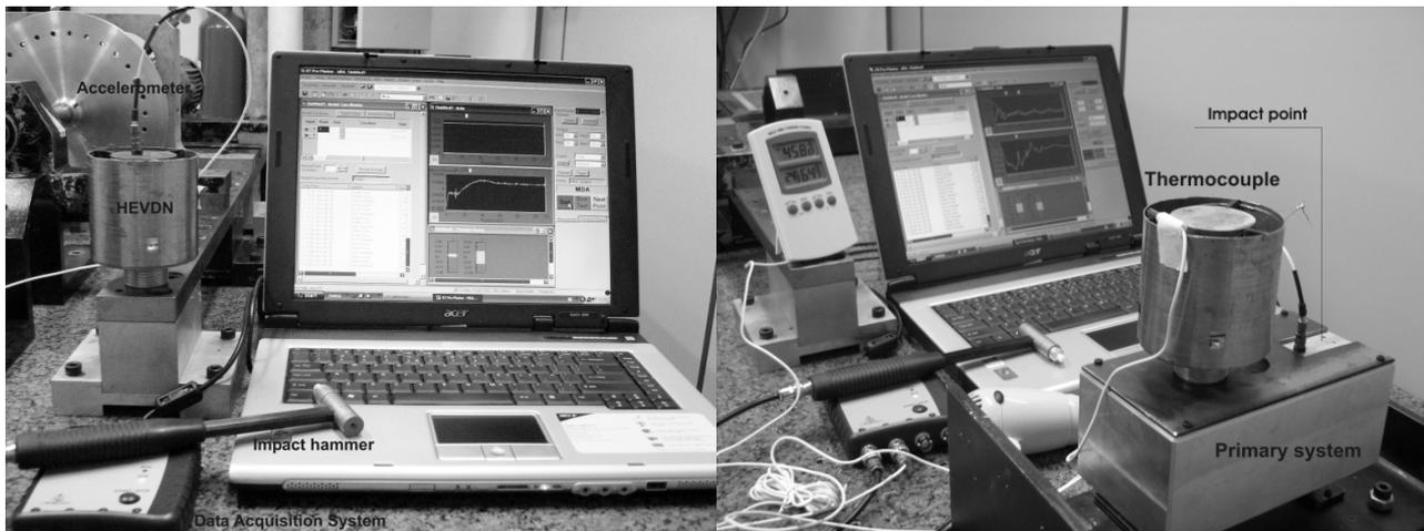
Figure 6. Neutralizer inertance measurement scheme (left) and composite system inertance measurement scheme (right)
