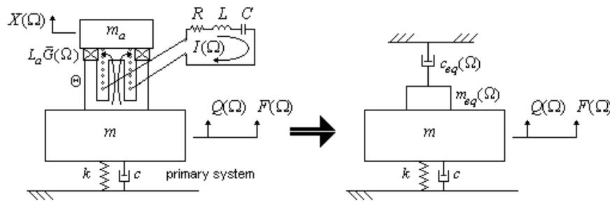
Figure 2. Equivalent quantities for the electro-viscoelastic vibration neutralizer
