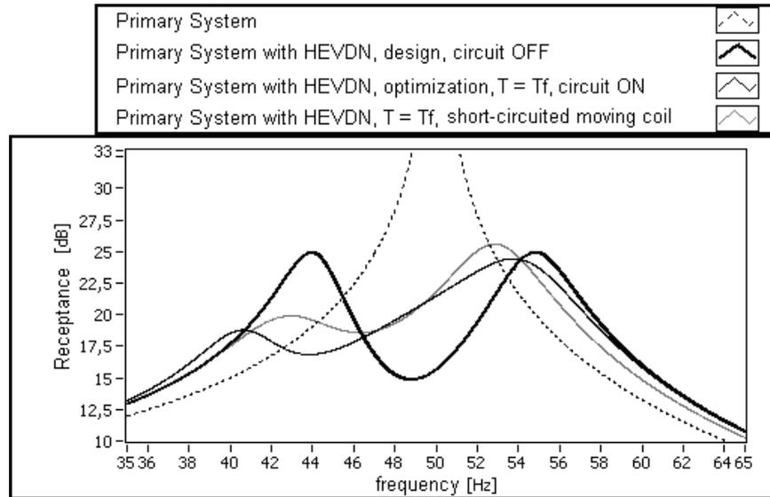
Figure 4. Comparison: simulation 1b versus short-circuited moving coil
