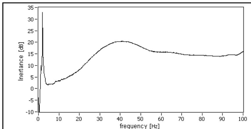
Figure 7. Neutralizer frequency response
