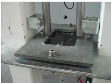
Figure 4. Coupon fixed within the Boeing test window
