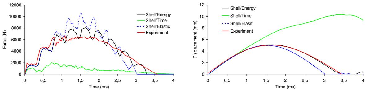
Figure 8. Force histories (a) and displacement vs. time at medium energy
