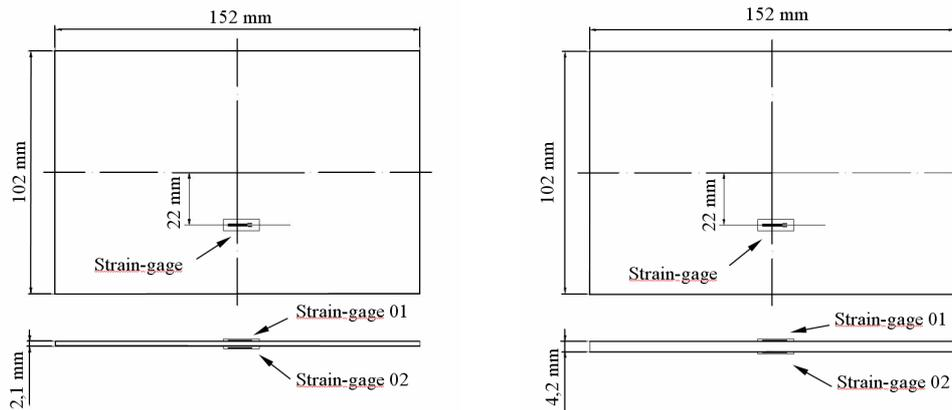
Figure 3. Dimension of the laminate 01 and position of the strain gages (a) Dimension of the laminate 02 and position of the strain gages (b)
