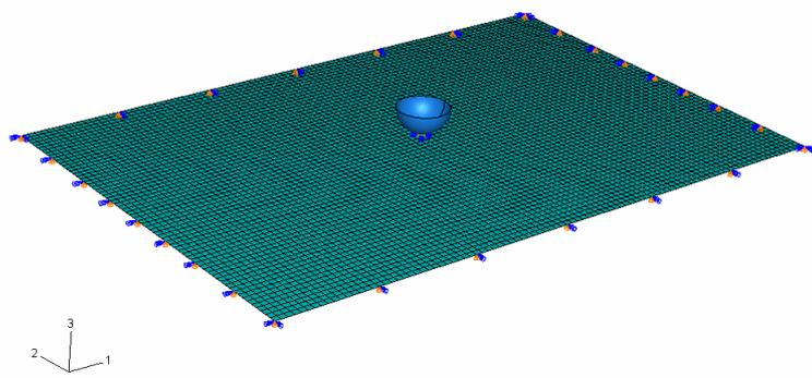
Figure 1. Mesh and boundary conditions of the numerical impact model
