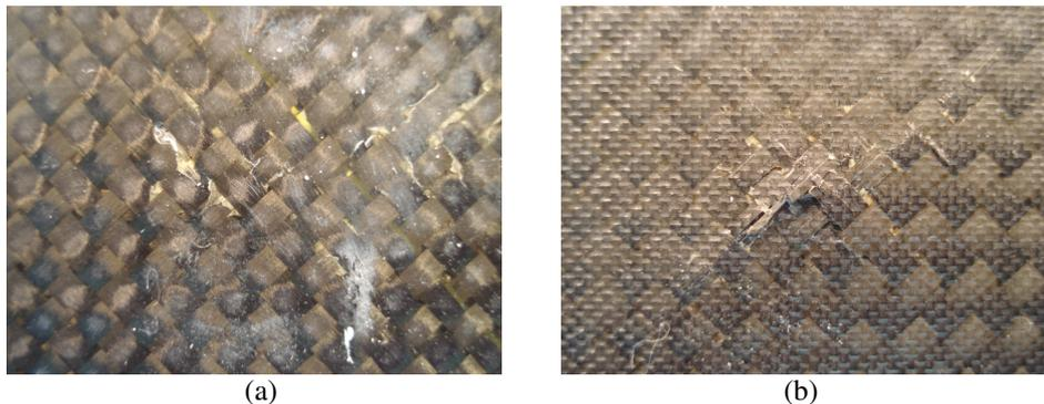
Figure 10. Front laminate face (a) and rear laminate face (b) after impact test at medium energy
