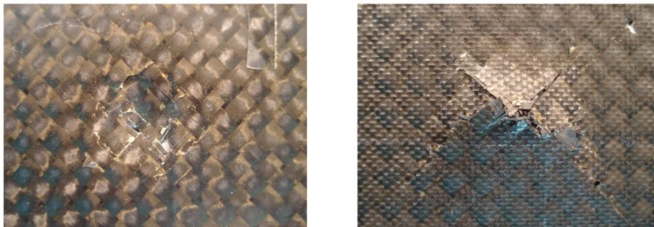
Figura 7. (a): Top face and (b): Bottom face of the impacted plate
