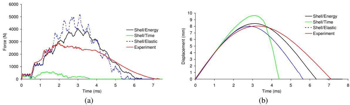
Figure 5. Force histories (a) and displacement vs. time at medium energy
