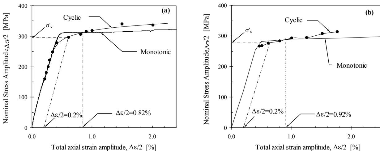
Figure 5. Monotonic and cyclic stress-strain curves: (a) alloy 6082-T6, (b) alloy 6061-T651.
