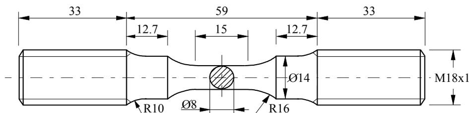
Figure 3. Geometry and dimensions of the specimens used in the low-cycle fatigue tests (dimensions in mm).
