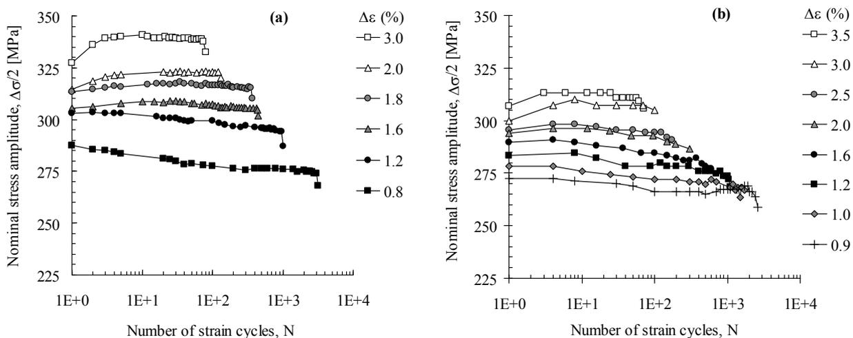
Figure 4. Stress amplitude *versus* number of cycles for fully-reversed strain-controlled tests: (a) alloy 6082-T6, (b) alloy 6061-T651.
