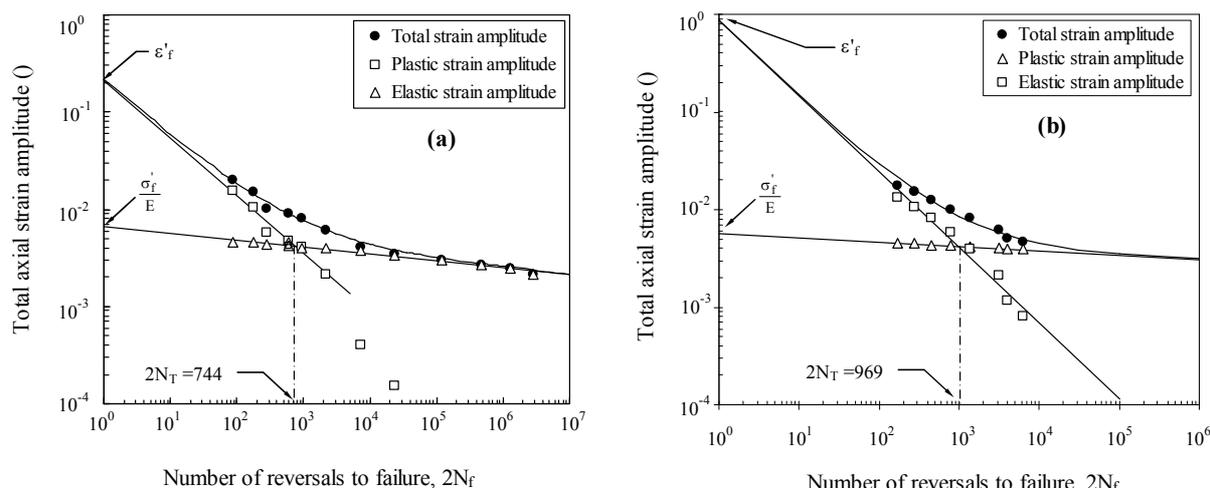
Figure 6. The total strain amplitude versus life curve obtained from the superposition of the elastic and plastic strain amplitude versus life curves: (a) alloy 6082-T6, (b) alloy 6061-T651.
