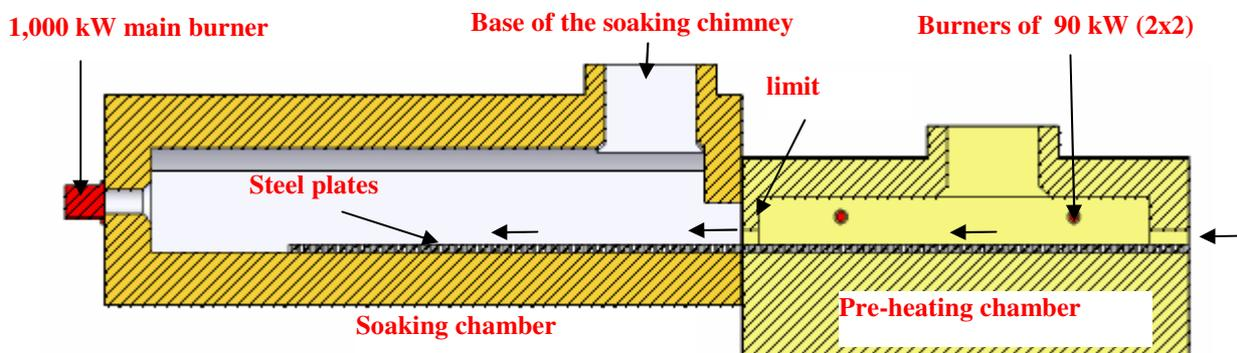
Figure 1. Current design of the furnace
