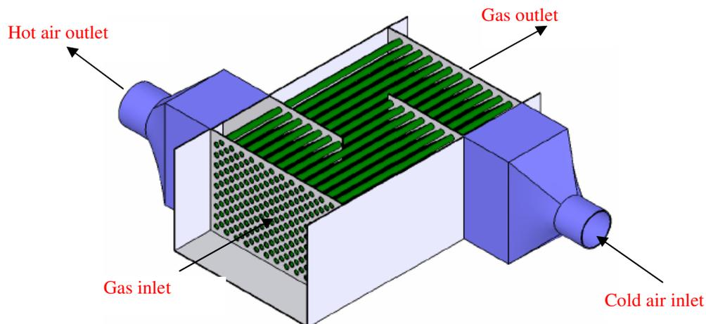
Figure 4. Configuration of the recovery heat exchanger proposed
