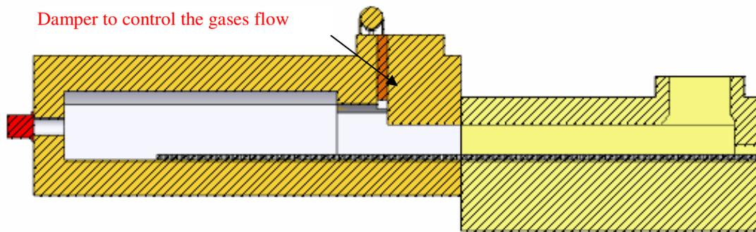
Figure 2. New design for the furnace with control damper of combustion gases and only one chimney
