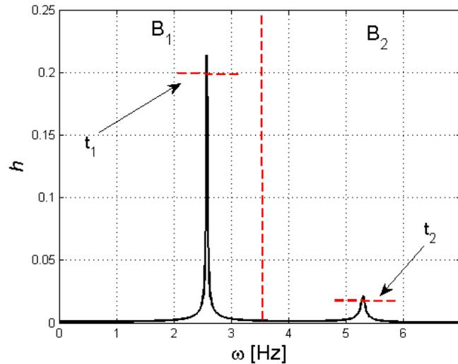
Figure 2. Frequency response function with targets  $t_1$  and  $t_2$ .
