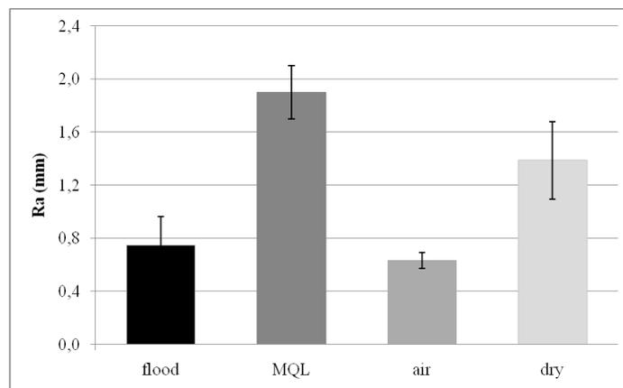
Figure 3. Surface roughness as a function of cooling-lubrication condition
