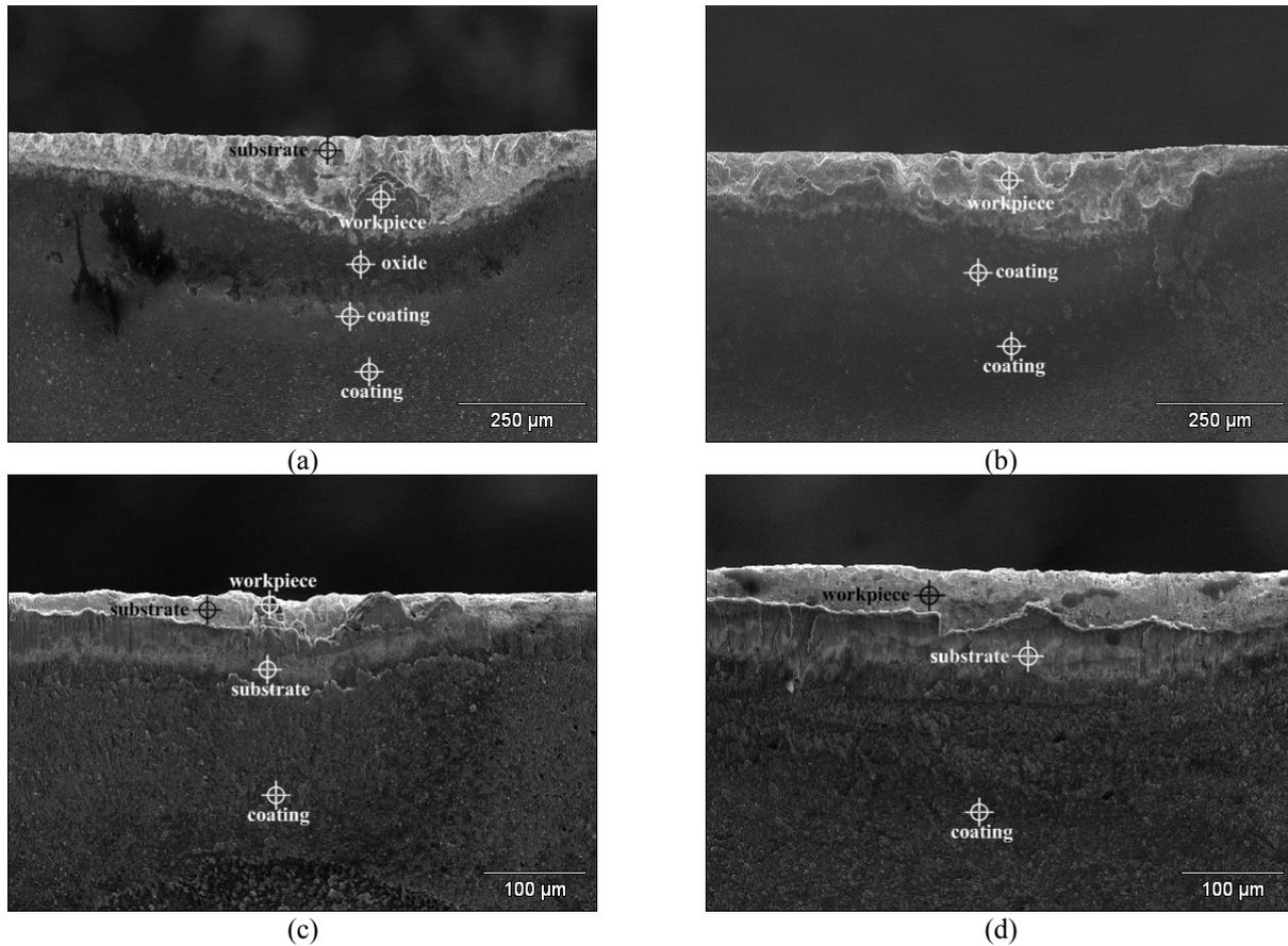
Figure 2. SEM pictures of worn tools as a function of cooling-lubrication condition:
