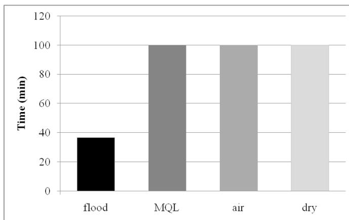
Figure 1. Tool life as a function of cooling-lubrication condition
