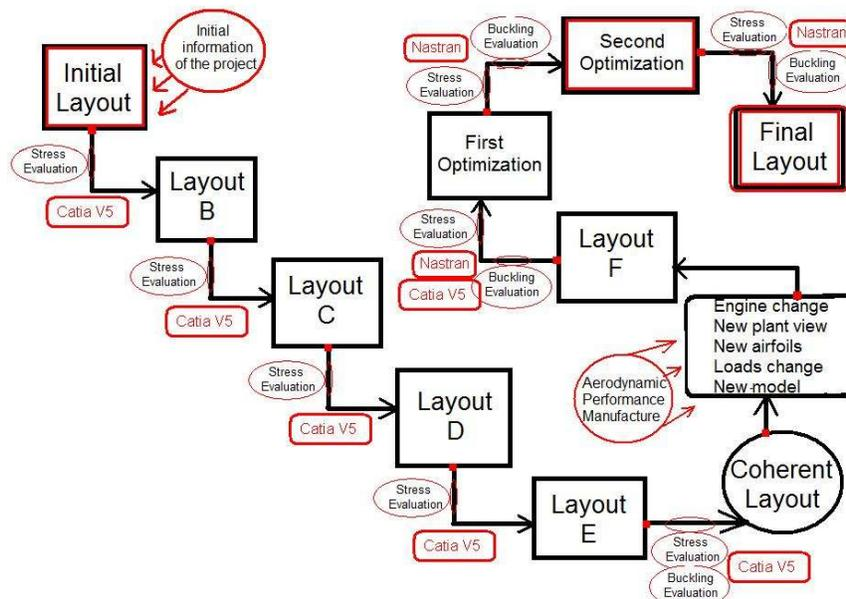
Figure 2. Detailed block diagram describing each step of the structural layout converging process
