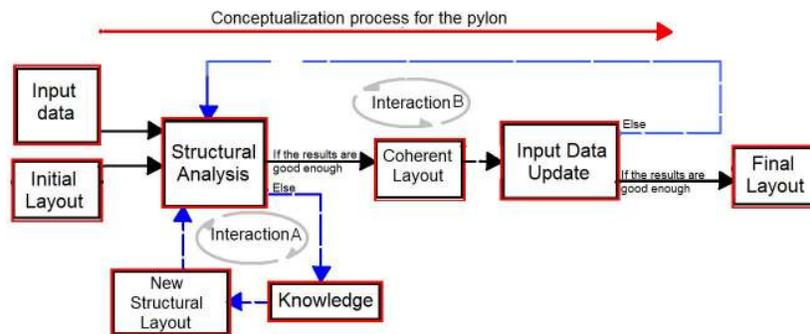
Figure 1. Block diagram for the conceptualization process of the pylon region
