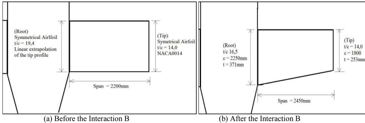
Figure 4. Plant view for the pylon wing – (a) Plant view for Initial Layout to Layout E. (b) Plant view for Layout F to Final Layout. “c”: chord. “t”: thickness.
