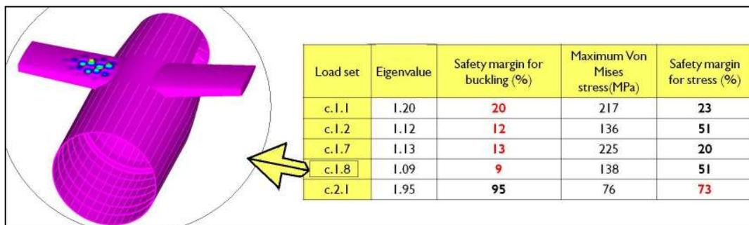
Figure 11. Results for the Final Layout. Detailed image for the buckling result of the load set c.1.8.
