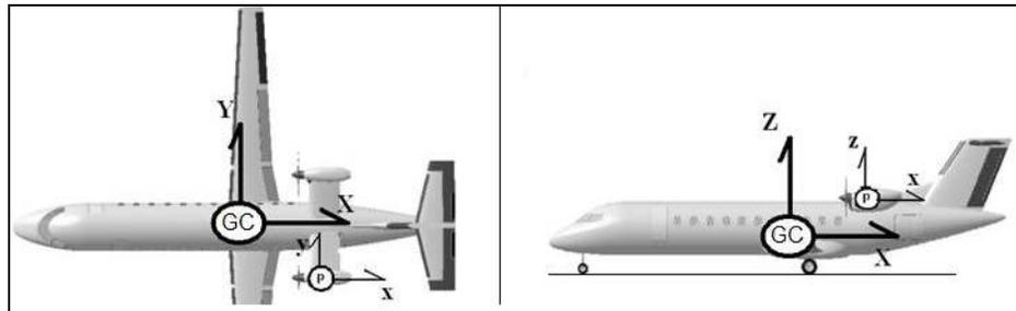
Figure 3. Reference system of loads. Top View of the airplane in study on the left side and Side View on the right
