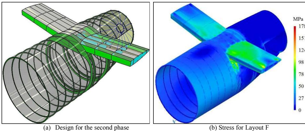
Figure 9. Pylon region after the update of the income information. (a) Three Dimensions model showing the internal disposition of structures (b) Von Mises stress distribution for Layout F loaded with c.1.7.
