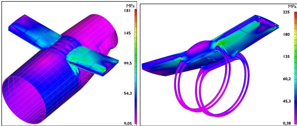
Figure 10. Von Mises stress distribution using Nastran®. (a) Results for Load set c.1.7 applied on Layout F. (b) Results after two optimizations of thickness with hidden fuselage.
