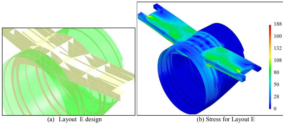
Figure 8. Layout E designed for reduced stress concentration – (a) Layout E design using a concept of continuity along the structure (b) Von Mises stress distribution for Layout E showing a maximum of 188MPa.
