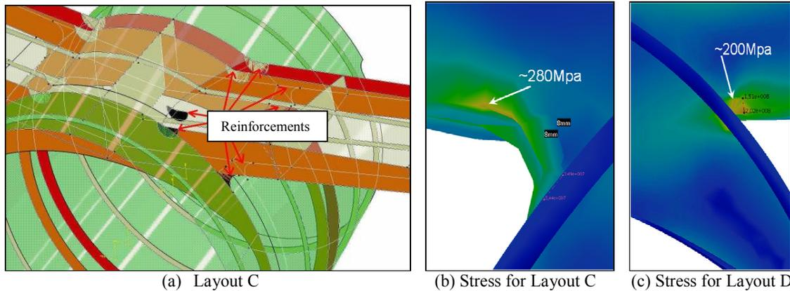
Figure 7. Comparison for Layout C and Layout D – (a) Layout C with reinforcements located at the stress concentration radii. (b) Von Mises stress distribution for Layout C showing a maximum of 280MPa. (c) Von Mises stress distribution for Layout D showing a maximum of 200MPa having no radii for the joint.
