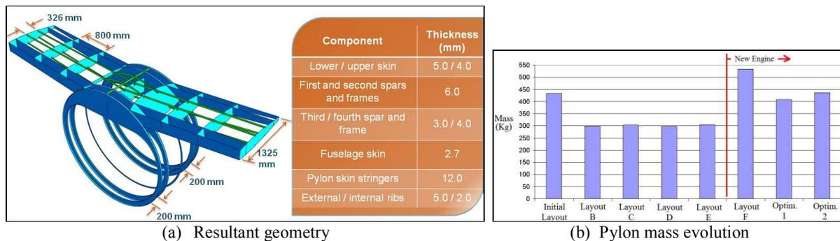
Figure 12. Resultant and evolution. (a) Main dimensions for the Final Layout disclosure. (b) Mass of the pylon along the development process.
