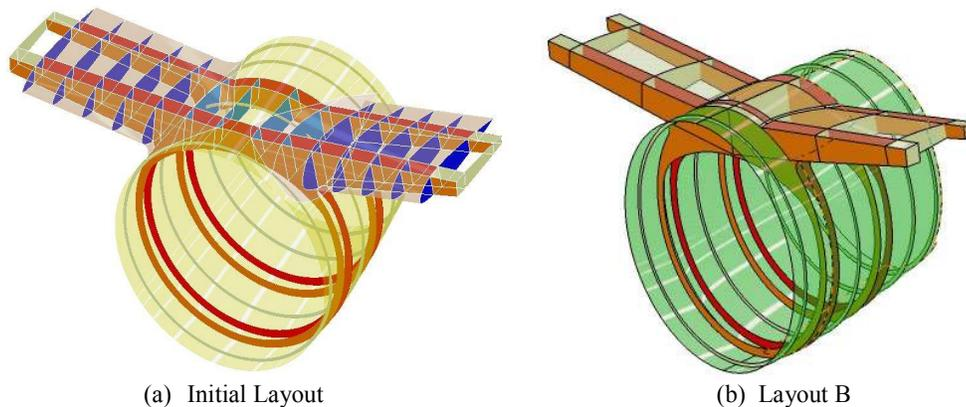
Figure 6. Three dimensions model for the pylon region – (a) Initial Layout used as an input from the market and airplane configuration study. (b) Layout B including the identified need from the initial design.
