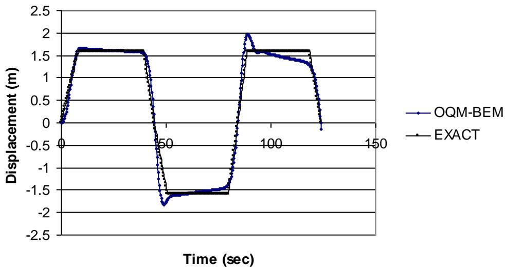
Figure 2. Time variations of vertical displacement of point A of a rectangular plate under a triangular tensile load.
