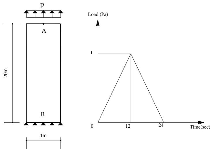
Figure 1. A long and rectangular plate under to a cyclic load.
