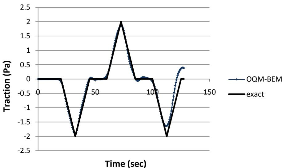
Figure 3. Time variation of normal traction at point B of a rectangular plate under a triangular load.
