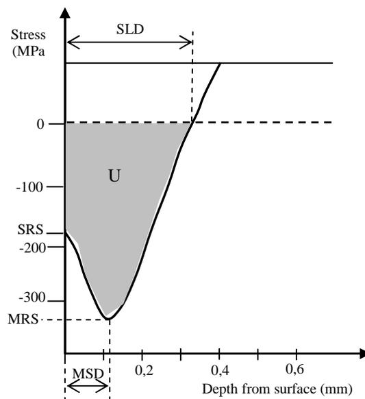
Figure 2. Typical profile of residual stresses due to peen forming.
