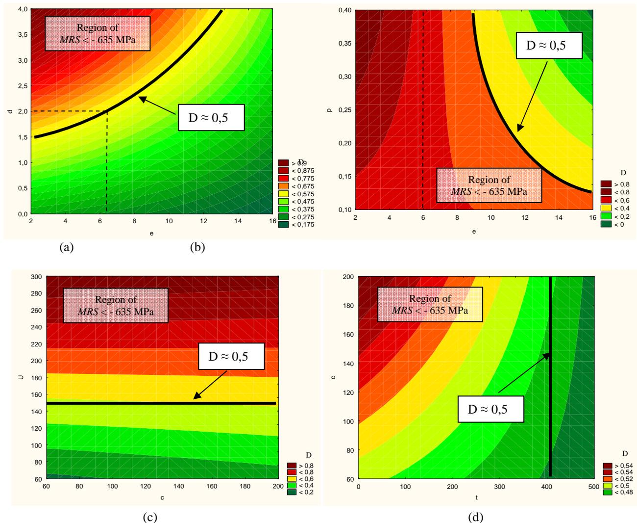
Figure 6: Contour plots for residual stress desirability function of the following primary independent pair of variables: (a) Plate thickness vs. Shot diameter; (b) Plate thickness vs. Blast pressure; (c) Coverage vs. Energy of deformation; (d) Static load vs. Coverage.
