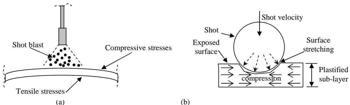
Figure 1. Plate subjected to peen forming.
