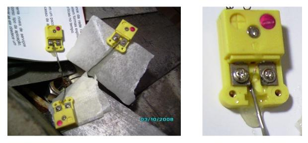
Figure 9. Thermocouples wires fixed on the connectors
