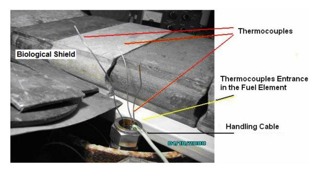
Figure 6. Place of the rupture of the thermocouples in the instrumented fuel element
