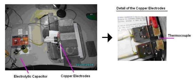
Figure 7. Assembly used for removal of the thermocouples shield by electric charge
