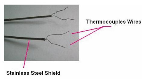
Figure 8. Two thermocouples after the shield and the MgO isolation had been removed
