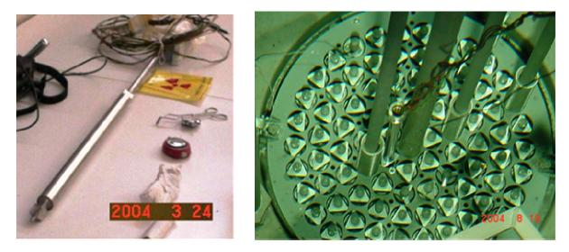
Figure 1. Instrumented fuel element before and after its positioning in the IPR-R1 reactor core.
