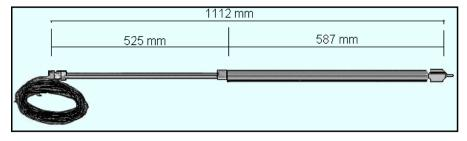
Figure 3. Instrumented fuel element (serial number 6821TC)
