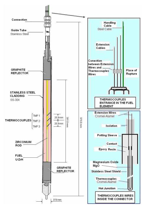
Figure 4. Instrumented fuel element and thermocouple connector detail
