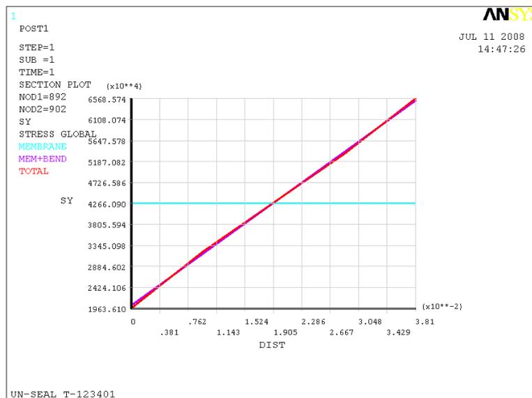
Figure 10 – Graph of linearized stresses.  $P_m = 42,76$  MPa;  $P_b = 22,46$  MPa.
