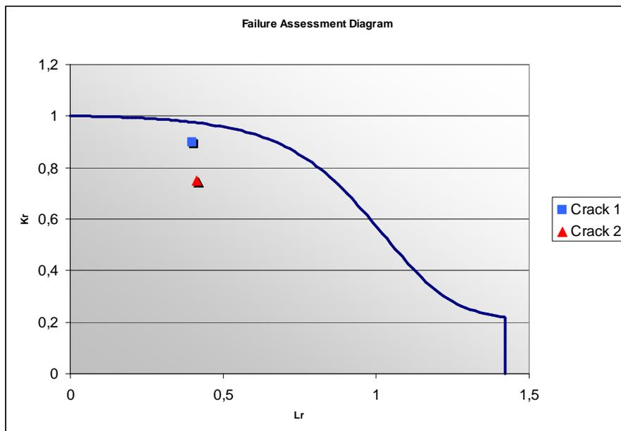
Figure 12 – Flaw sizes according to BS-7910 nomenclature. Dots below the blue line are considered safe.
