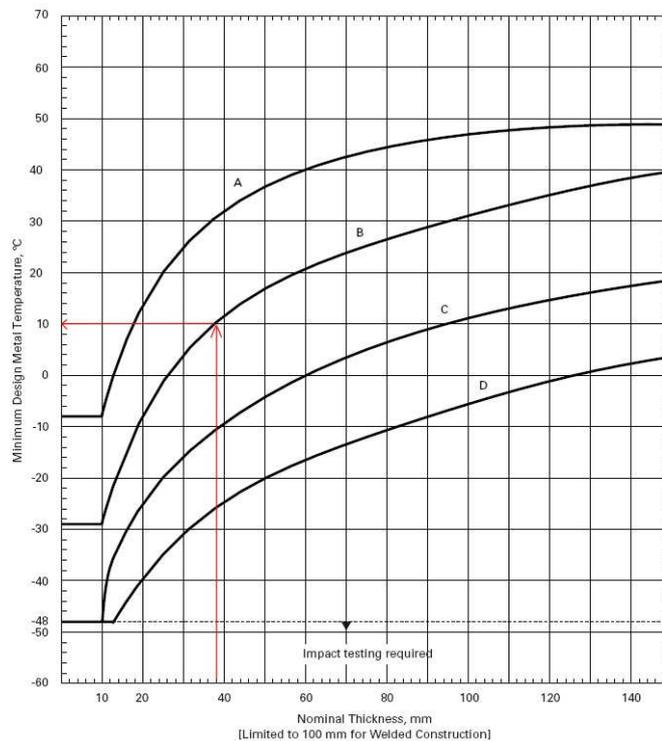
Figure 5 – Curve UCS-66. The red arrows represent the studied case, a 38 mm thickness SA-516 grade 70 plate.
