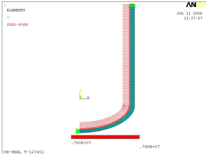
Figure 7 – Axi-symmetric FEM model of the DEA tower. Design pressure = 7.6 MPa.
