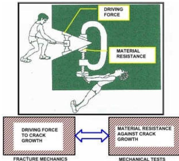
Figure 1 – Fracture mechanics X materials strength.
