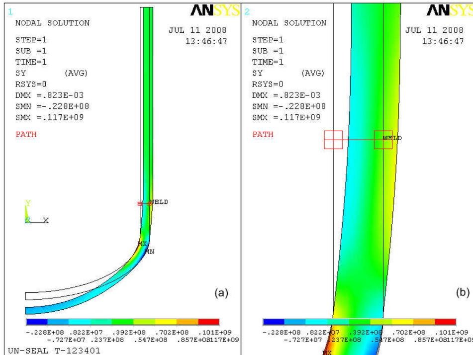
Figure 9 – (a) Longitudinal stress ( $S_y$ ) distribution in the tower. (b) Detail of the stress distribution close to the cracks' site. The underformed configuration is also represented (black lines). Stresses are shown in Pa.
