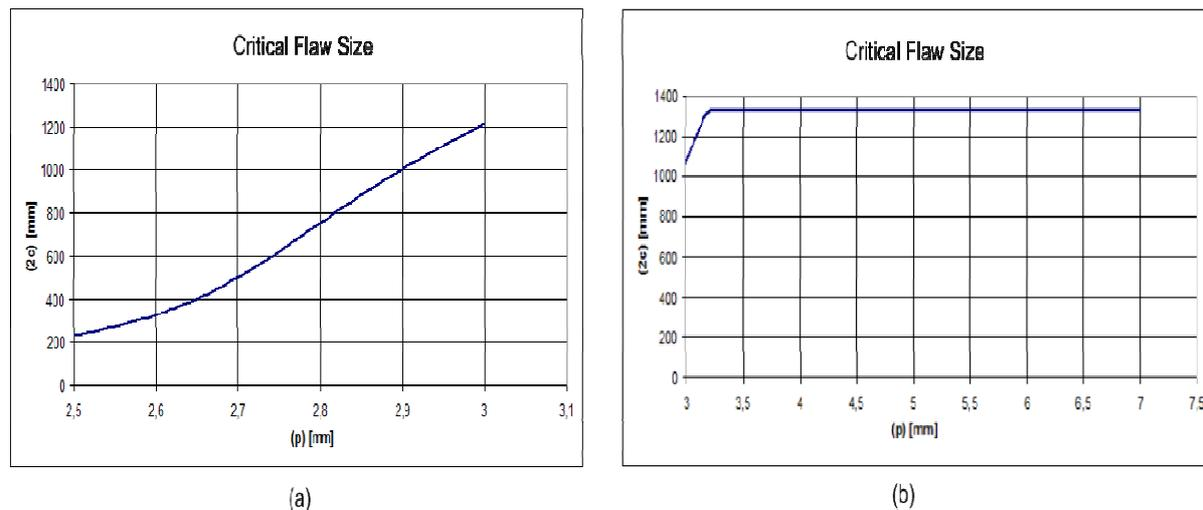
Figure 13 – Critical flaw sizes for (a) crack 1 and (b) crack 2. Height is constant, while varying length ( $2c$ ) against ligament ( $p$ ).
