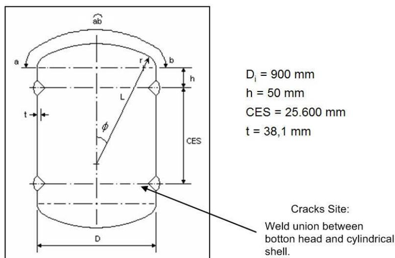
Figure 3 – DEA absorber tower main geometry.
