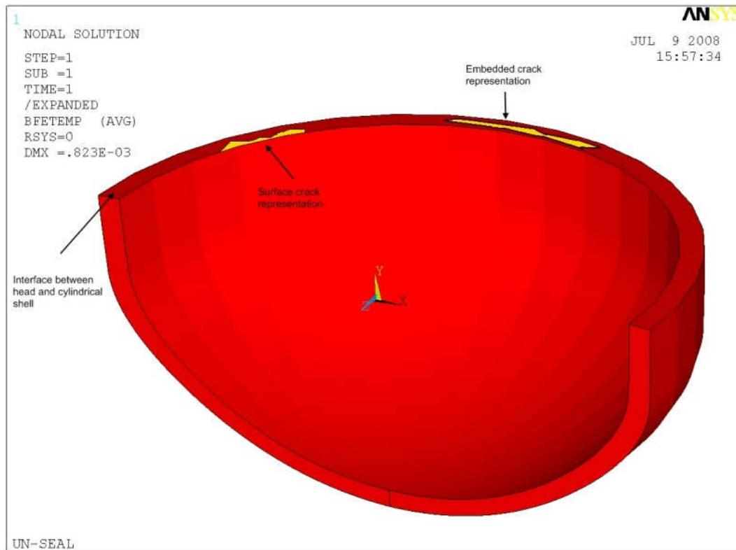
Figure 4 – Geometric representation of the cracks location.
