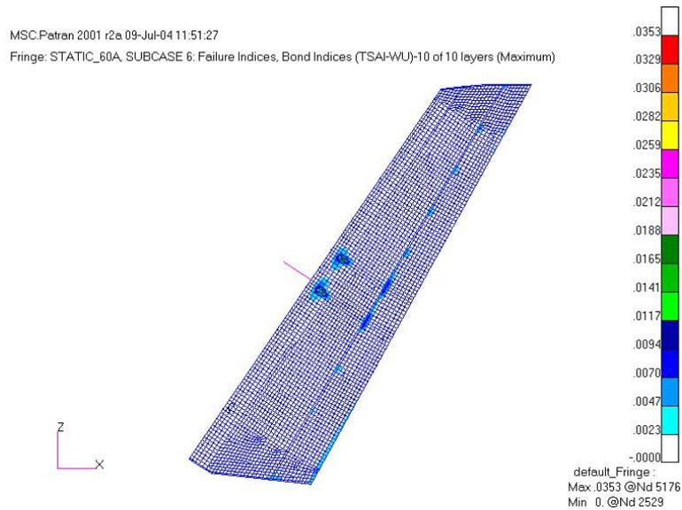
Figure 7. Tsai-Wu failure index results.
