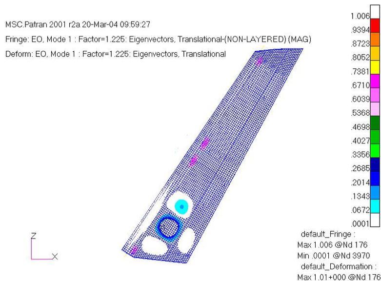
Figure 8. Buckling results using Lanczos method (Sundar, 2000).
