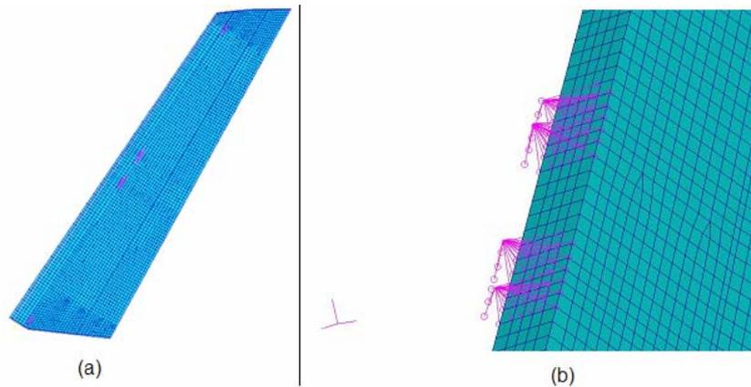
Figure 5. (a) FEM model of the rudder and (b) hinges modeled as rigid bodies (MPC).
