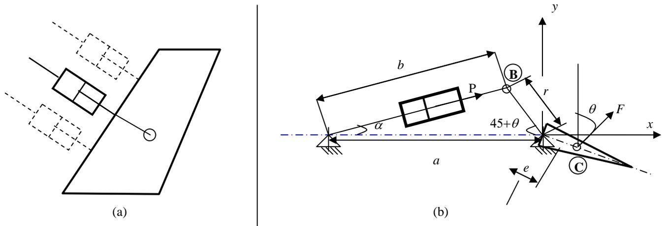
Figure 3. (a) Idealized single actuator aligned with the pressure center and (b) variables used in the formulation.
