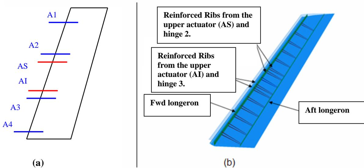
Figure 1. Schematic position of the hinges (a) and ribs position (b).
