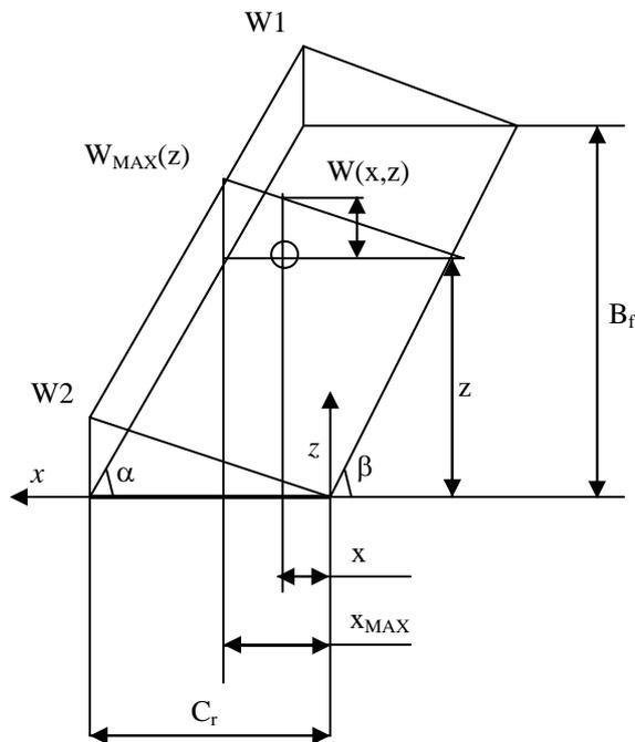
Figure 2. Idealized distribution of load at the rudder.
