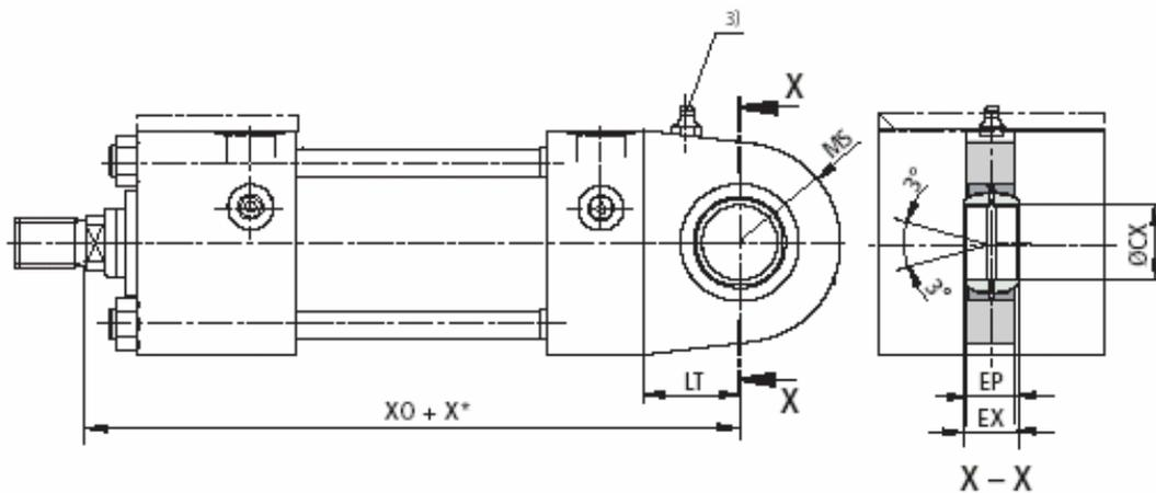
Figure 4. Actuator dimensions
