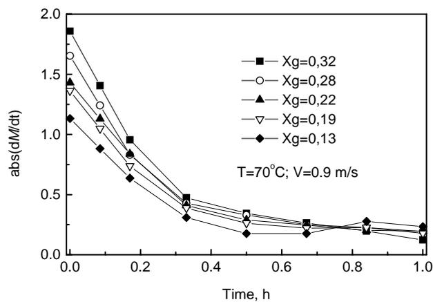
Figure 6. Dynamics of absolute drying rate variation in a thin layer at different initial grain moisture contents
