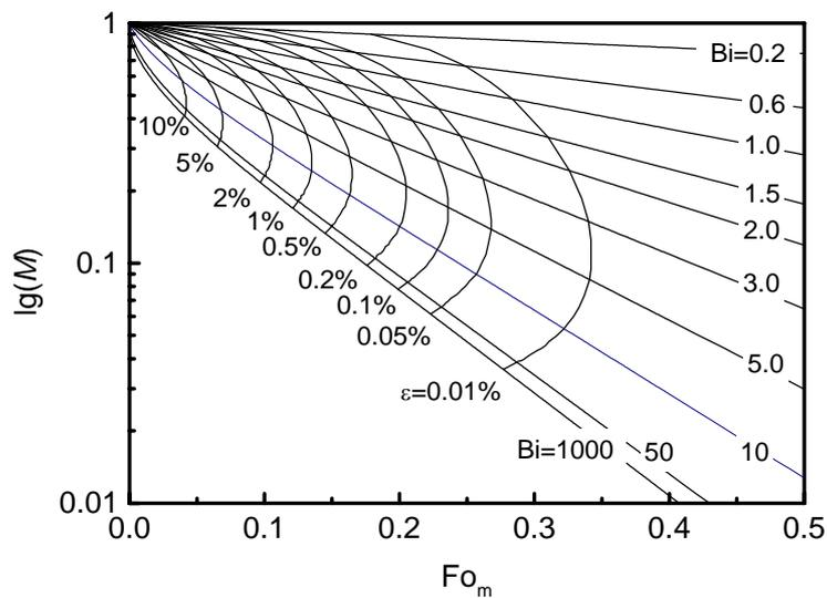
Figure 2. Start of regular regime for a sphere with variation of moisture content  $M$  as function of  $Fo_m$ ,  $Bi_m$  criteria for various tolerances.
