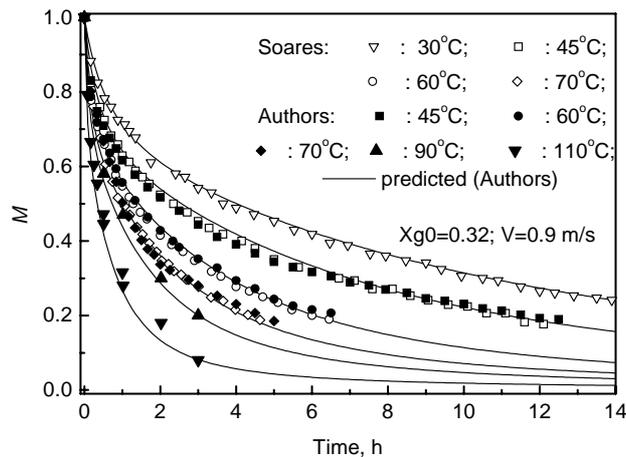
Figure 7. Temperature influence on soybean drying dynamics.
