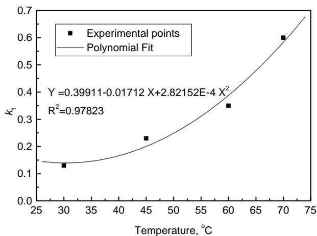
Figure 10. Dependence of coefficient  $k_1$  from drying temperature.
