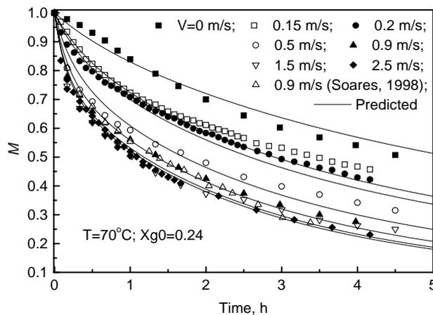
Figure 8. Velocity influence on soybean drying dynamics.
