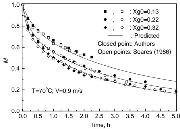
Figure 4. Soybean drying dynamics in a thin-layer at different initial grain moisture contents:  $T=70^{\circ}\text{C}$ .
