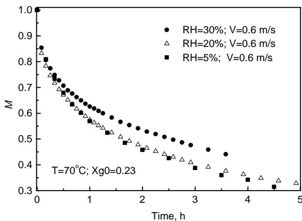
Figure 12. Influence of air relative humidity on thin-layer drying.
