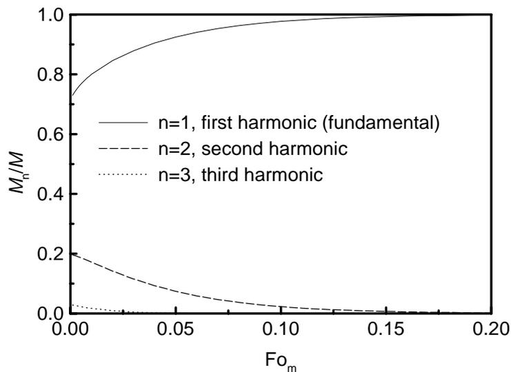
Figure 1. Dynamics of distribution of moisture content on harmonical components in solution of the system (8)-(10),  $Bi_m=10$ .
