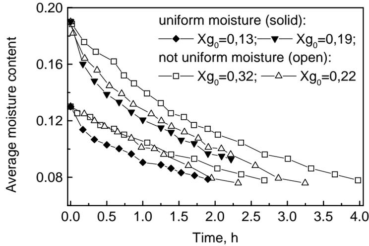
Figure 9. Thin-layer drying dynamics for "uniform" and "non uniform" initial distribution of moisture inside of grain.
