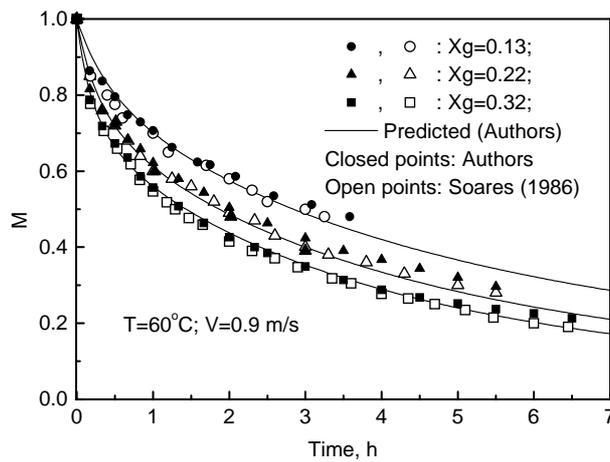
Figure 5. Soybean drying dynamics in a thin-layer at different initial grain moisture contents:  $T=60^{\circ}\text{C}$ .
