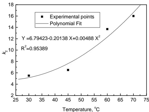
Figure 11. Dependence of coefficient  $k_2$  from drying temperature.
