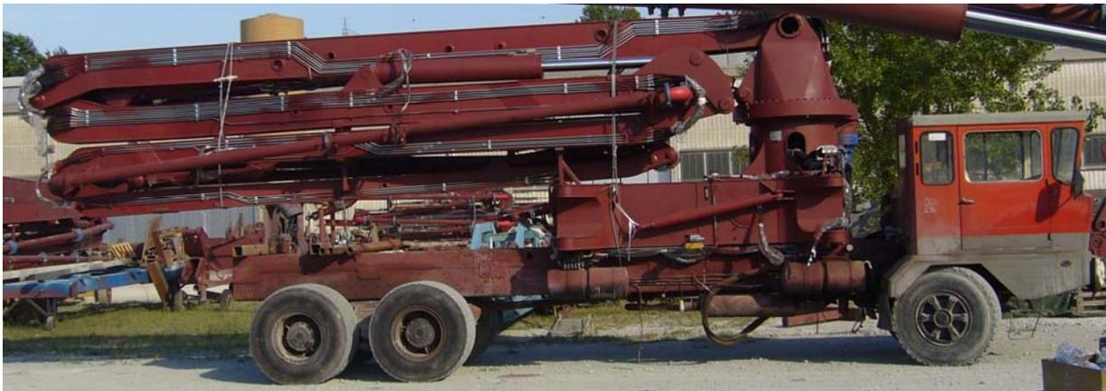
Figure 1c. Example of the folded assembly of an equipment for pouring concrete, carried by a suitable tractor unit.
