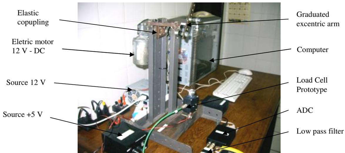
Figure 16. The repeatability test device
