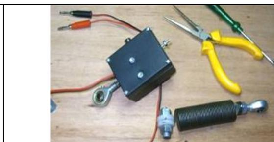
Figure 12. Load cell and amplifier circuit in a box
