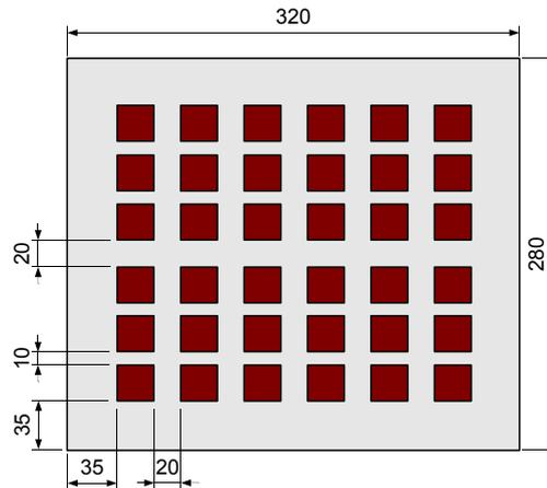
Figure 1. Aluminum plate with thirty-six PZT-5H piezoceramic patches bonded to one of its surfaces (dimensions in mm).
