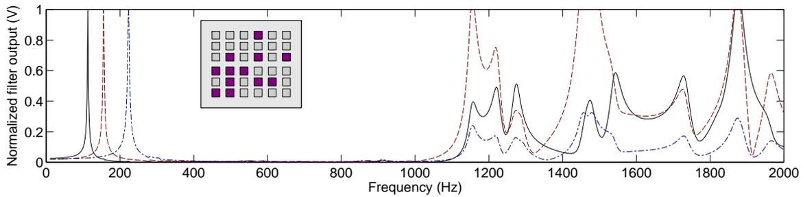
Figure 2. Normalized output of the modal filter designed for the isolation of the first three vibration modes.
