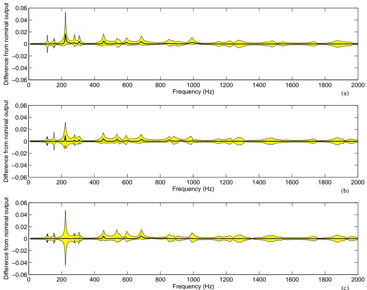
Figure 5. Difference from nominal model of filter output mean and confidence intervals for the isolation of first (a), second (b) and third (c) modes.
