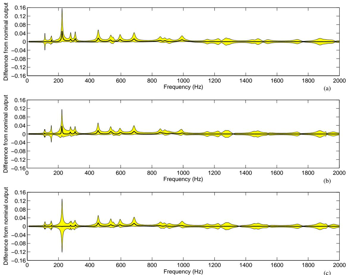
Figure 6. Difference from nominal model of filter output mean and confidence intervals for the isolation of first (a), second (b) and third (c) modes.
