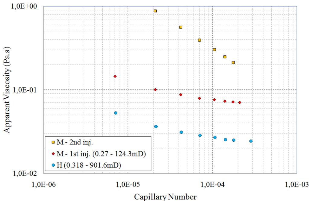
Figure 4. Behavior of the apparent viscosity with the capillary number.
