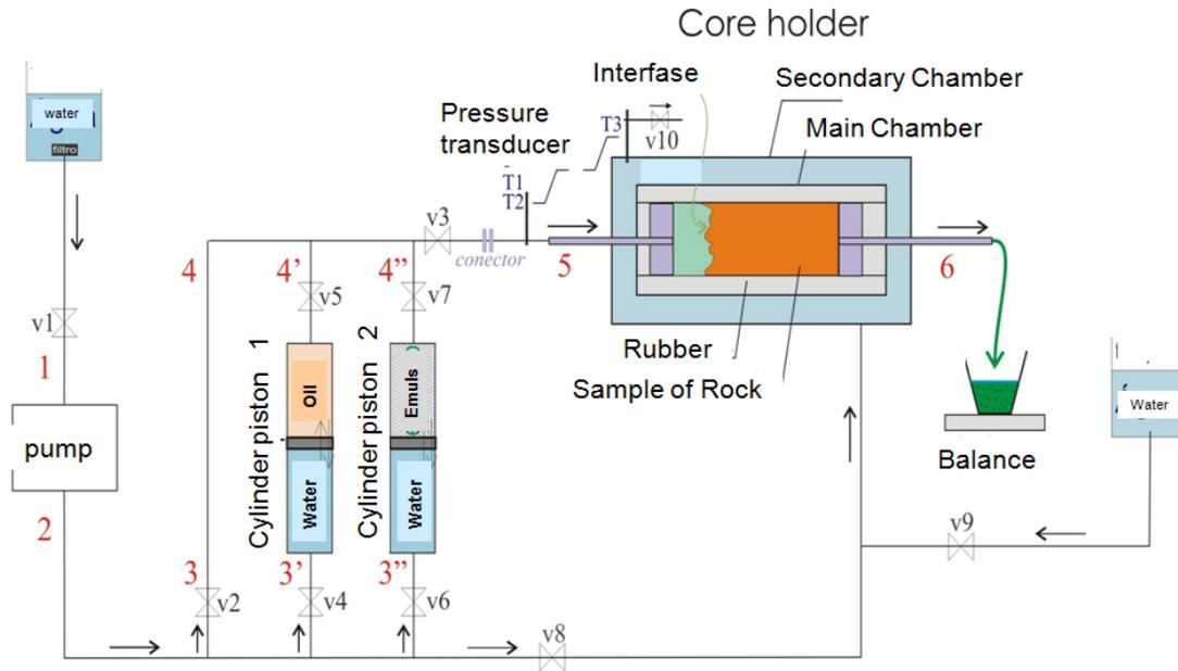
Figure 2. Schematic representation of the experimental apparatus
