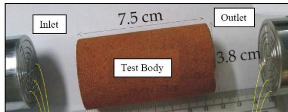
Figure 3. Sandstone sample (Sample of Rock in the Fig. 2)
