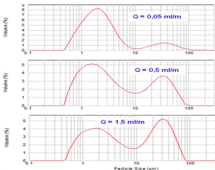
Figure 5. Drop size distribution of the produced emulsion on the 2<sup>nd</sup> injection through core M.
