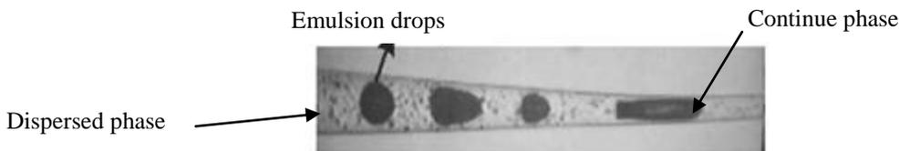
Figure 10. Image of the emulsion flow in a capillary, from Cobos *et al.* (2009).
