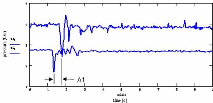
Figure 1. Characteristic pressure waveforms during a simulated leak test.
