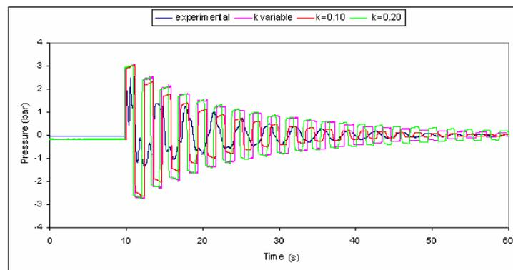
Figure 7. Comparison between numerical and experimental results in the pipeline without leak.
