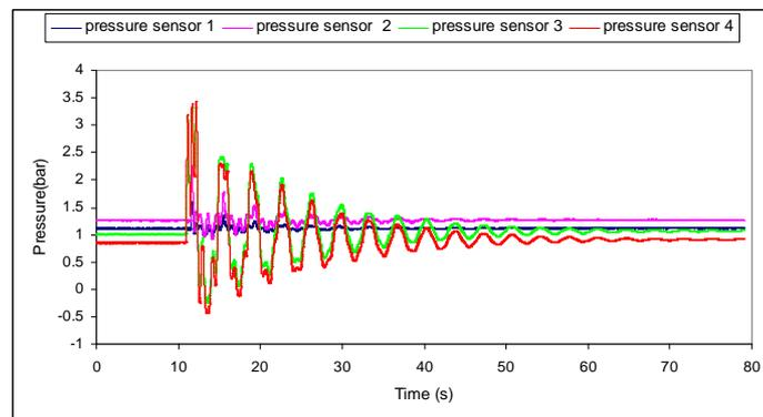
Figure 3. Experimental results in a pipeline without leak.
