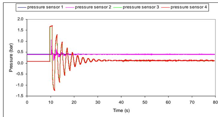
Figure 6. Numerical results in a pipeline with a leak in solenoid valve 1.
