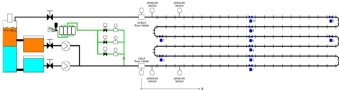
Figure 2. Schematic representation of the pilot pipeline at the Industrial Multiphase Flow laboratory.
