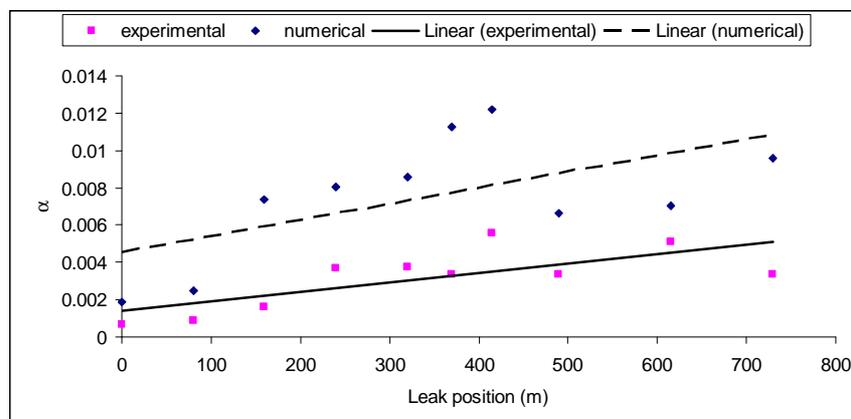
Figure 9. Detection obtained in experimental and numerical results ( $\alpha$  at  $x=0$  represents no leak).
