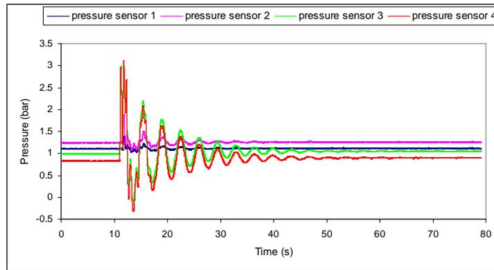
Figure 5. Experimental results in a pipeline with a leak in solenoid valve 1.
