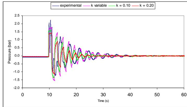
Figure 8. Comparison of numerical and experimental results in the pipeline with a leak in solenoid valve 1.
