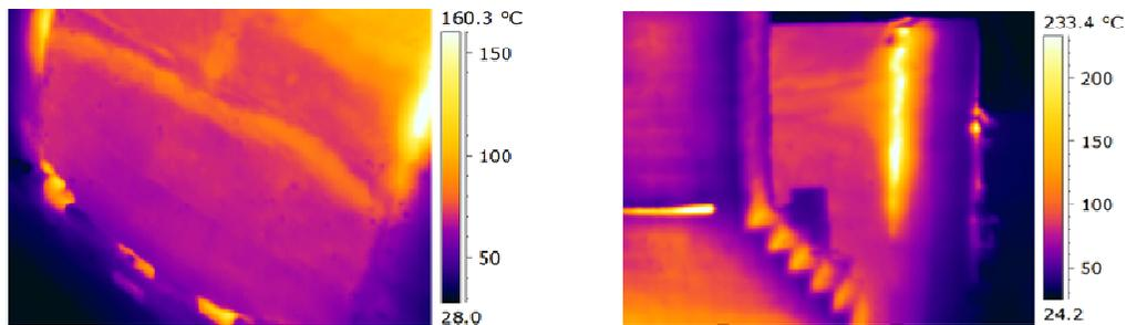
Figure 6. Critical points on Oven 1
