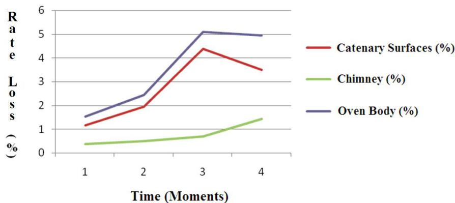
Figure 11. Rate of heat loss in relation to the increase of the oven 2 internal temperature
