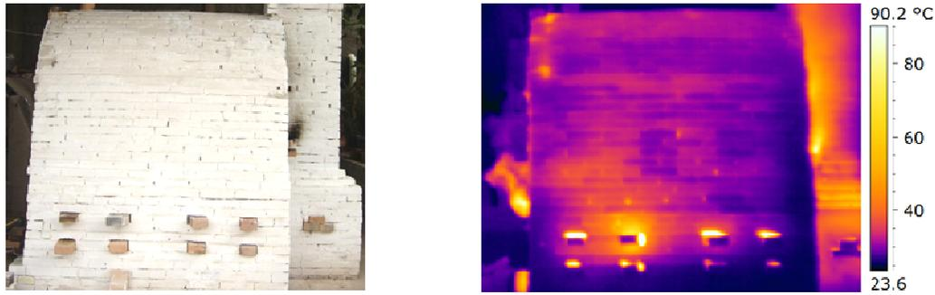
Figure 7. Critical points in the surface of Oven 2
