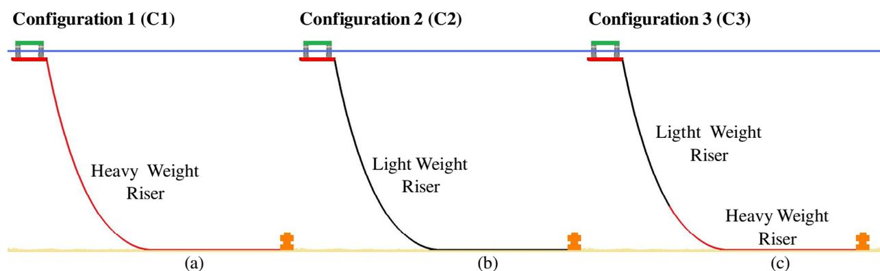
Figure 2. Scheme of catenary shaped riser system with different materials
