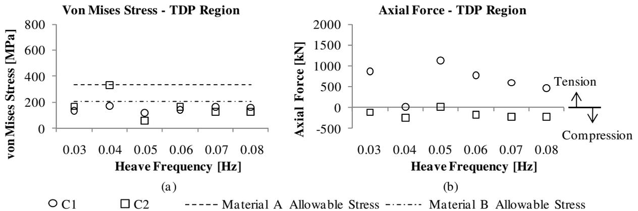
Figure 5. Effects of platform heave motion frequency on (a) riser's stress and (b) axial force at the TDP region
