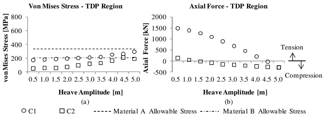
Figure 4. Effects of platform heave motion amplitude on (a) riser's stress and (b) axial force at the TDP region
