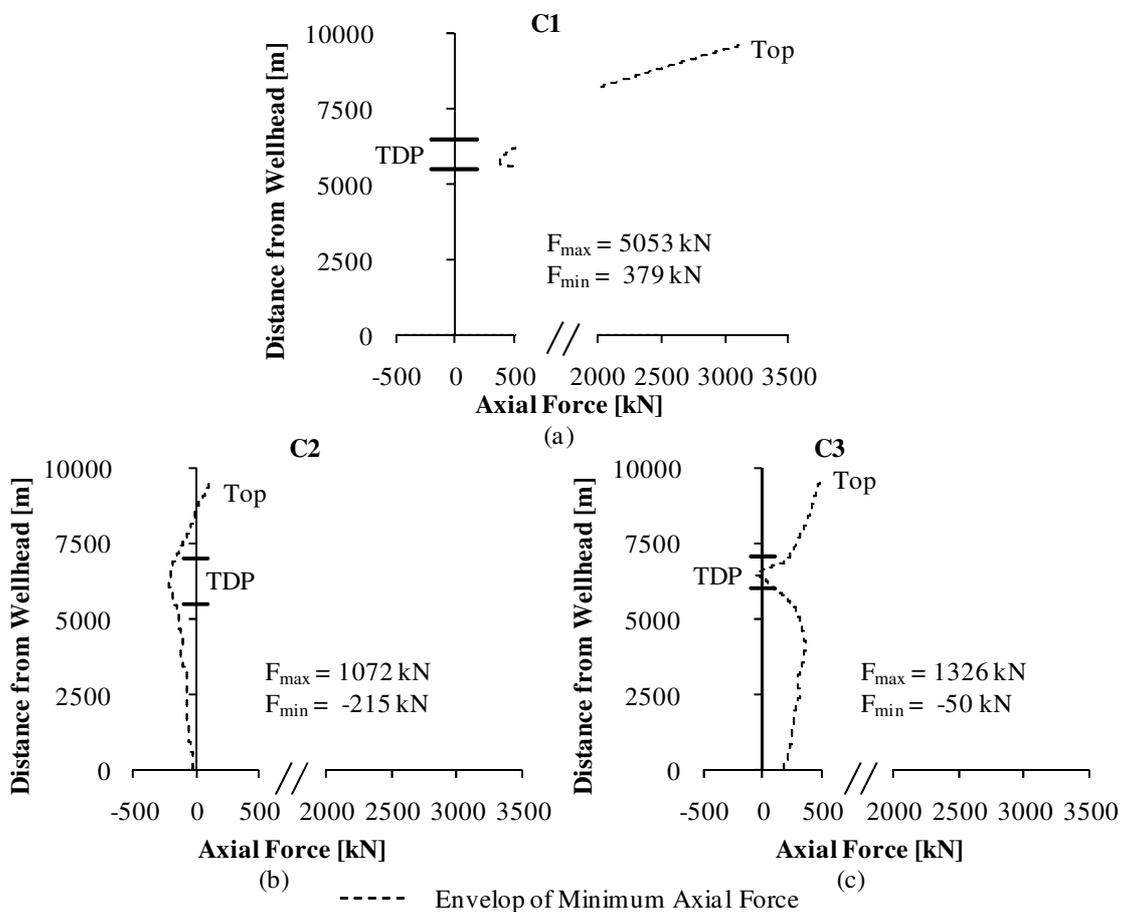
Figure 6. Envelop of minimum axial force of different configurations
