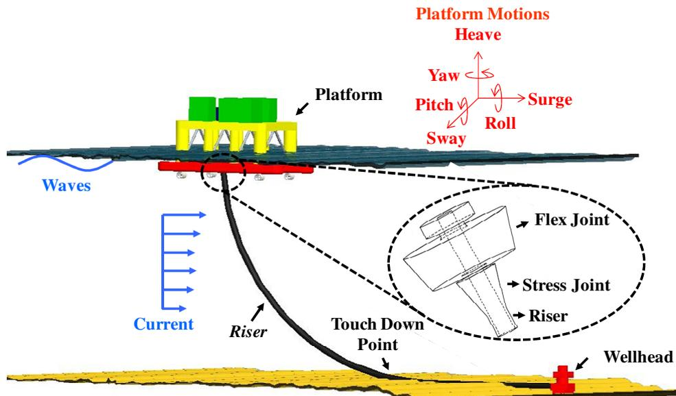
Figure 1. Schematic view of the riser system in the study
