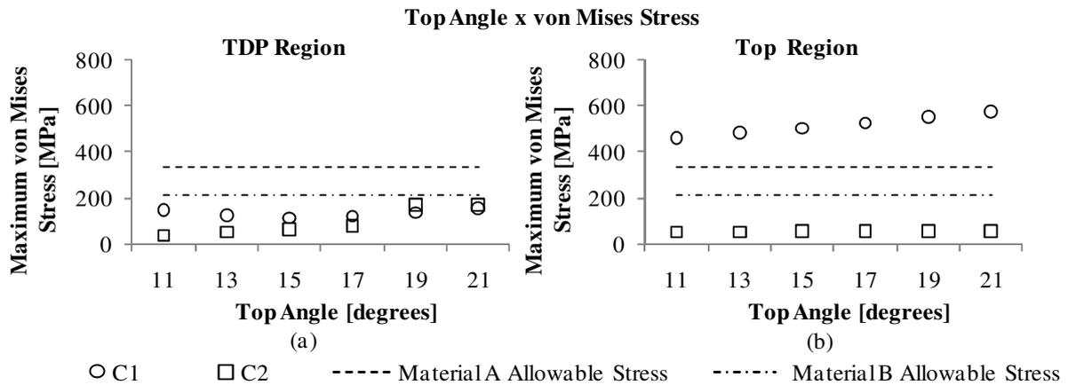
Figure 3. (a) Riser Top Angle vs. von Mises Stress for the TDP Region, and (b) Riser Top Angle vs. von Mises Stress for the Riser Top Region
