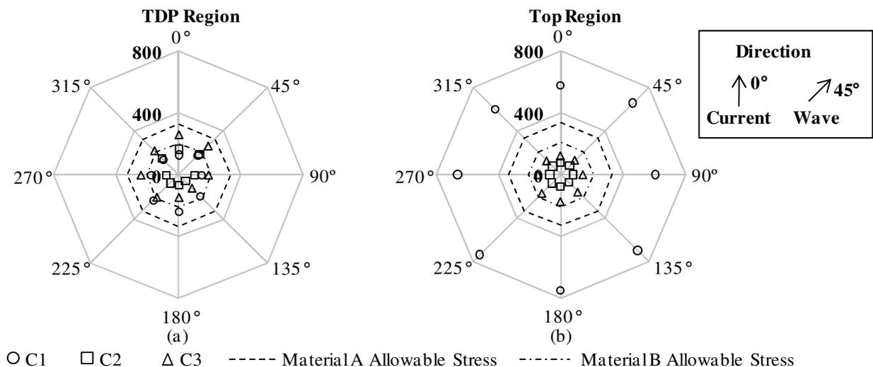
Figure 8. Maximum von Mises stress for different heading direction
