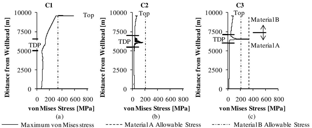
Figure 7. Maximum von Mises stress of different configurations
