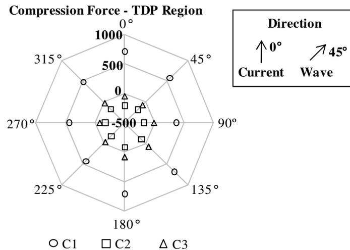
Figure 9. Compression force for different heading direction
