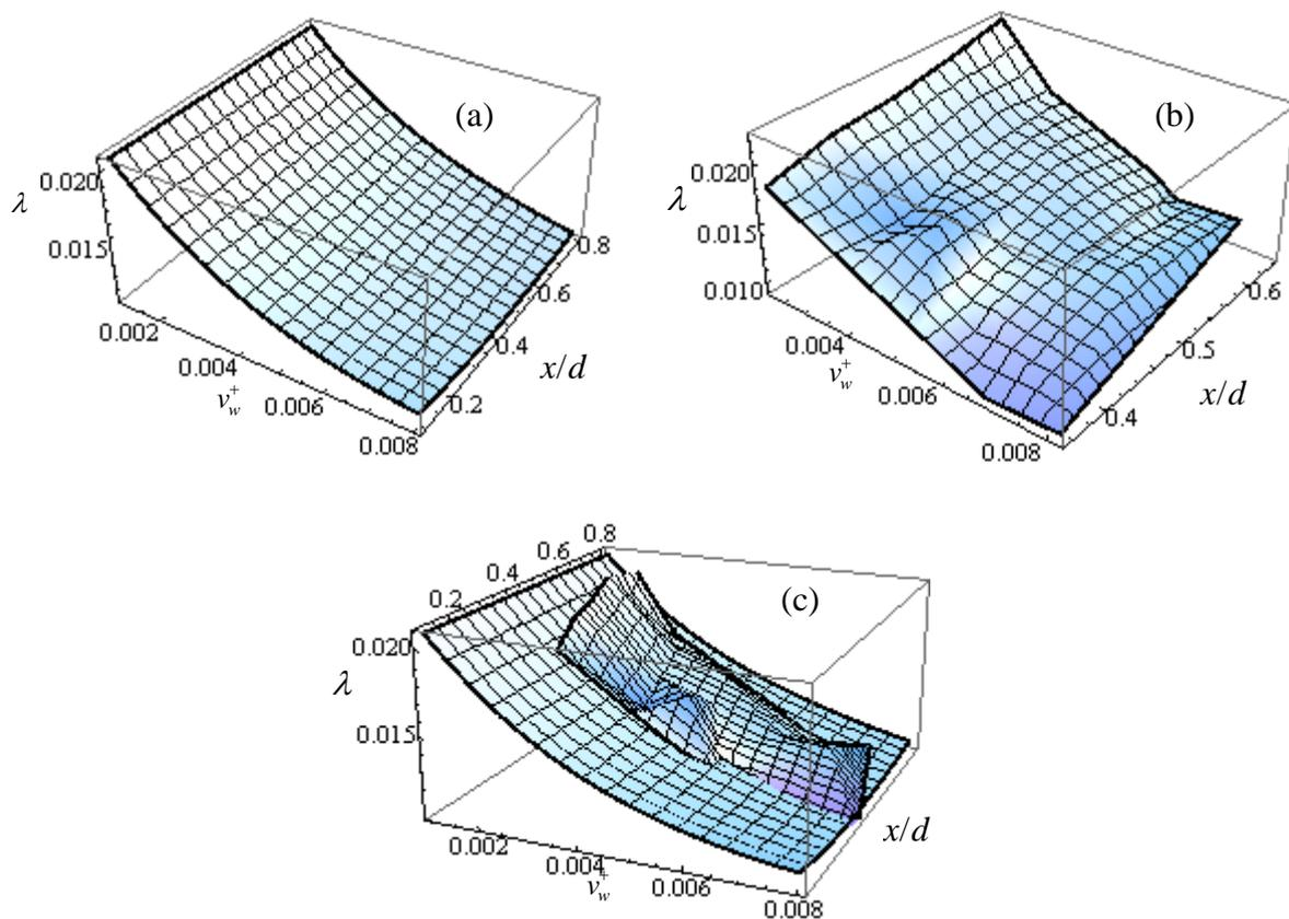
Figure 1. Friction coefficient for transpired flow over rough walls. a: present theory, b: data of Olson and Eckert (1966), c: comparison of (a) and (b).
