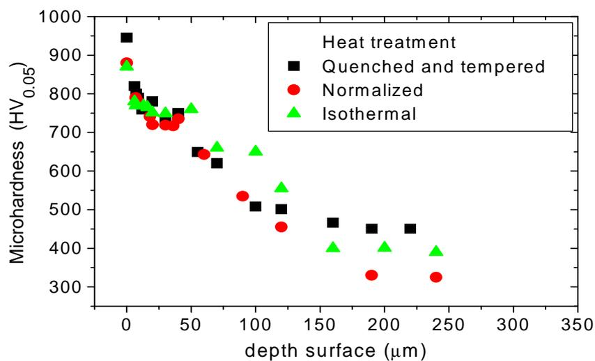
**Figure 5** AISI 4340 steel microhardness profile: Quenched/Tempered, Isothermal transformation and Normalized.
