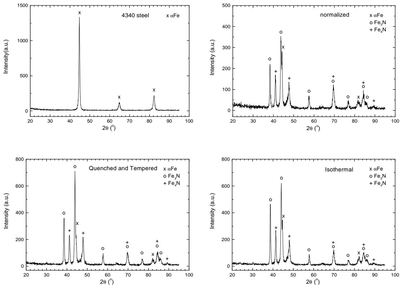
**Figure 6:** AISI 4340 XR Diffractometer: Nitrocarburizing on three heat treatment conditions.
