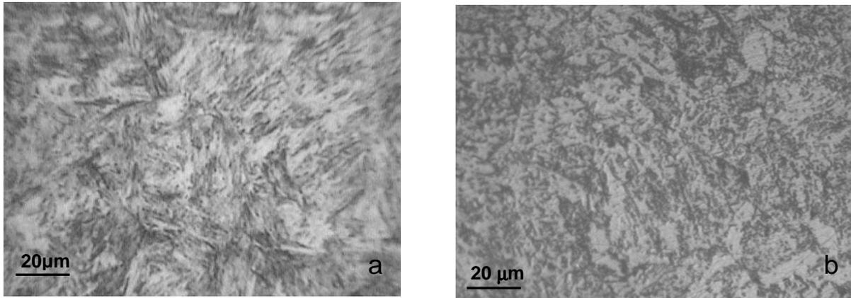
**Figure 2:** AISI 4340 steel microstructure: (a) Quenched and Tempered; (b) Quenched/Tempered and Nitrocarburized.
