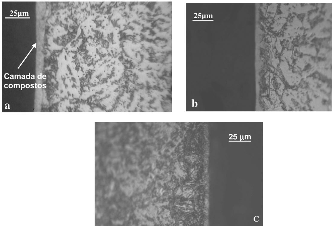
**Figure 4:** AISI 4340 steel microstructure: (a) Normalized and Nitrocarburized; (b) Quenched and Tempered; (c) Isothermal Transformation.
