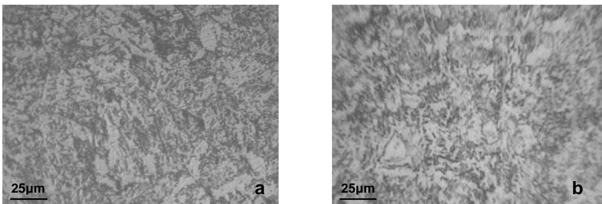
**Figure 1:** AISI 4340 steel microstructure: (a) Normalized; (b) Normalized and Nitrocarburized.
