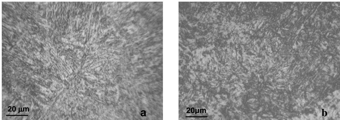
**Figure 3:** AISI 4340 steel microstructure: (a) Isothermal transformation; (b) Isothermal transformation and Nitrocarburizing.
