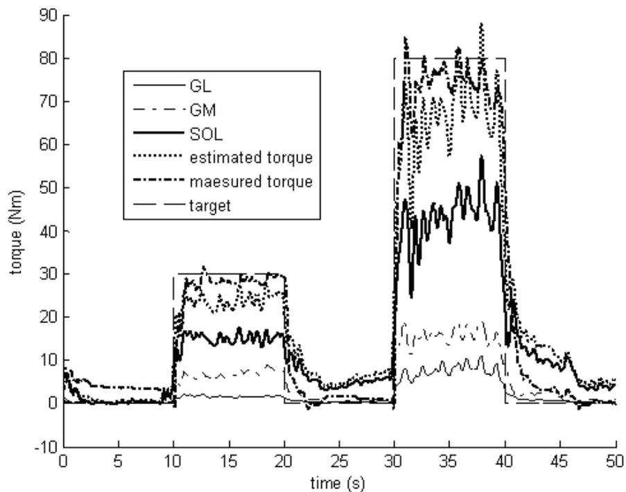
Figure 2. Ankle torque estimated for each individual muscle, overall sum of such torques and the torque measured by Cybex<sup>TM</sup>, for the same subject. The dashed line represents the target shown on-line to the subject with the torque demands, superimposed with the measured torque from the dynamometer.
