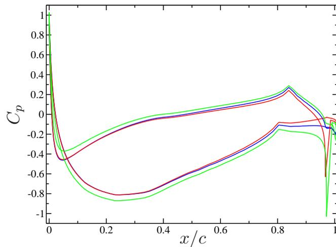
Figure 8. Pressure coefficient at  $\alpha = 0^\circ$ . (SS – PS – no act –)
