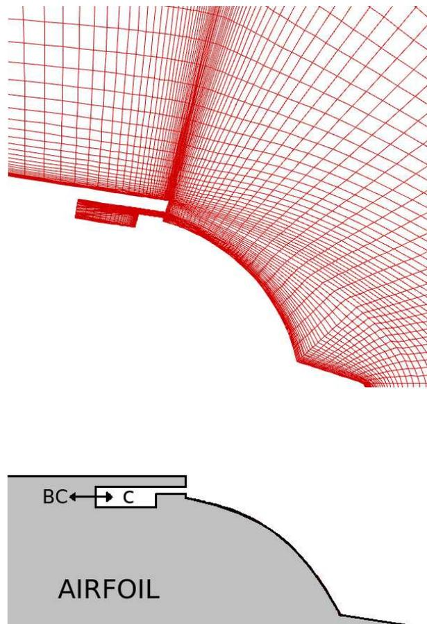
Figure 2. Geometry of the synthetic jet cavity (c) with mesh and detail of the boundary condition (BC)
