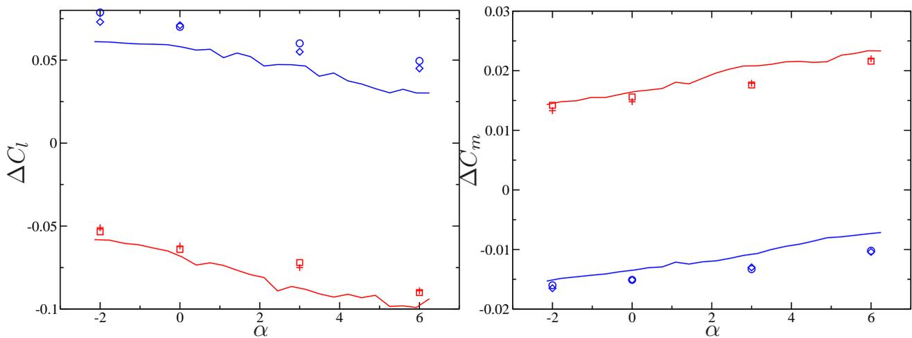
Figure 9. Actuator effectiveness. (SS exp — PS exp — SS detailed model ◊ PS detailed model + SS RSSJ model ◊ PS RSSJ model ◻)
