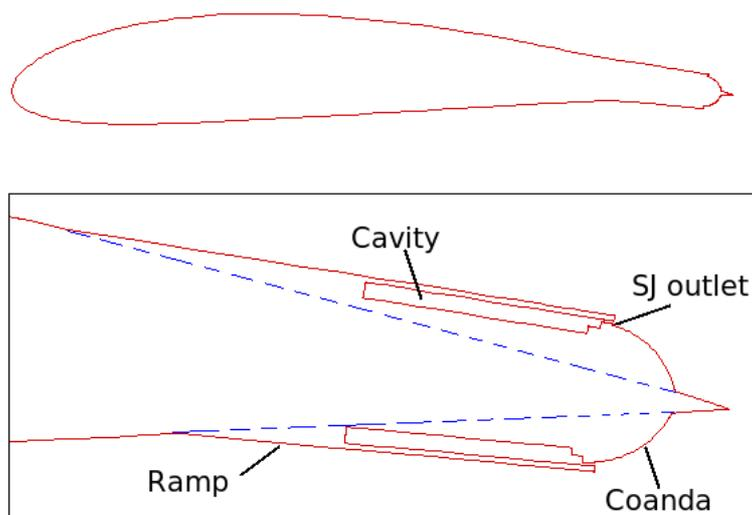
Figure 1. Modified NACA 4415 profile with trailing edge detail.
