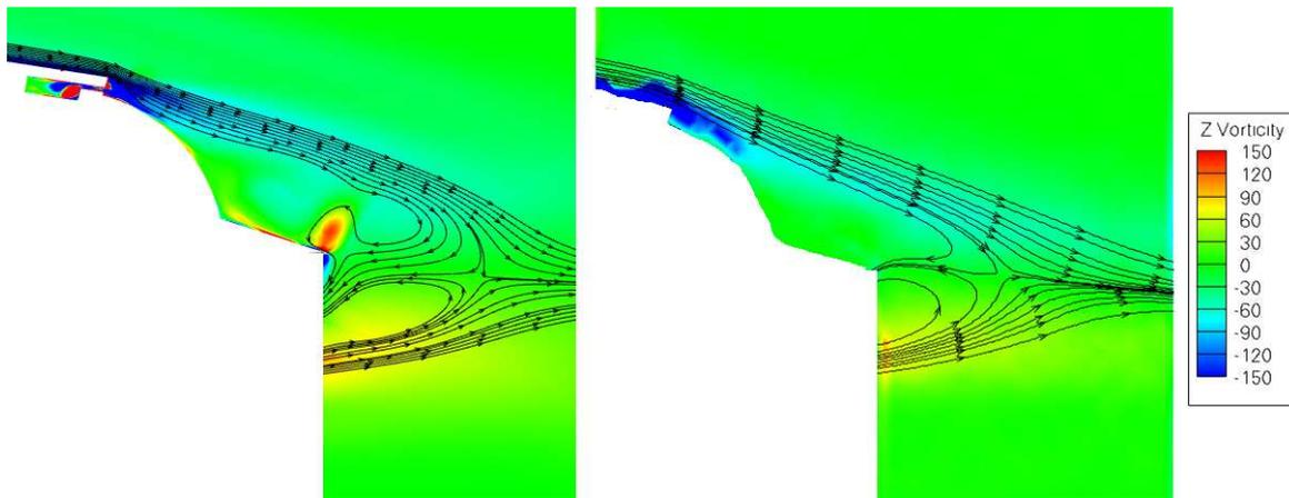
Figure 4. Time averaged vorticity field including streamlines for the suction side actuator. Computational (left) and experimental PIV (right)
