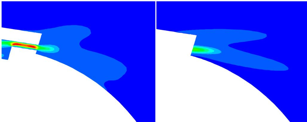
Figure 3. Averaged difference of the  $\overline{u'u'}$  Reynolds stress component at  $\alpha = 0^\circ$ ,  $Re = 9 \times 10^5$ . Detailed model(left) and RSSJ model (right)
