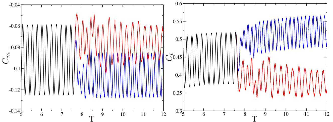
Figure 7. Evolution of aerodynamic properties - RSSJ model. (No act – SS – PS –)
