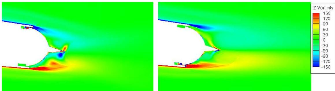
Figure 5. Computational time averaged vorticity field in the near wake ( $\alpha = 0^\circ$ ). SS actuation (left) and PS actuation (right)
