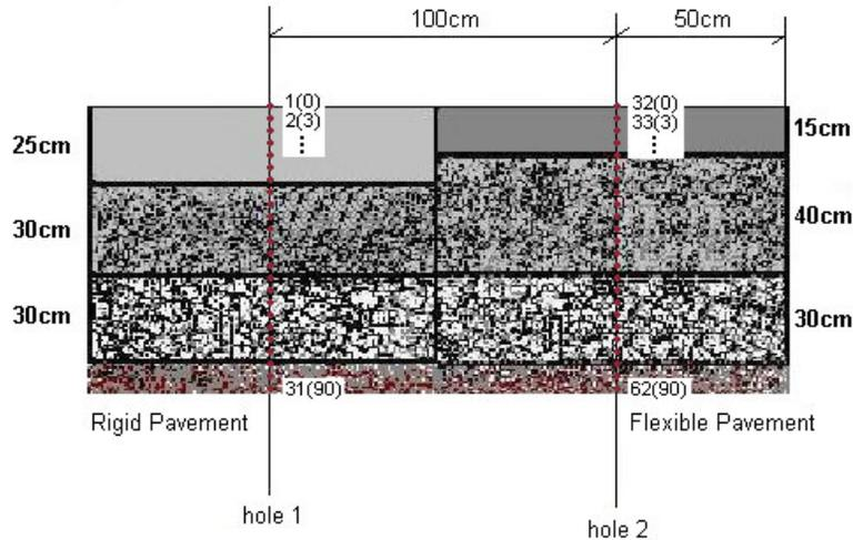
Figure 1. Pavement scheme (the first no. indicates the channel and the second the depth)
