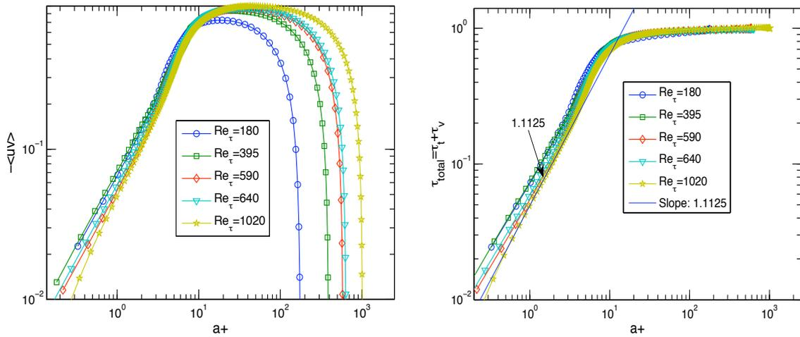
Figure 4. The profile of turbulent Reynolds stress  $-\overline{u'v'}$  (a) and total stress  $\tau_{total}$  (b) vs. shear rate  $a^+$  in log-log plot.
