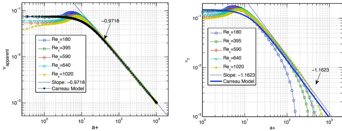
Figure 2. The profile of apparent viscosity  $\nu_{apparent}$  (a) and turbulent viscosity  $\nu_T$  (b) vs. shear rate  $a^+$  in log-log plot and Carreau model fitting.
