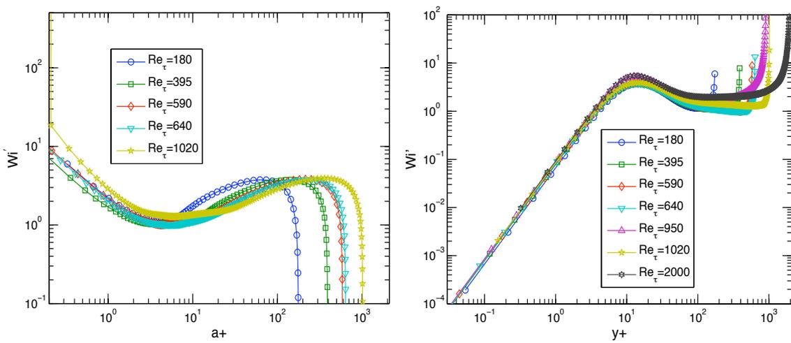
Figure 3. The distributions of Weissenberg number  $Wi' = \lambda' a^+$  vs.  $a^+$  (a) and vs.  $y^+$  (b) in log-log plot.
