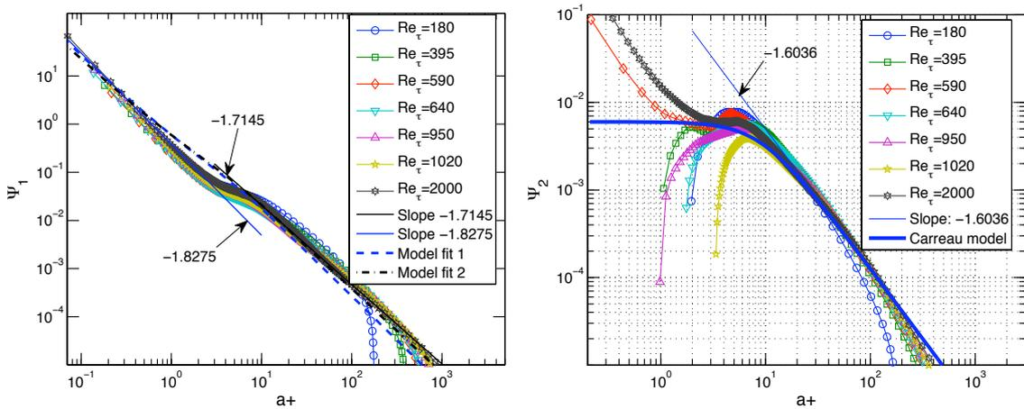
Figure 5. The Carreau model fitting of viscometric functions  $\Psi_1$  (a) and  $\Psi_2$  (b).
