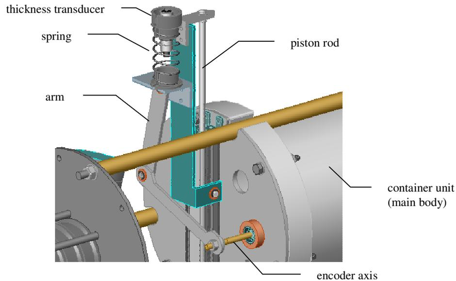
Figure 7. Details of the Tinta-P container unit and onboard components.
