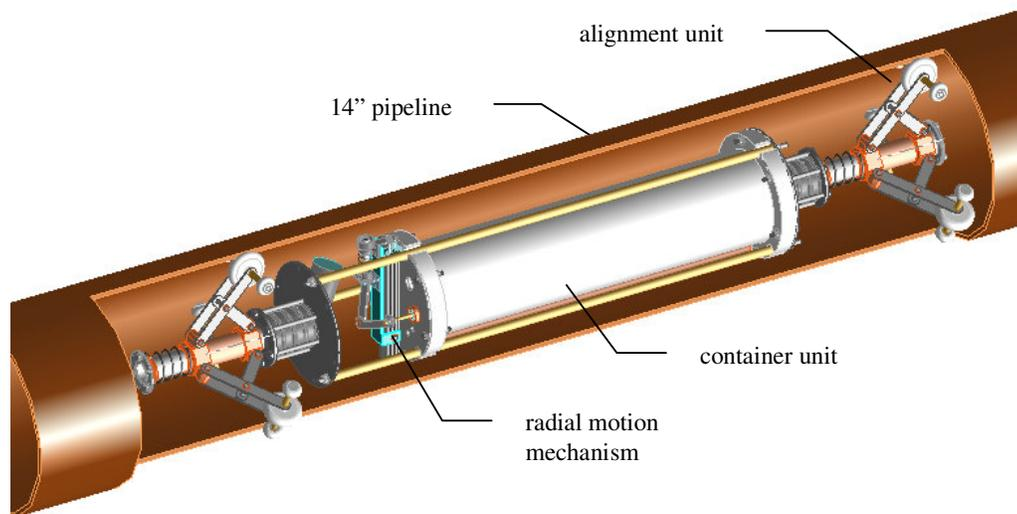
Figure 4. Tinta-P prototype and pipeline CAD model.
