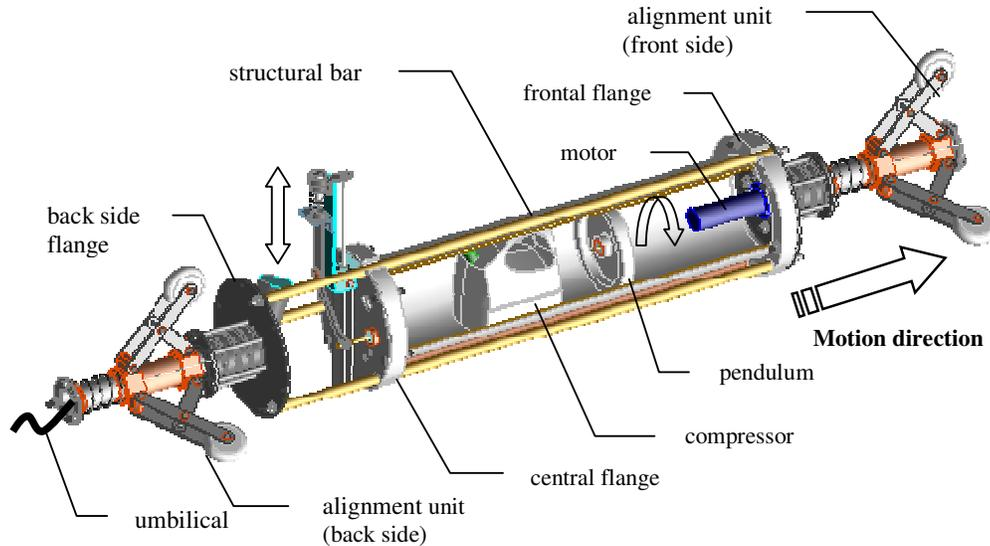
Figure 5. Details of Tinta-P components.
