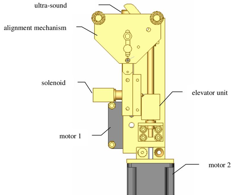
Figure 2. First prototype: mechanism main parts.
