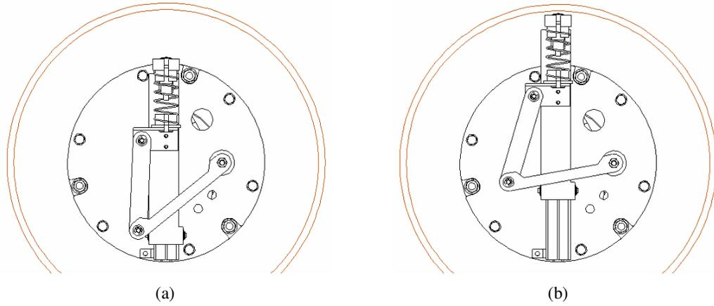
Figure 8. Arm measuring system. (a) retracted configuration. (b) extended configuration.
