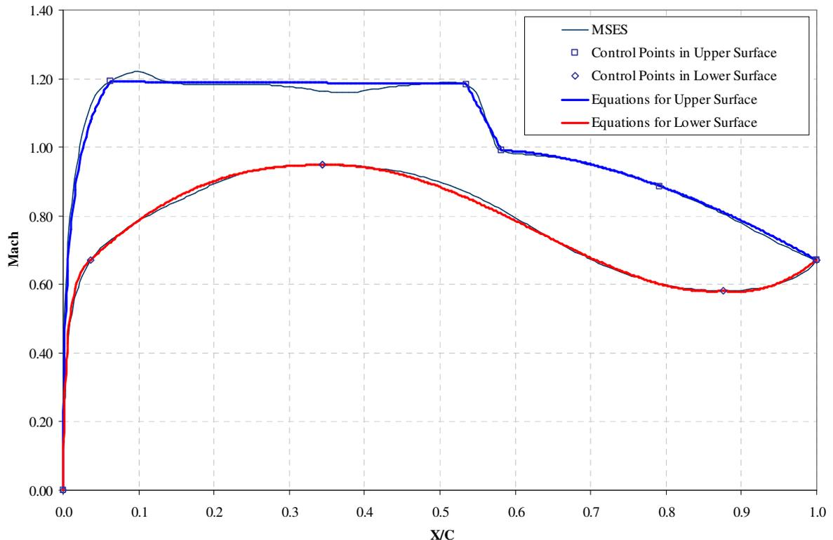
Figure 4. MSES results compared with Kim and Rho (1997) equations in an airfoil with  $(t/c)_{max} = 13\%$ , at  $CL$  0.60 and Mach 0.75.
