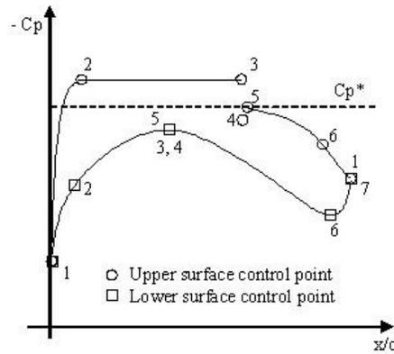
Figure 1. Control point from supercritical airfoil pressure distribution.
