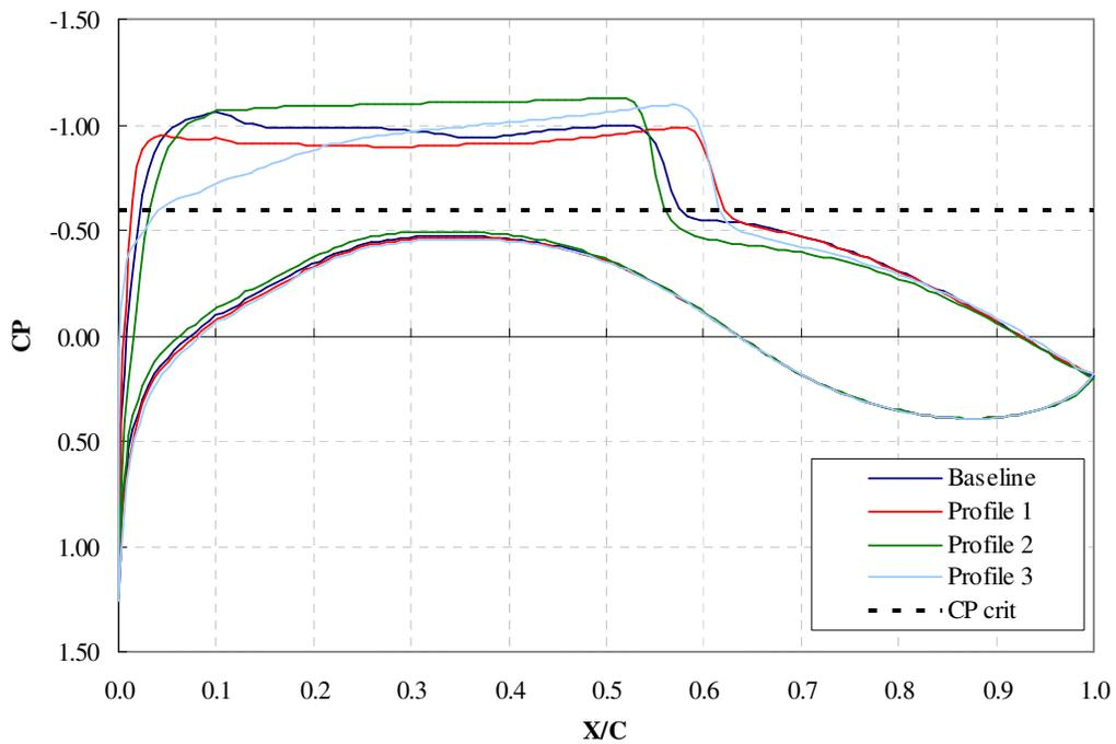
Figure 8.  $C_p$  versus  $X/C$  at Mach 0.75 and  $CL$  0.60 for the four airfoils
