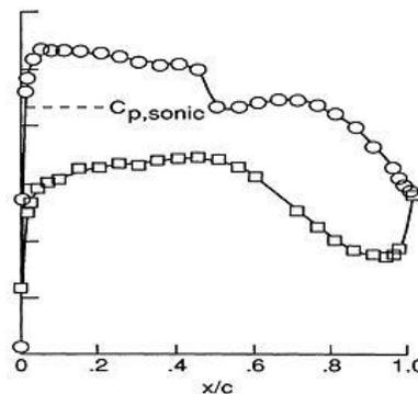
Figure 6. Pressure distribution at design condition for supercritical airfoil.
