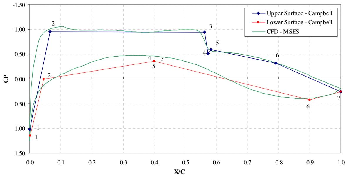
Figure 2. Campbell (1992) methodology with modified control point 2 and 6 from lower surface compared with MSES results. Airfoil with  $(t/c)_{\max} = 13\%$ , at Mach = 0.75 and  $CL = 0.60$
