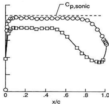
Figure 5. Sonic-plateau pressure distribution at off-design condition with Mach and  $CL$  lower than design condition for supercritical airfoils.
