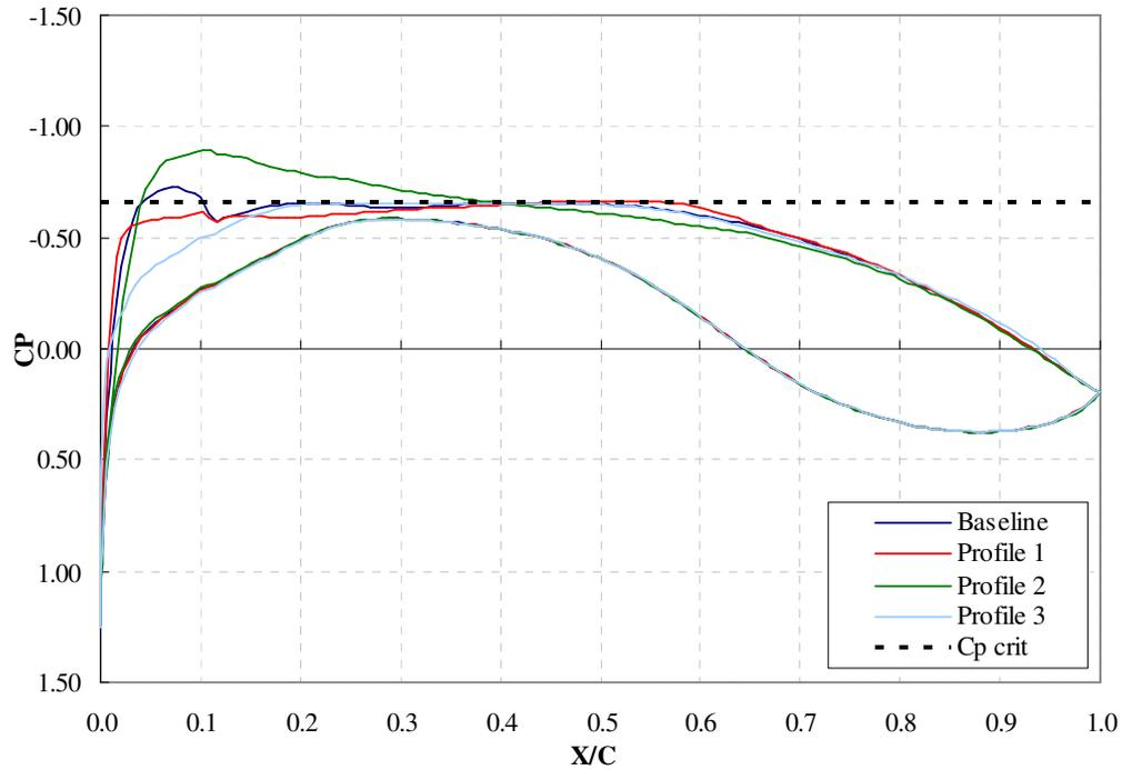
Figure 7.  $C_p$  versus  $X/C$  at Mach 0.73 for baseline airfoil and modified ones.
