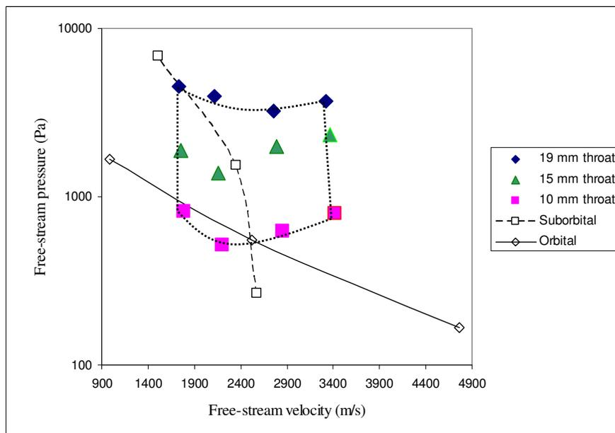
Figure 10. The SARA trajectories and the tunnel T2 operational map (Pressure x Velocity)
