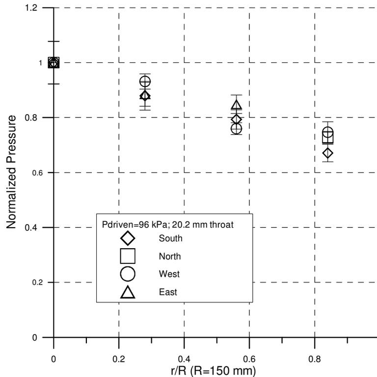
Figure 5. Normalized pressure distribution as a function of transducer position ( $P_{driven}=96$  kPa; helium in driver)
