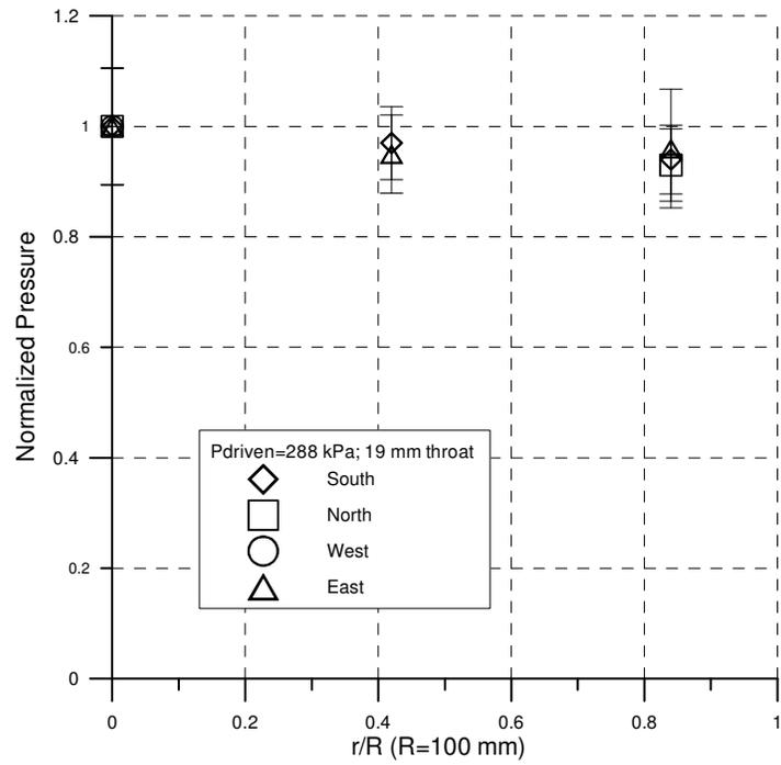
Figure 3. Normalized pressure distribution as a function of transducer position ( $P_{driven}=288$  kPa; helium in driver)
