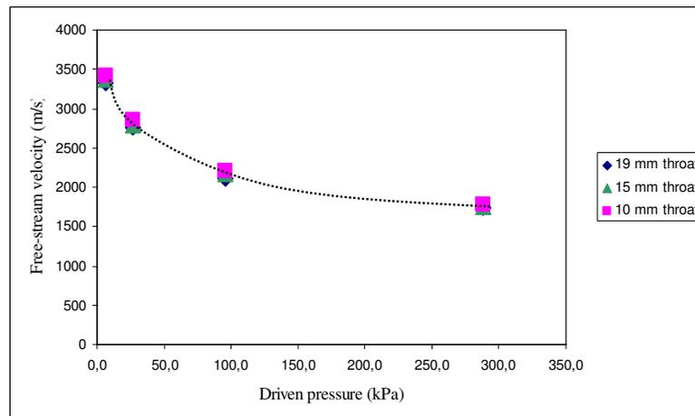
Figure 8. Free-stream velocities as a function of the shock tunnel T2 driven pressures
