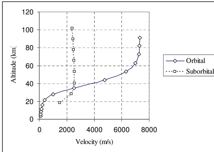
Figure 9. Segments of the orbital and suborbital descending trajectories of SARA vehicle
