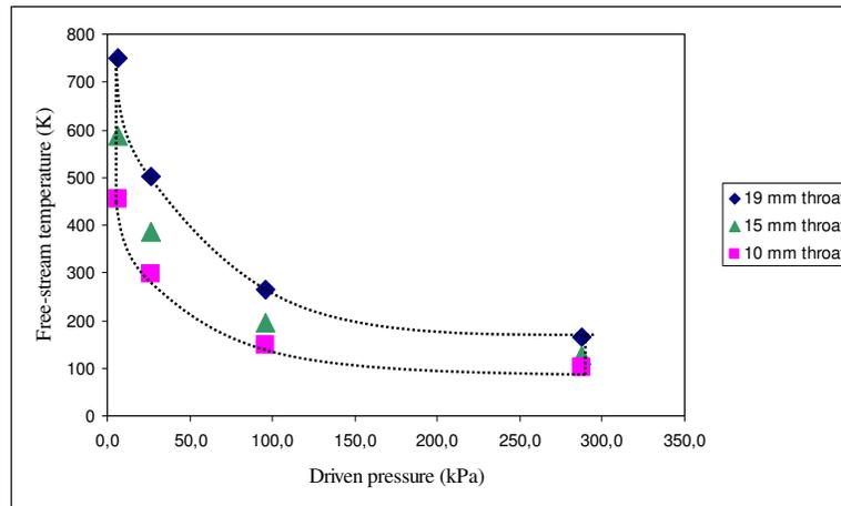
Figure 7. Free-stream temperatures as a function of the shock tunnel T2 driven pressures
