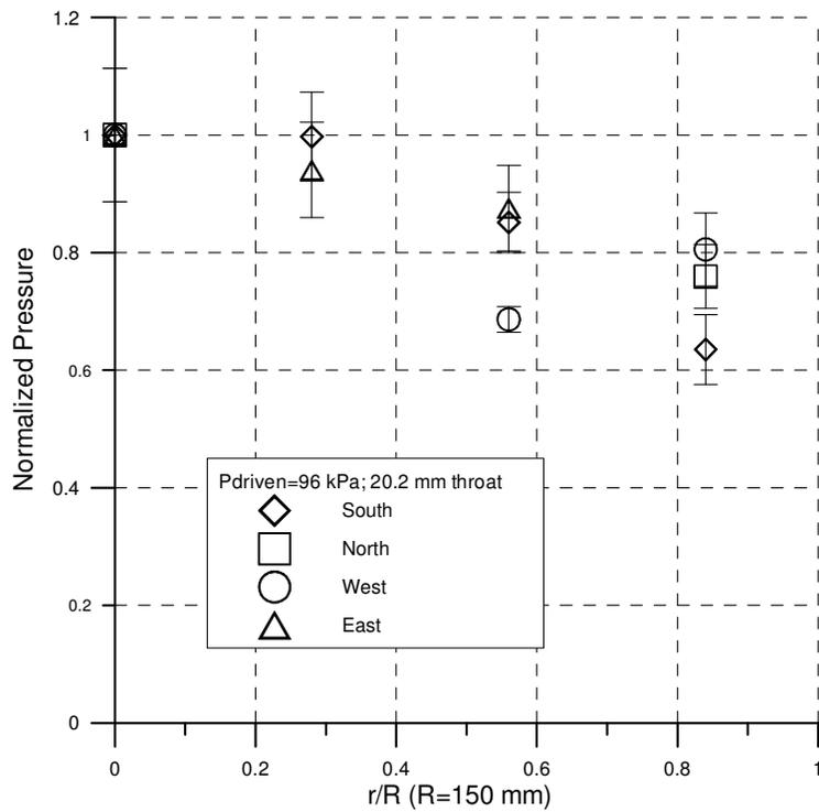
Figure 4. Normalized pressure distribution as a function of transducer position ( $P_{driven}=96$  kPa; air in driver)
