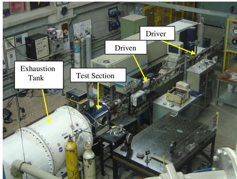
Figure 1. Panoramic view of the T2 hypersonic tunnel
