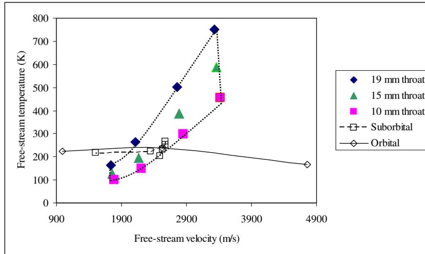
Figure 11. The SARA trajectories and the tunnel T2 operational map (Temperature x Velocity)
