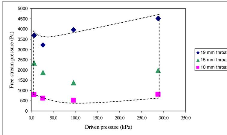
Figure 6. Free-stream pressures as a function of the shock tunnel T2 driven pressures
