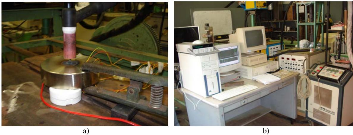
Figure 2. Experimental apparatus: a) Thermocouples and welding torch positioned in the sample; b) Data acquisition system.
