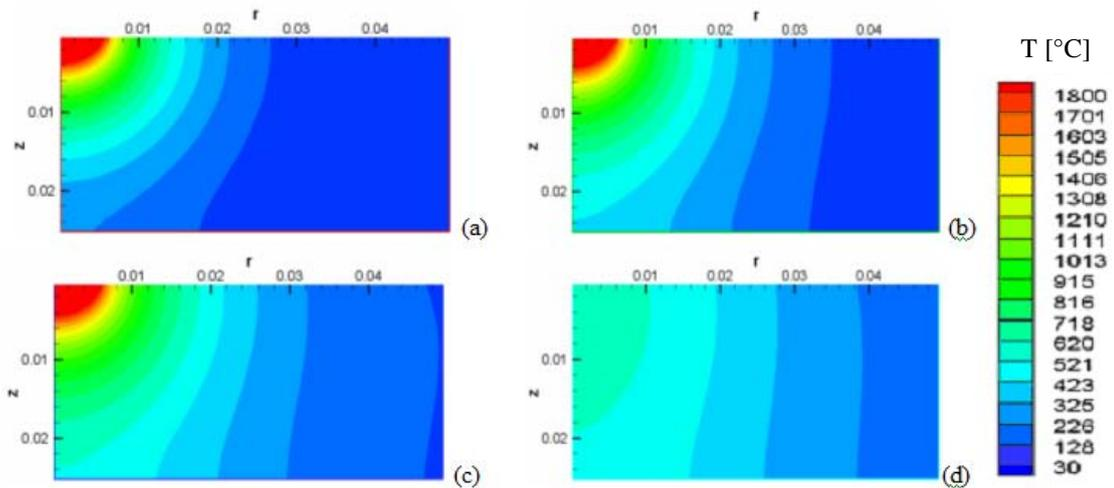
Figure 5. Thermal fields at: a) 37.5 [s]; b) 75.0 [s]; c) 112.5 [s] e d) 150.0 [s].
