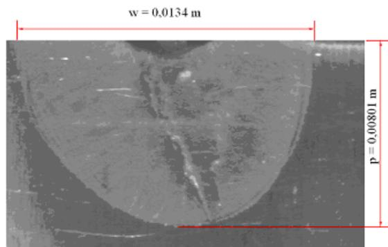
Figure 7. Width and depth of the weld bead for test C1.
