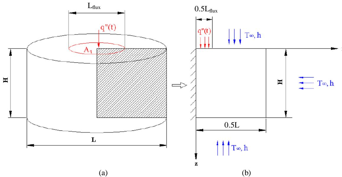
Figure 1. a) The physical model in cylindrical coordinates. b) The simplified physical model.
