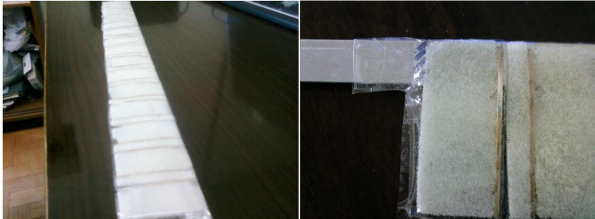
Figure 12: Wing model made by expanded polyurethane
