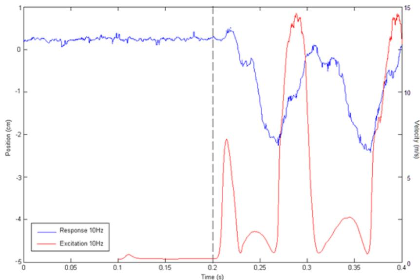
Figure 12. Excitation and response at 10Hz
