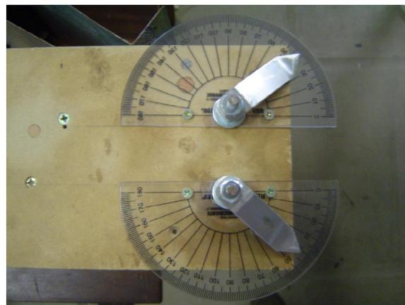
Figure 2. Protractors used to measure the diffuser's angle
