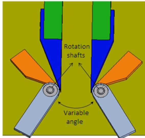
Figure 1. Variable angle diffuser (upper view without the upper wall)
