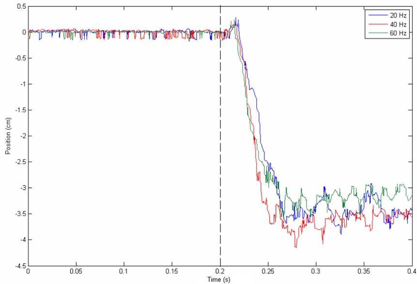
Figure 11. Response to step signals (20Hz, 40Hz, 60Hz)
