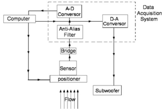
Figure 3. Data Acquisition System Setup
