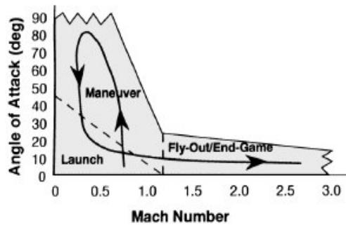
Figure 3. Agile missile flight envelope (Wise and Roy, 1998)
