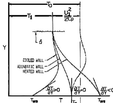
Figure 7. Boundary-layer temperature distribution.
