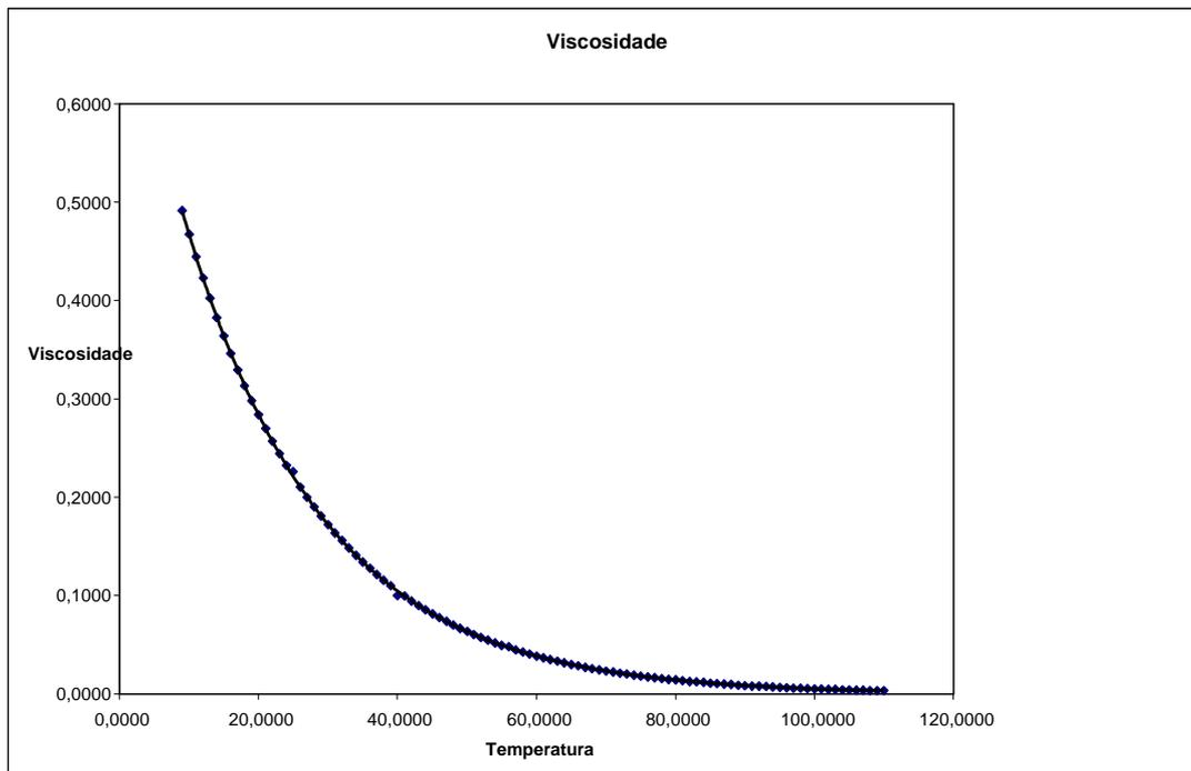
Figure 3. Char Viscosity x Temperature
